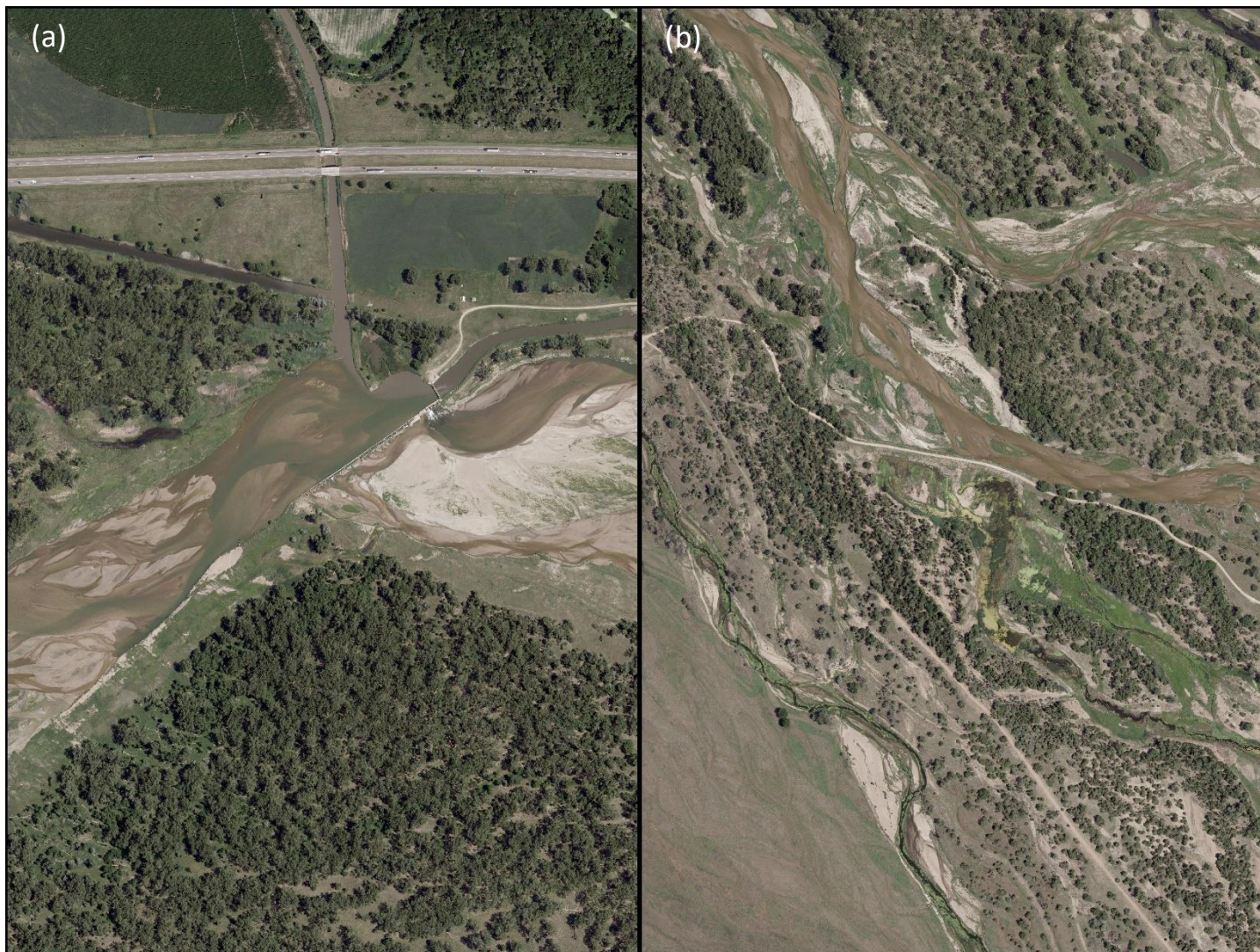
Figure 3. Kearney Diversion Dam (a) and the levee that disconnects the south channel, also called the “Sand Dam” (b). A portion of the breakthrough channel that is blocked with a berm at the upstream end is also shown in (b).
