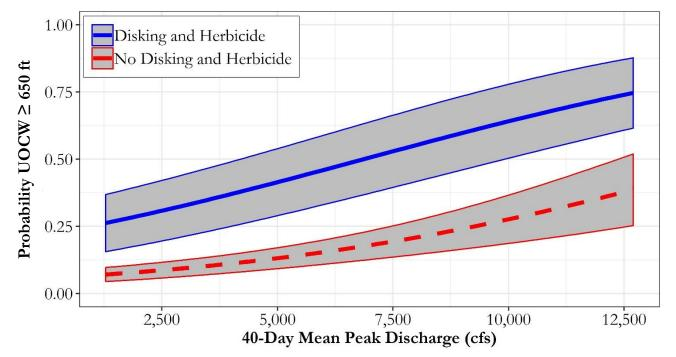
**Figure 4**. Predicted probability of a transect measuring  $\geq$ 650 ft in unobstructed channel width (suitable for whooping cranes) in relation to 40-day peak discharge at transects with (blue solid line) or without (red dashed line) mechanical management actions in the AHR from 2007 to 2018. Shaded regions indicate 95% confidence intervals. Disking and herbicide application provide a significantly greater probability of having channels with more than 650 ft unobstructed channel widths.
