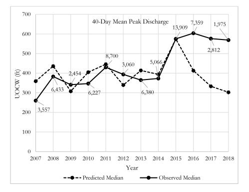
**Figure 3.** Observed versus predicted median unobstructed channels widths (UOCW) in the AHR during the period of 2007-2018. The UOCW model provides good predictive capacity for evaluating the efficacy of SDHF releases prior to 2016<sup>5</sup>. Poor predictive performance in 2016-2018 indicates there is an additional driver that is maintaining UOCW during that period despite low 40-day mean peak discharge magnitudes.
