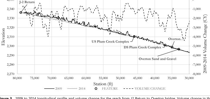
**Figure 3.** 2009 to 2014 longitudinal profile and volume change for the reach from J2 Return to Overton bridge. Volume change in the reach immediately downstream of the J-2 Return is caused by channel incision. Futher downstream, volume change is due primarily to channel widening.
