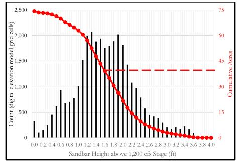
**Figure 2.** Distribution of emergent sandbar area produced during the 2015 peak flow event in the portion of the AHR downstream of Kearney. The 15,000 cfs event produced 43 cumulative acres (line) of sandbar habitat exceeding the minimum height suitability criterion of 1.5 ft above 1,200 cfs stage. Median height of bars was 1.6 ft above 1,200 cfs stage.
