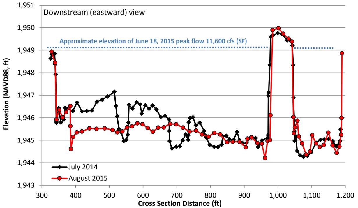
**Figure A-8. Primary Cross Section #2 – June 2014 and August 2015**
