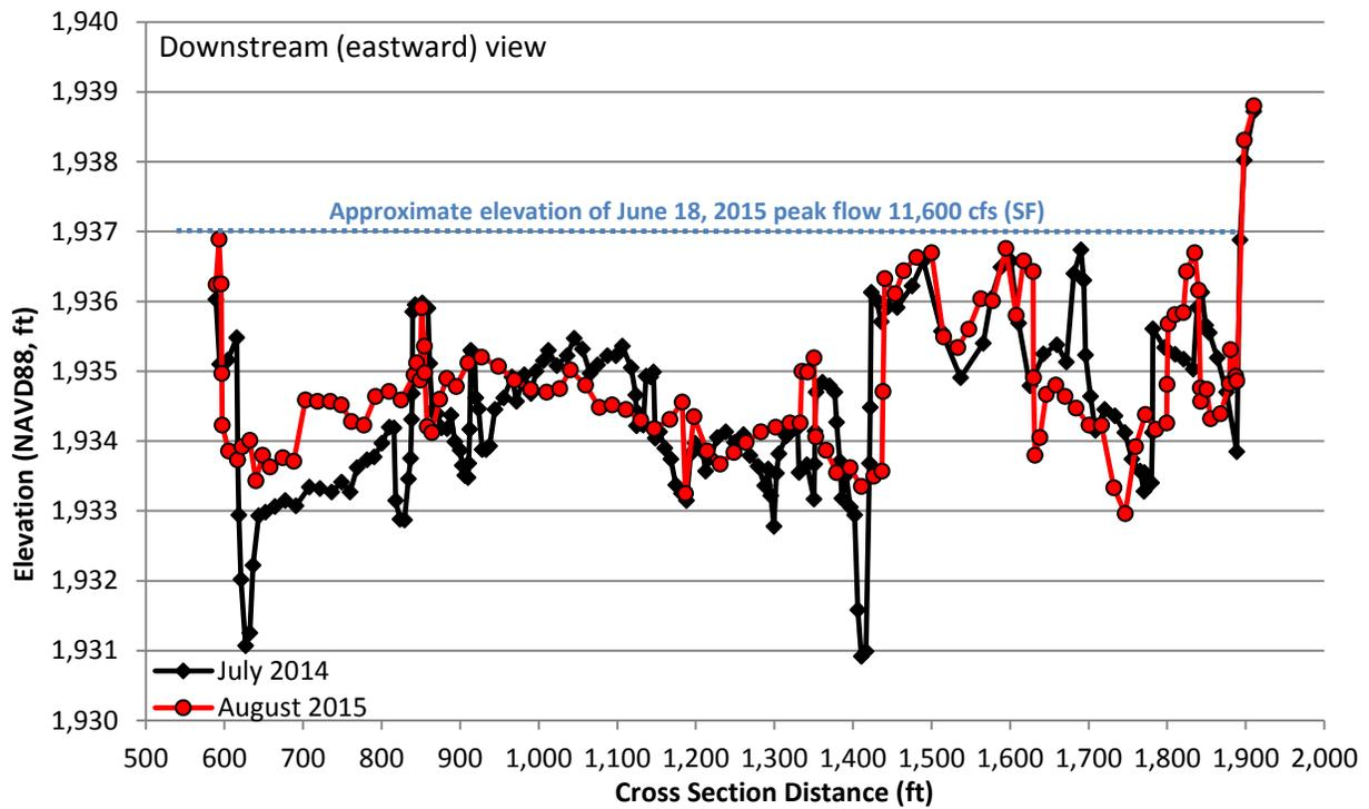
**Figure A-20. Primary Cross Section #14 – June 2014 and August 2015**
