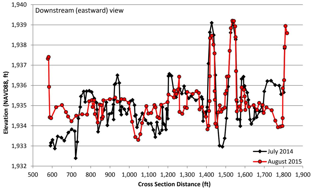
**Figure A-38. Supplemental Cross Section N – June 2014 and August 2015**
