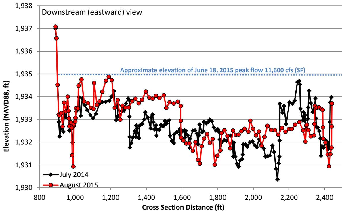
Figure A-22. Primary Cross Section #16 – June 2014 and August 2015
