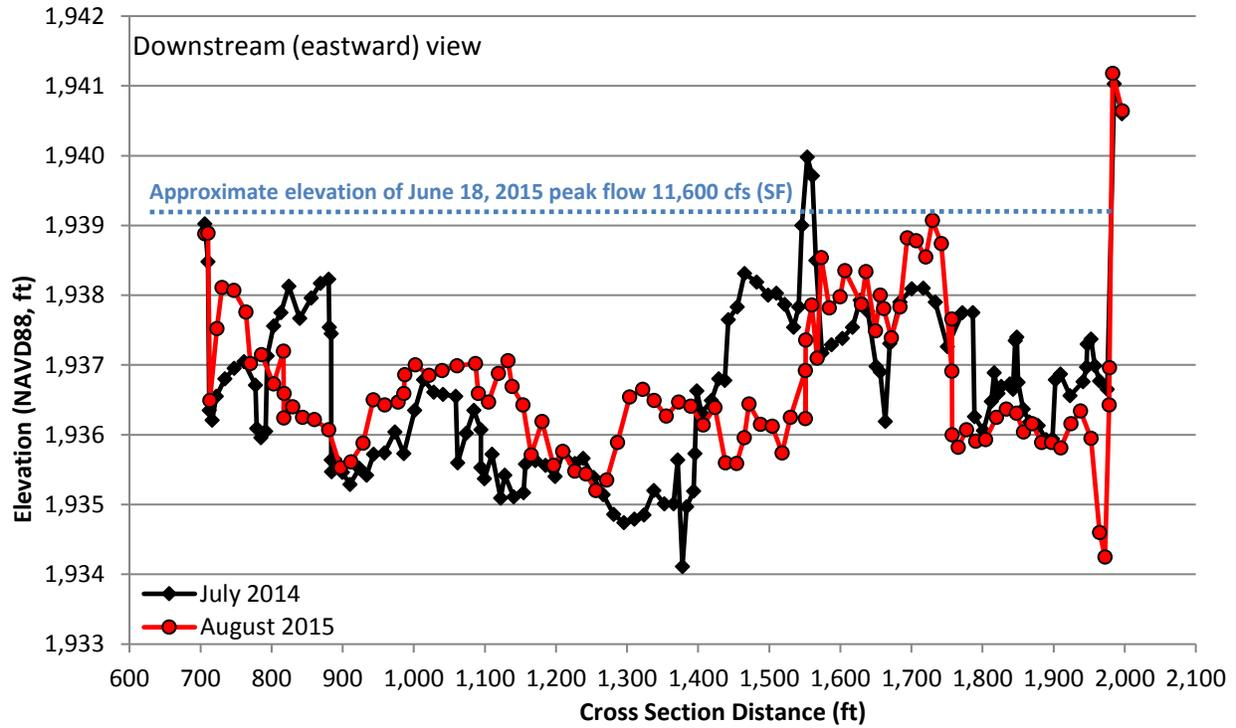
**Figure A-18. Primary Cross Section #12 – June 2014 and August 2015**
