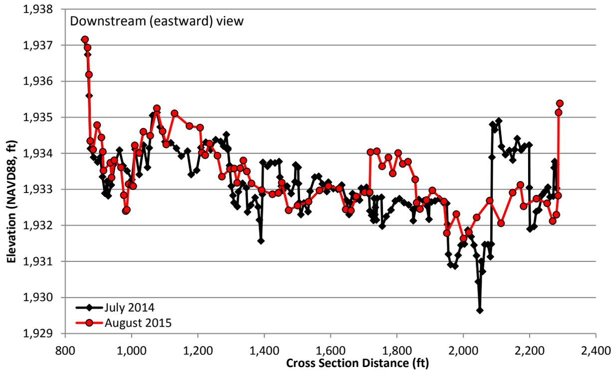
**Figure A-40. Supplemental Cross Section P – June 2014 and August 2015**
