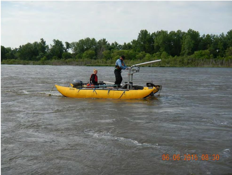
9. **Depth Integrated Sampling** – DIS samples collected from a cataraft between cross sections 2 and 3.
