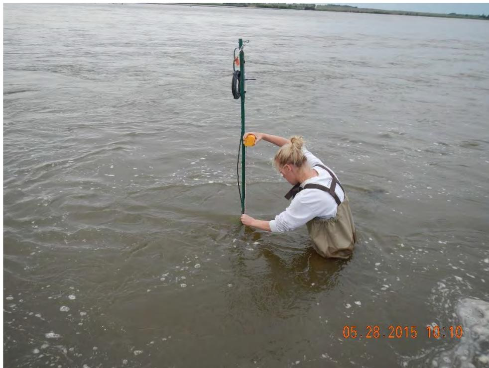
10. **River Stage** – Collection of river stage measurements at the pressure transducer located near cross section 18 during the June 2015 high flow event.
