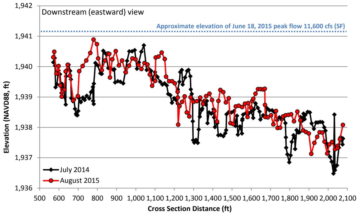
**Figure A-16. Primary Cross Section #10 – June 2014 and August 2015**
