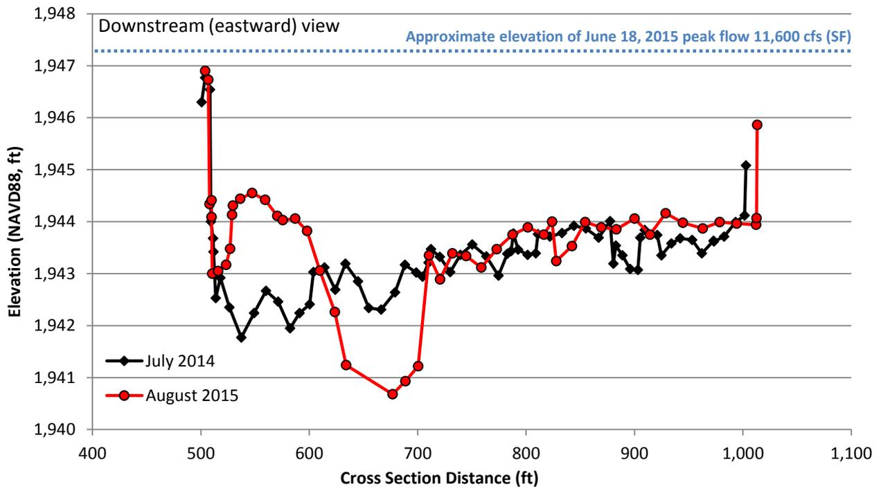
**Figure A-10. Primary Cross Section #4 – June 2014 and August 2015**
