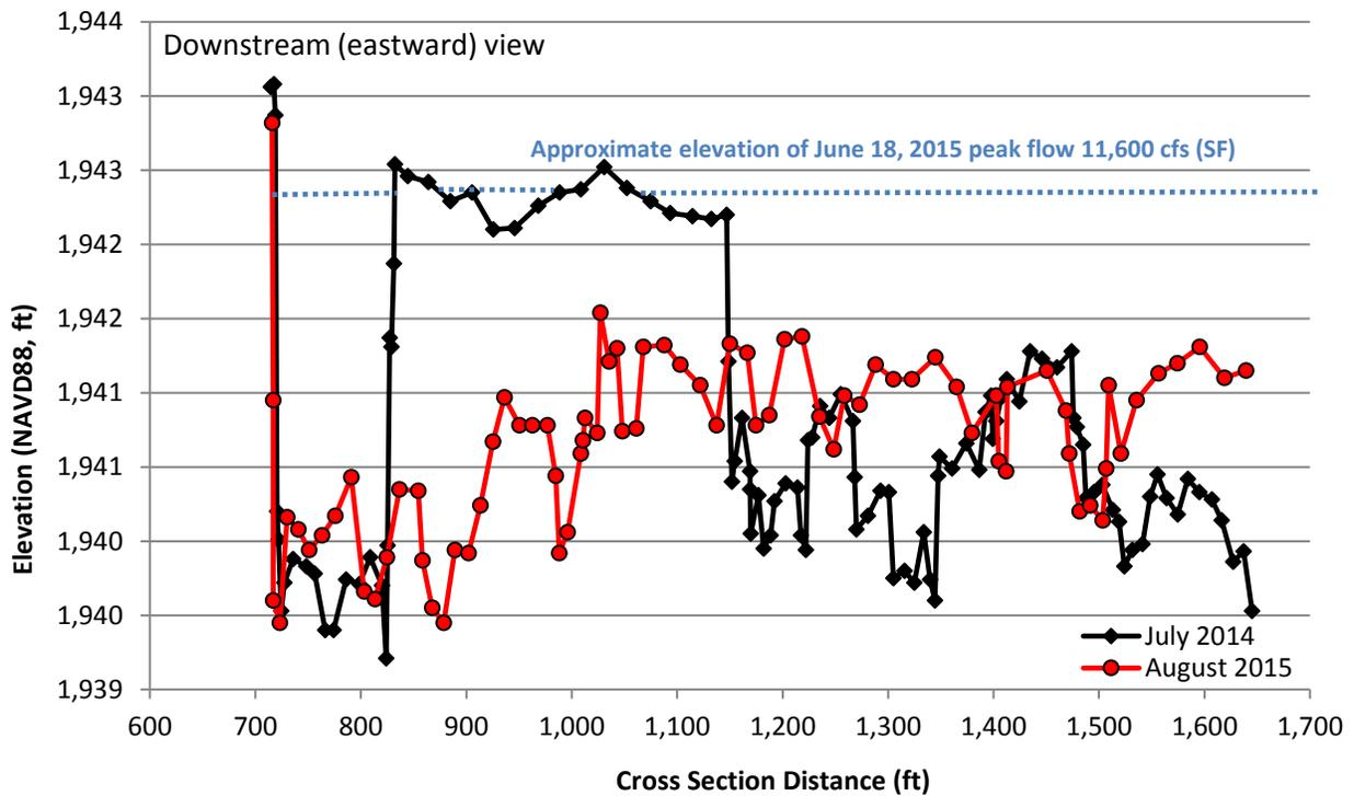
**Figure A-14. Primary Cross Section #8 – June 2014 and August 2015**
