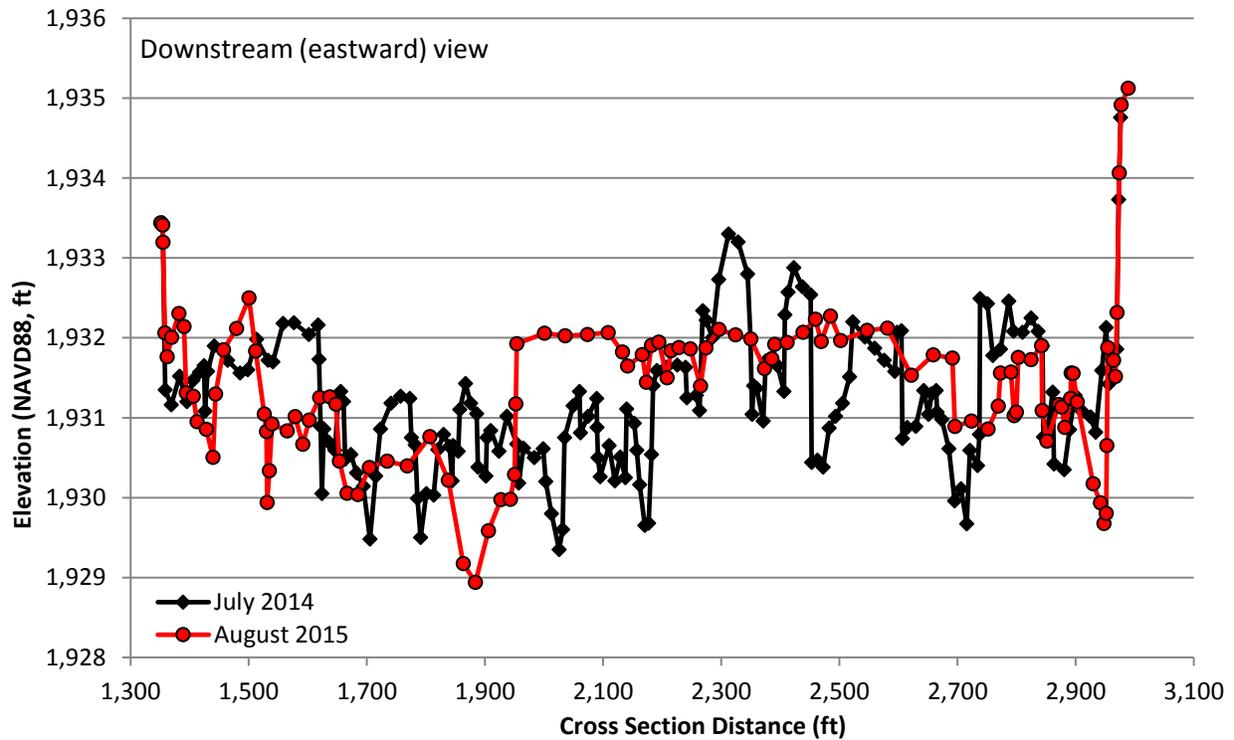
**Figure A-42. Supplemental Cross Section R – June 2014 and August 2015**
