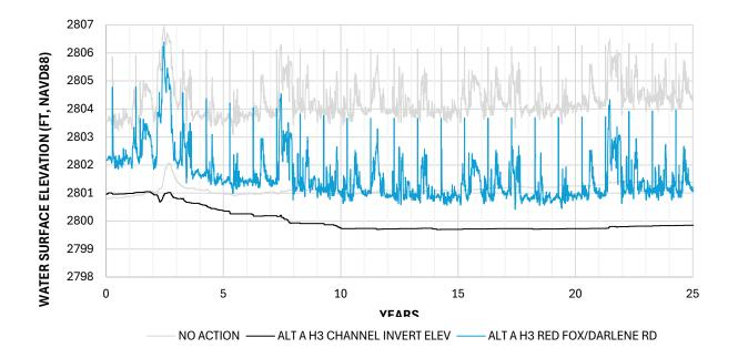
Figure B-15 Water Surface and Channel Elevation at Red Fox/Darlene Rd – No Action and Alt A H3
