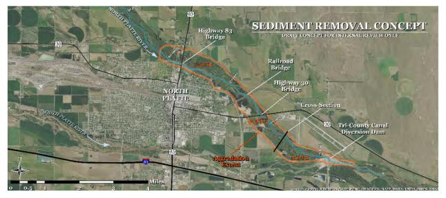
Figure 13. Sediment Removal Concept – VESPR Report (RDG 2023)
