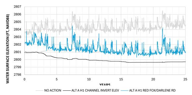
Figure B-4 Water Surface and Channel Elevation at HWY 83 - No Action and Alt A H1
