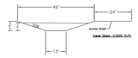
Figure 10. Bypass Canal Cross Section – 500 cfs Capacity
