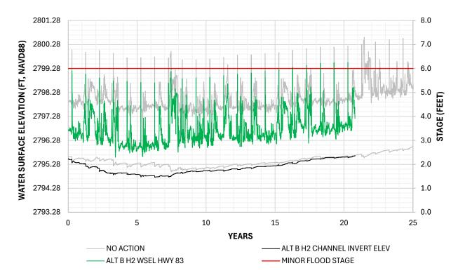
Figure C-3 Water Surface and Channel Elevation at HWY 83 – No Action and Alt B H2
