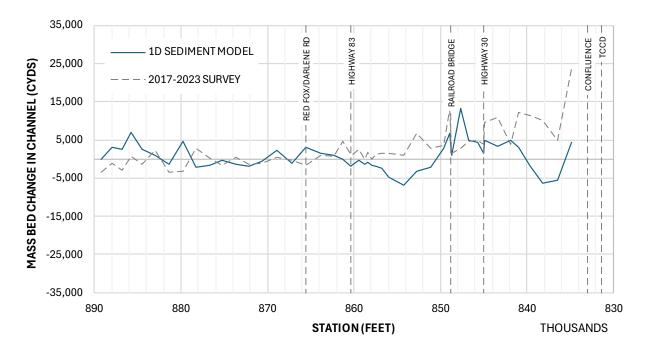
Figure 12 Mass Bed Change in Channel – Calibration Model vs Survey Data using Yang
