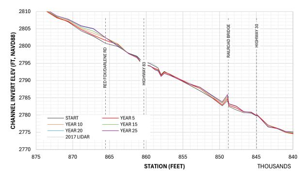
Figure F-5 Channel Profile through Time – ACE2016 Alt H2
