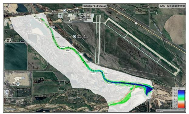
**Figure 5-8 Alt A 2D Model Results – Bed Change at Year 5** Deposition shown in green and blue, erosion shown in orange and red.
