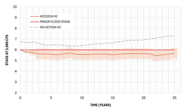
Figure F-2 Stage at HWY83 at 3,000 cfs through Time – No Action and ACE2016 Alt H2
