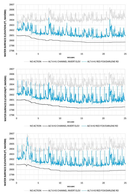
Figure 5-5 Alt A 25-Year Forecast - Water Surface and Channel Elevation at Red Fox/Darlene Rd H1 (top), H2 (middle) and H3 (bottom)
