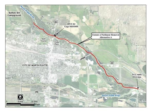
Figure B-1 Extents of Sediment Removal Alternative A
