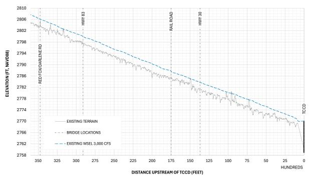
Figure 4-2 3,000 cfs Water Surface Profile - Existing Condition
