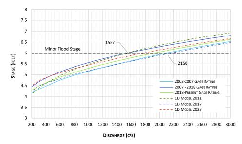
Figure 1. Stage Discharge Rating Curves at HWY 83 Gage (Gage Data and 1D Hydraulic Model)
