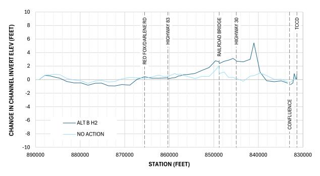
Figure C-6 Change in Channel Invert Elevation – No Action and Alt B H2
