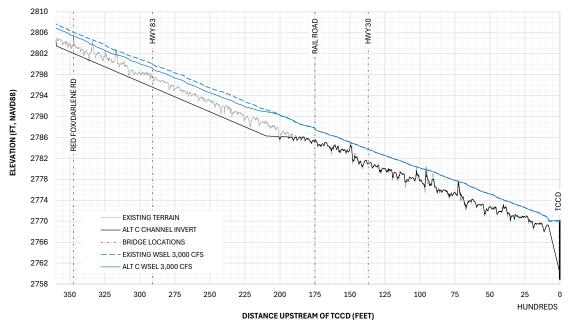
Figure D-2 3,000 cfs Water Surface Profile - Existing Condition and Alt C
