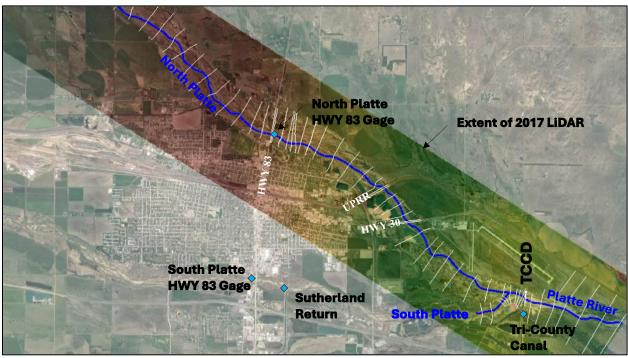
Figure 1 1D Hydraulic and Sediment Transport Model Reaches
