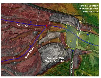
Figure 3-2 Area of Model Dredging at TCCD
