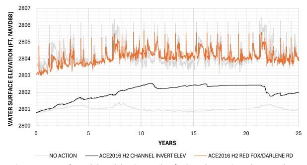
Figure F-3 Water Surface and Channel Elevation at Red Fox/Darlene Rd – No Action and ACE2016 Alt H2
