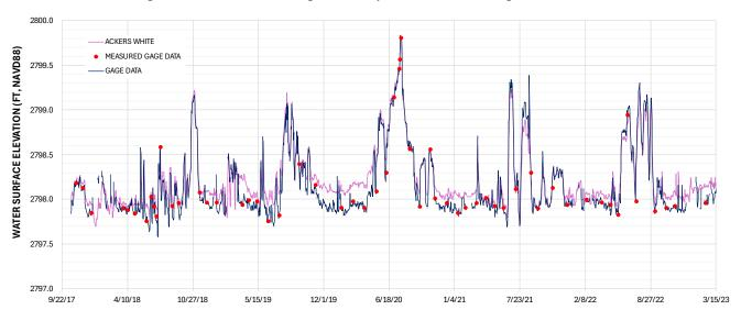
Figure 6 Model Results using Ackers White vs HWY 83 Gage Data
