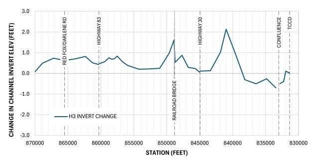
Figure A-13 Change in Channel Invert Elevation – No Action H3
