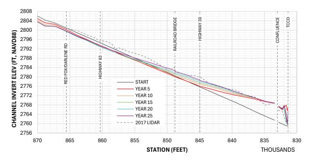
Figure B-12 Channel Profile through Time – Alt A H2
