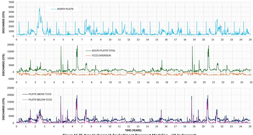
Figure 16 25-Year Hydrograph for Sediment Transport Modeling – H3 Hydrograph
