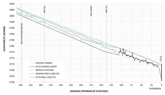
Figure C-2 3,000 cfs Water Surface Profile - Existing Condition and Alt B
