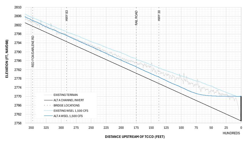
Figure 3 Existing and Sediment Removal Alt A Water Surface Profile 1.500 cfs
