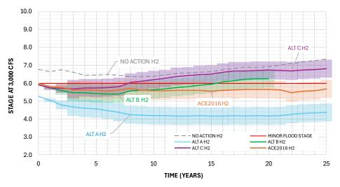
Figure 5-26 Alternative Comparisons - Stage at 3,000 cfs through Time
