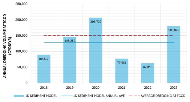
Figure 10 Comparison of Calibration Model Annual Dredging Volume at TCCD using Yang
