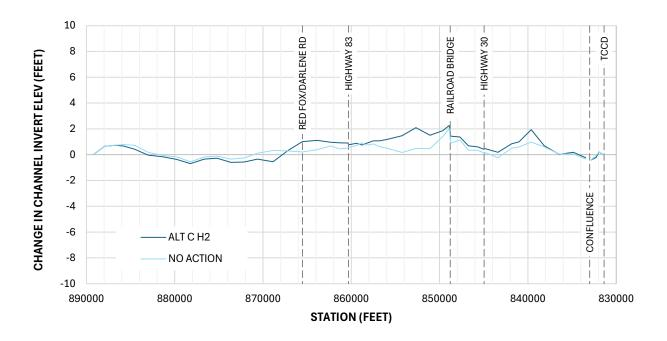
Figure D-6 Change in Channel Invert Elevation – No Action and Alt C H2
