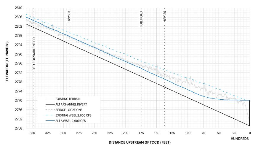
Figure 4 Existing and Sediment Removal Alt A Water Surface Profile 2,000 cfs
