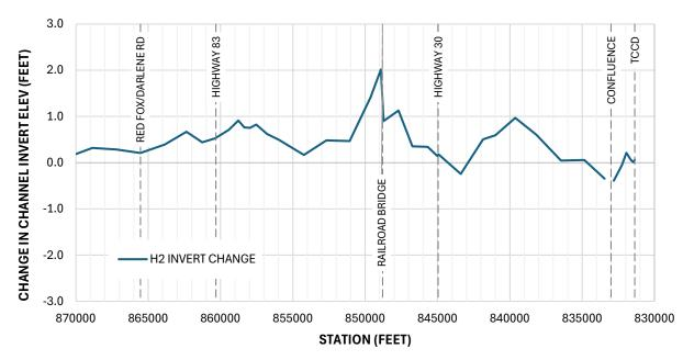
Figure A-9 Change in Channel Invert Elevation – No Action H2
