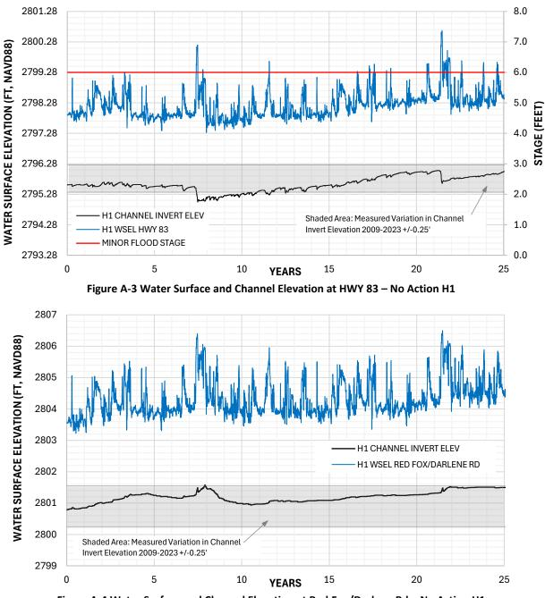
Figure A-4 Water Surface and Channel Elevation at Red Fox/Darlene Rd – No Action H1
