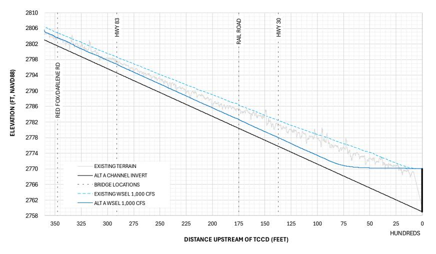
Figure 2 Existing and Sediment Removal Alt A Water Surface Profile 1,000 cfs
