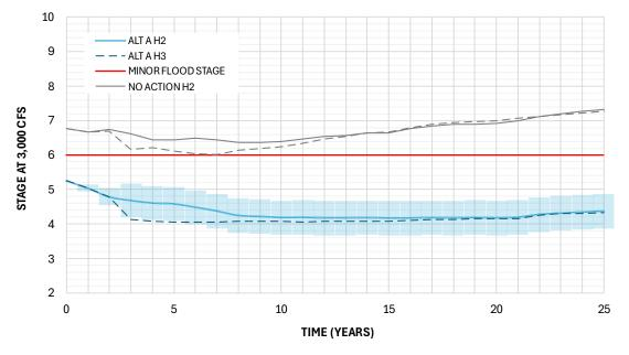
Figure 5-7 Alt A and No Action H2 and H3 25-Year Forecast - Stage at 3,000 cfs through Time
