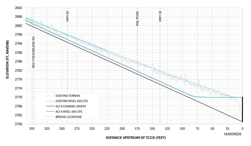
Figure 1 Existing and Sediment Removal Alt A Water Surface Profile 400 cfs (Baseflow)
