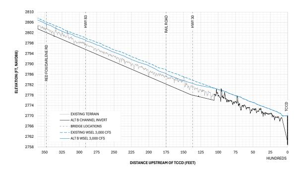
Figure 5-12 3,000 cfs Water Surface Profile - Existing Condition and Alt B
