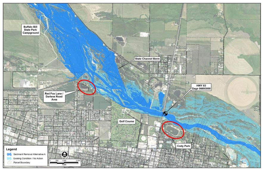
Figure B-3 North Platte Chokepoint Inundation Mapping at 3,000 cfs – Existing Conditions/No Action and Alt A
