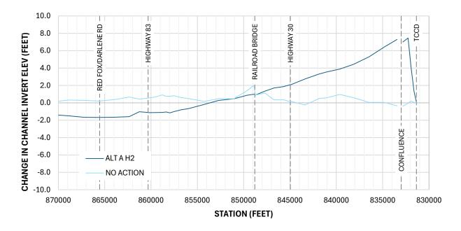
Figure B-11 Change in Channel Invert Elevation – No Action and Alt A H2
