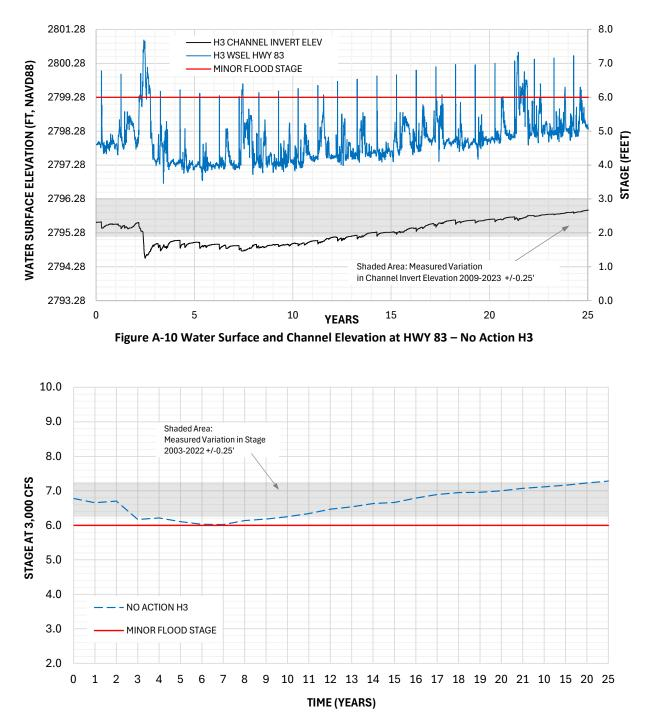
Figure A-11 Stage at HWY83 at 3,000 cfs through Time – No Action H3
