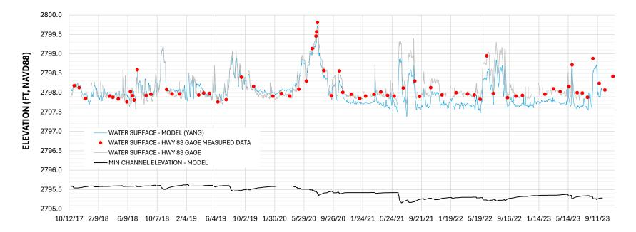
Figure 3-4 Comparison of Water Surface Elevation HWY 83 Gage vs Model 2017 - 2023
