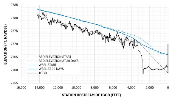
Figure 5-29 Headcut - 2D Sediment Transport Model Channel Profile
