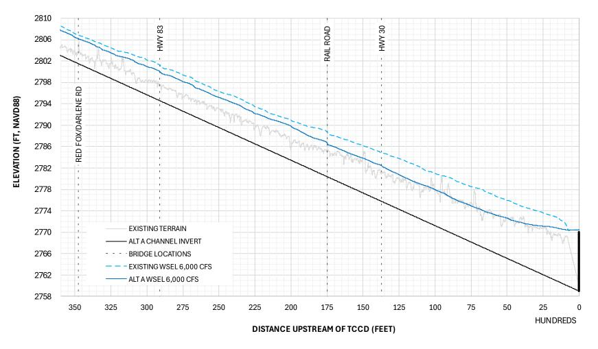
Figure 4 Existing and Sediment Removal Alt A Water Surface Profile 6,000 cfs
