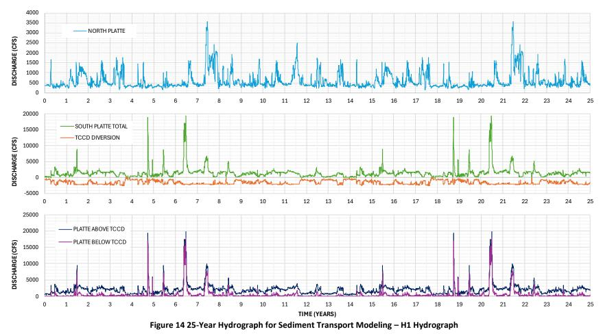
H1 Hydrograph: 2009 – 2022, 2009 – 2019, both occurrences of the 2011 flood (in year 3 and 17) were removed and replaced with 2019.
