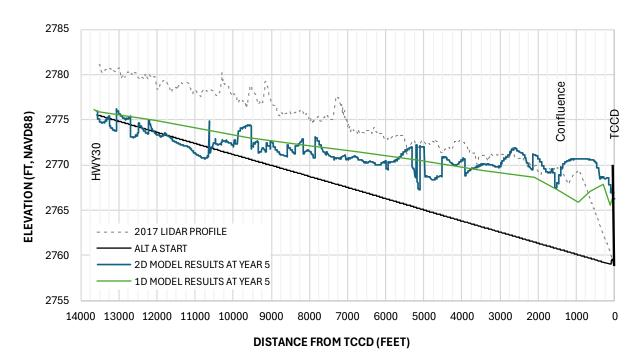
Figure 5-10 Comparison of Alt A 1D and 2D Sediment Model Results – Channel Profile at Start and Year 5.
