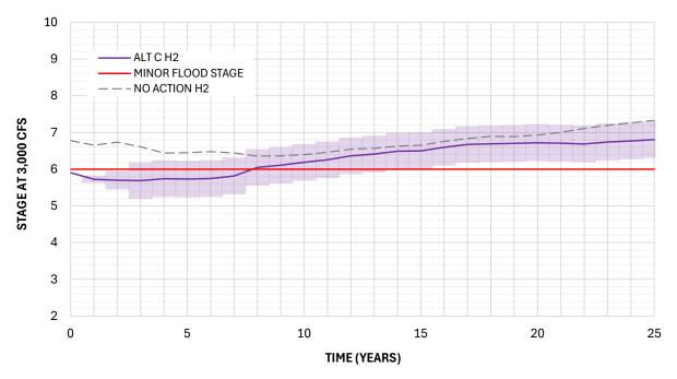
Figure D-4 Stage at HWY83 at 3,000 cfs through Time – No Action and Alt C H2
