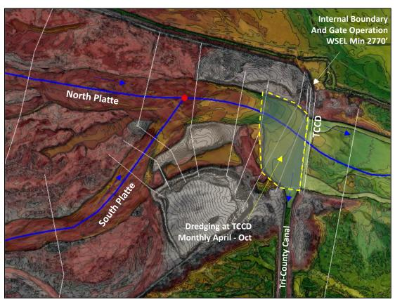
Figure 3 Area of Model Dredging at TCCD
