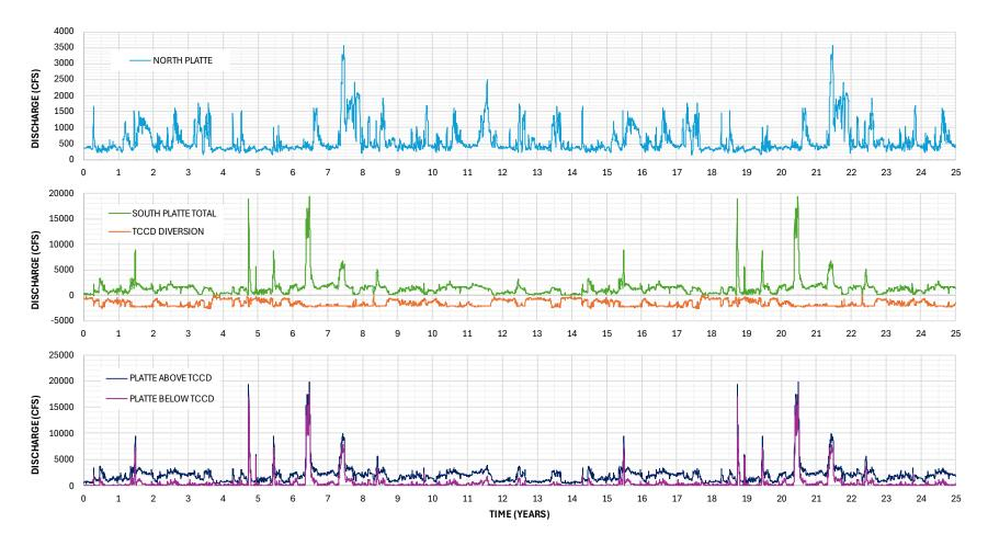
Figure 3-8 25-Year Hydrograph for Sediment Transport Modeling – H1 Hydrograph
