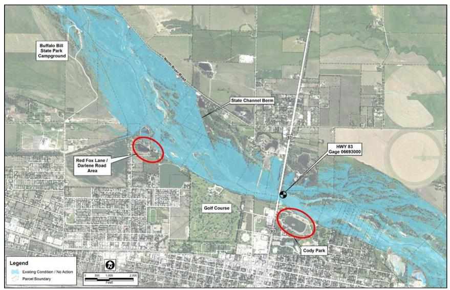
Figure A-2 North Platte Chokepoint Inundation Mapping at 3,000 cfs – Existing Conditions/No Action
