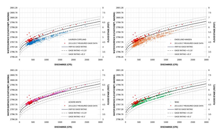
Figure 9 Stage Discharge Rating Curves at HWY 83 Gage – 1D Sediment Transport Model Results 2017-2023 using 4 Transport Equations Upper Left: Larsen Copeland, Upper Right: Engelund Hansen, Lower Left: Ackers White, and Lower Right: Yang
