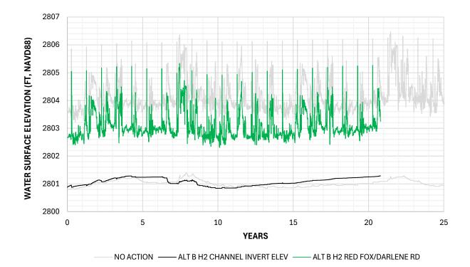
Figure C-5 Water Surface and Channel Elevation at Red Fox/Darlene Rd – No Action and Alt B H2
