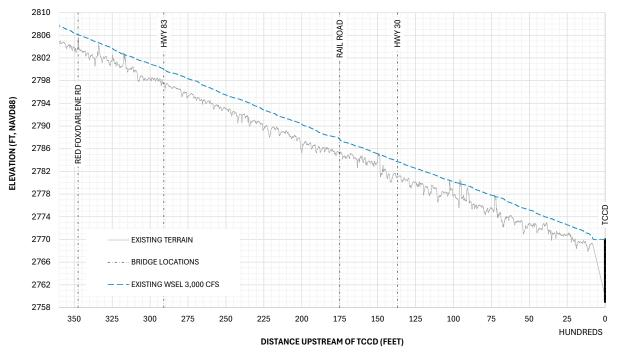
Figure A-1 3,000 cfs Water Surface Profile - Existing Condition/No Action
