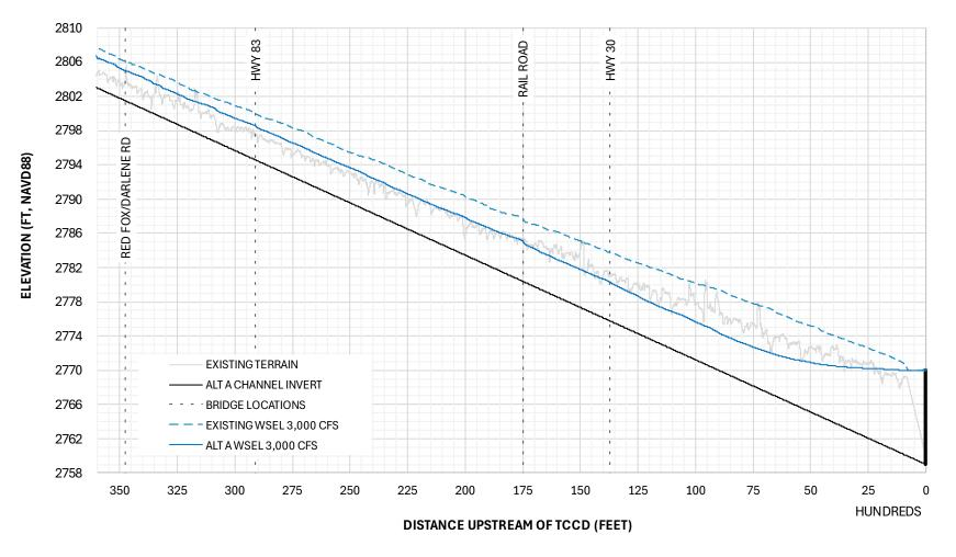
Figure 4 Existing and Sediment Removal Alt A Water Surface Profile 3,000 cfs
