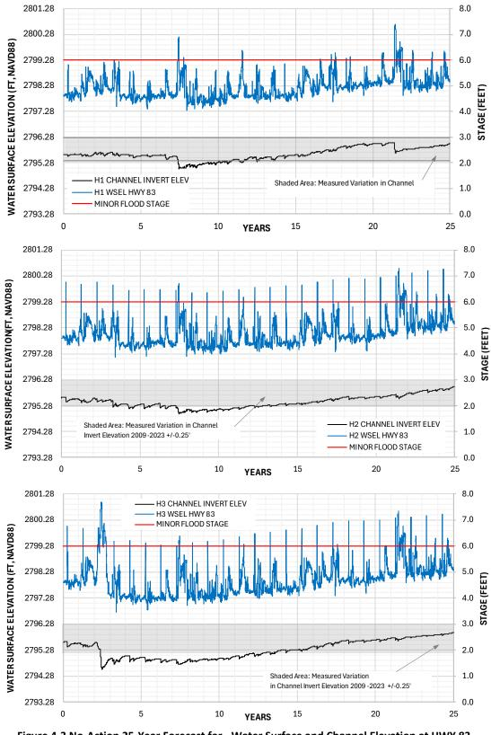
Figure 4-3 No-Action 25-Year Forecast for - Water Surface and Channel Elevation at HWY 83 H1 (top), H2 (middle) and H3 (bottom)
