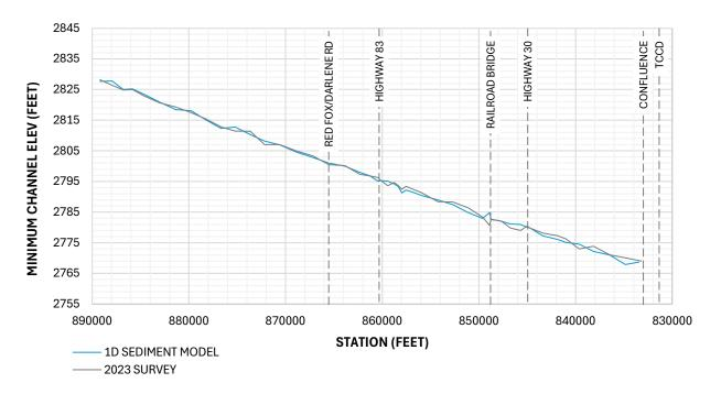
Figure 3-6 Channel Profile Comparison – Model vs 2023 Survey
