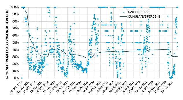
Figure 13 Percent of Sediment Load from North Platte over Calibration Period
