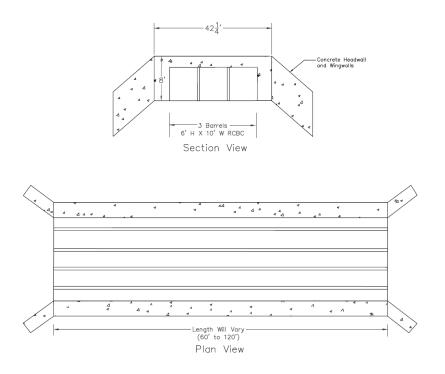
Figure 11. Typical Canal Road Crossing Structure – 500 cfs Canal
