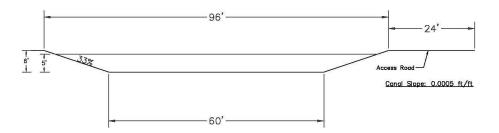
*Figure 7.* Bypass Canal Section – 1,500 cfs Capacity
