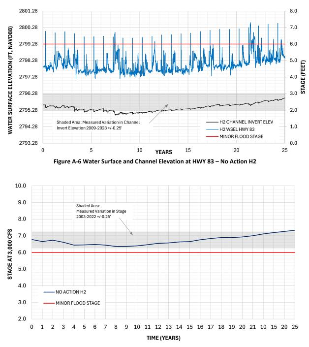
Figure A-7 Stage at HWY83 at 3,000 cfs through Time – No Action H2
