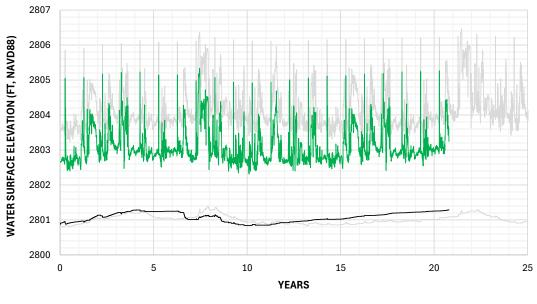
Figure 5-14 Alt B 25-Year Forecast - Water Surface and Channel Elevation at Red Fox/Darlene Rd
