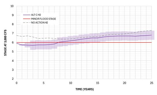
Figure 5-20 Alt C H2 25-Year Forecast - Stage at 3,000 cfs through Time
