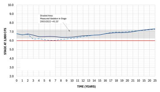
Figure 4-5 No-Action H2 and H3 25-Year Forecast - Stage at 3,000 cfs through Time
