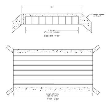
Figure 8. Typical Canal Road Crossing Structure – 1,500 cfs Canal
