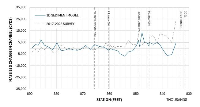
Figure 3-7 Mass Bed Change in Channel – Model vs Survey Data
