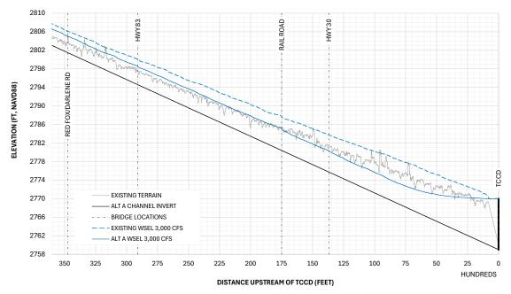
Figure B-2 3,000 cfs Water Surface Profile - Existing Condition/No Action and Alt A
