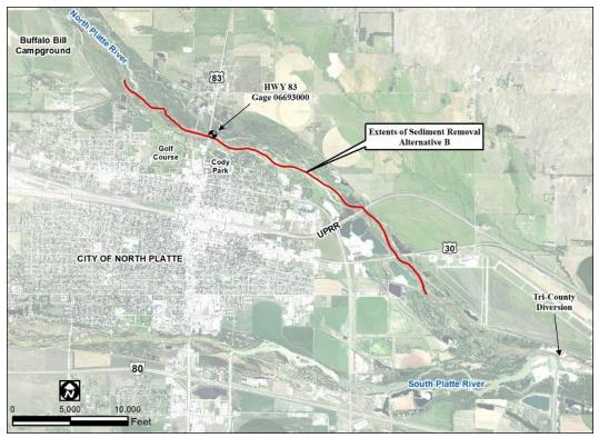
Figure 5-11 Extents of Sediment Removal Alternative B
