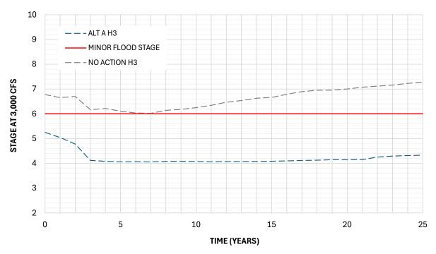
Figure B-14 Stage at HWY83 at 3,000 cfs through Time – No Action and Alt A H3
