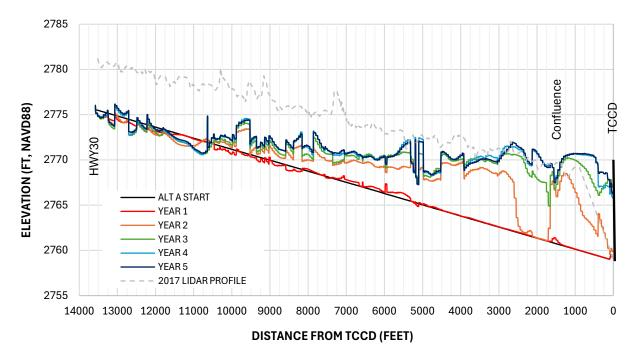
Figure 5-9 Alt A 2D Sediment Model Results – Channel Profile Year 1 through 5.
