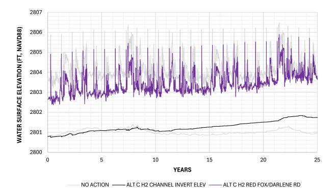
Figure D-5 Water Surface and Channel Elevation at Red Fox/Darlene Rd – No Action and Alt C H2
