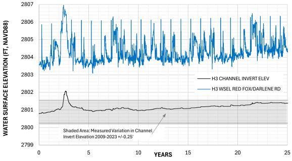
Figure A-12 Water Surface and Channel Elevation at Red Fox/Darlene Rd – No Action H3
