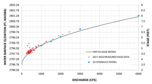
Figure 2 Measured Data vs 1D Hydraulic Model - Stage vs Discharge at HWY 83 Gage
