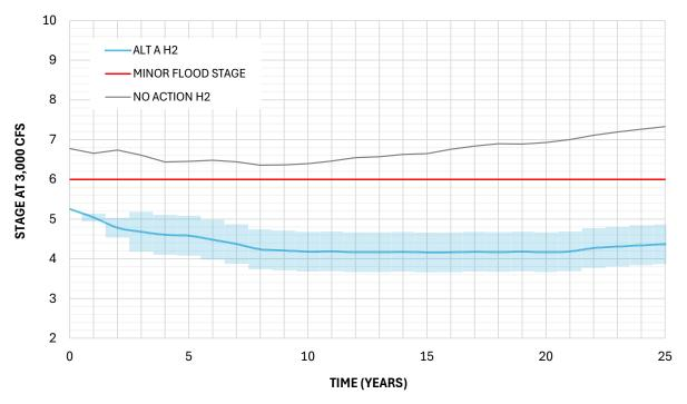
Figure B-9 Stage at HWY83 at 3,000 cfs through Time – No Action and Alt A H2
