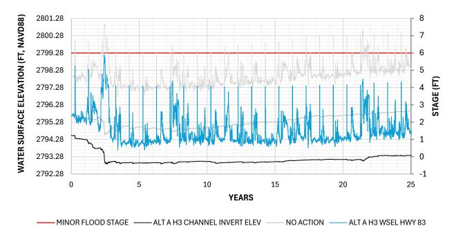
Figure B-13 Water Surface and Channel Elevation at HWY 83 – No Action and Alt A H3
