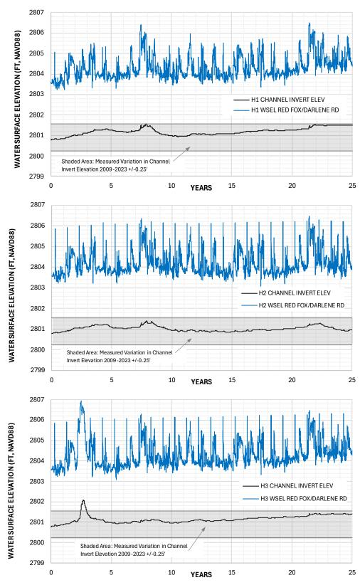
Figure 4-4 No-Action 25-Year Forecast - Water Surface and Channel Elevation at Red Fox/Darlene Rd H1 (top), H2 (middle) and H3 (bottom)
