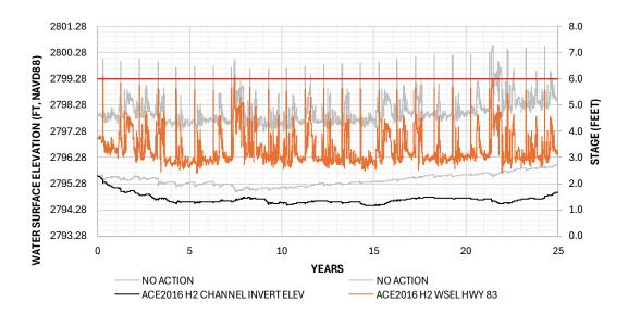
Figure 5-22 Mod ACE 2016 Alt 25-Year Forecast - Water Surface and Channel Elevation at HWY 83
