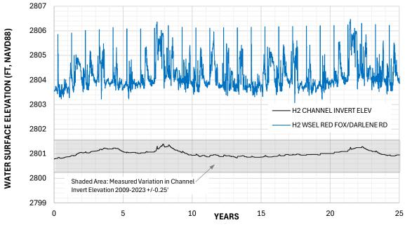
Figure A-8 Water Surface and Channel Elevation at Red Fox/Darlene Rd – No Action H2
