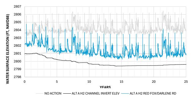
Figure B-10 Water Surface and Channel Elevation at Red Fox/Darlene Rd – No Action and Alt A H2
