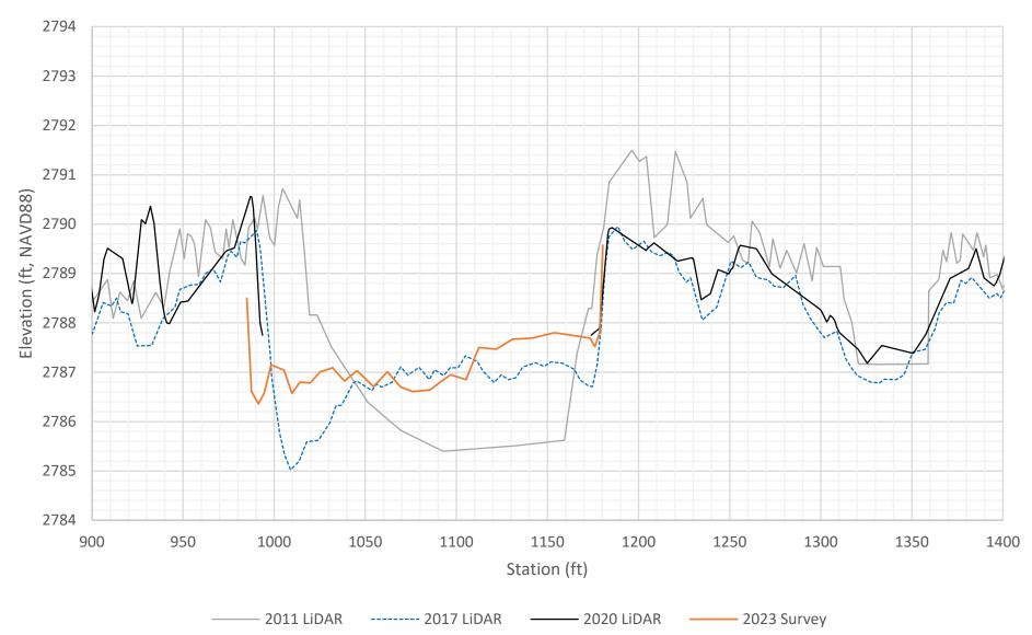
NORTH PLATTE RIVER CROSS SECTION COMPARISON CROSS SECTION 851072.7
