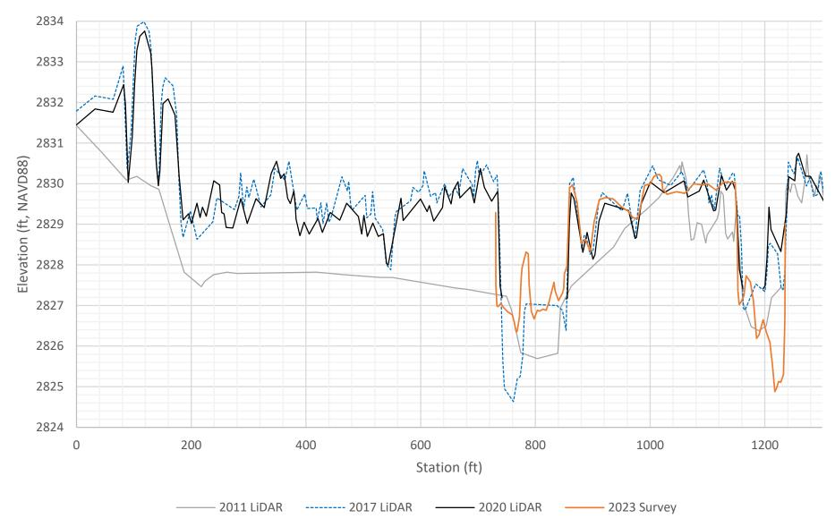
NORTH PLATTE RIVER CROSS SECTION COMPARISON CROSS SECTION 886787.3
