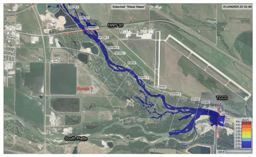
Figure E-25 Shear Stress (lbs/ft2) Mapping 400 cfs – HWY 30 to Tri-County Diversion
