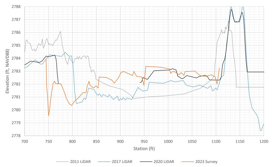
NORTH PLATTE RIVER CROSS SECTION COMPARISON CROSS SECTION 845678.8
