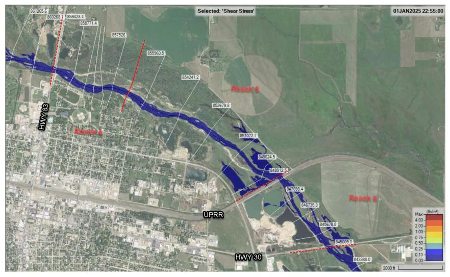
Figure E-24 Shear Stress (lbs/ft2) Mapping 400 cfs – HWY 83 to HWY 30
