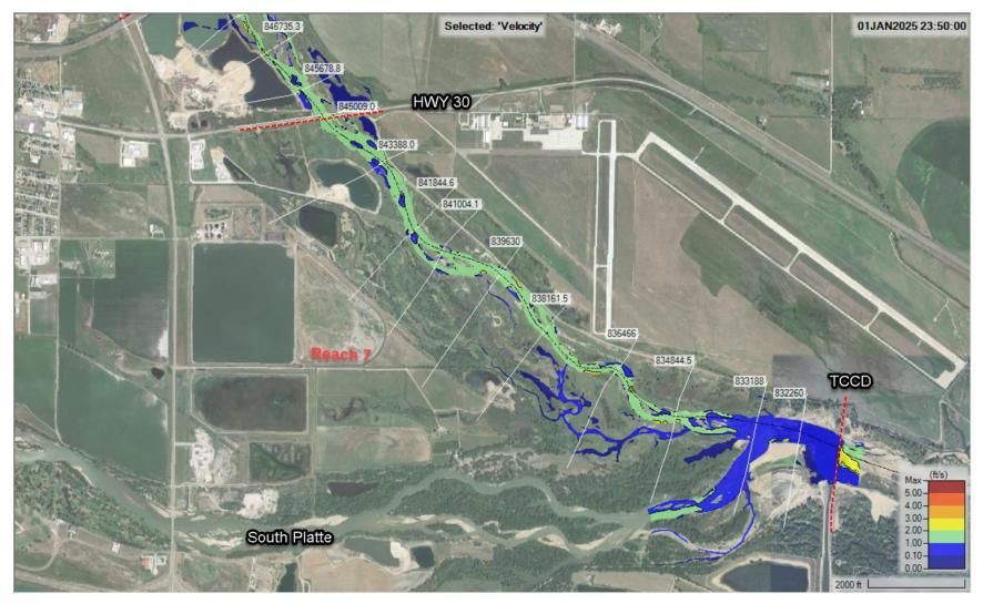
Figure E-21 Velocity (ft/sec) Mapping 400 cfs – HWY 30 to Tri-County Diversion
