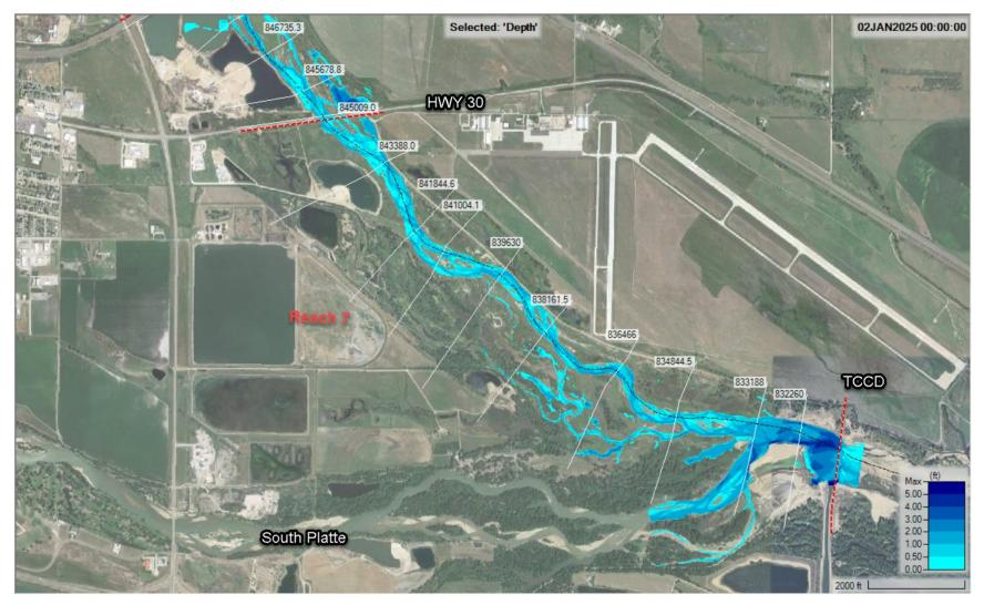
Figure E-4 Inundation Mapping 400 cfs – HWY 30 to Tri-County Diversion
