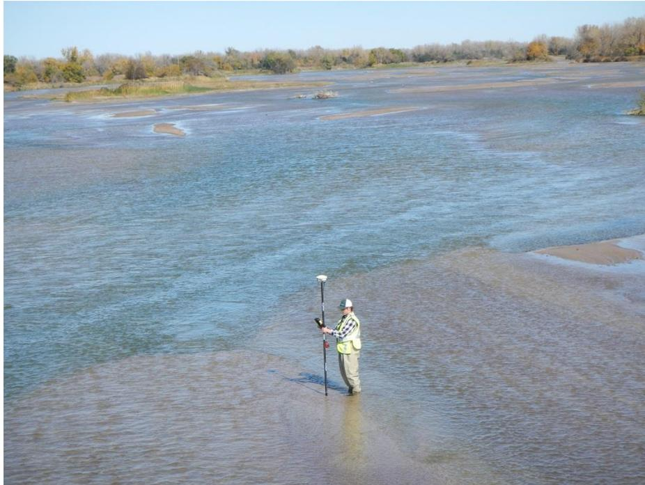
Top image: QSI ground surveying professional collecting submerged bathymetric check point data.
