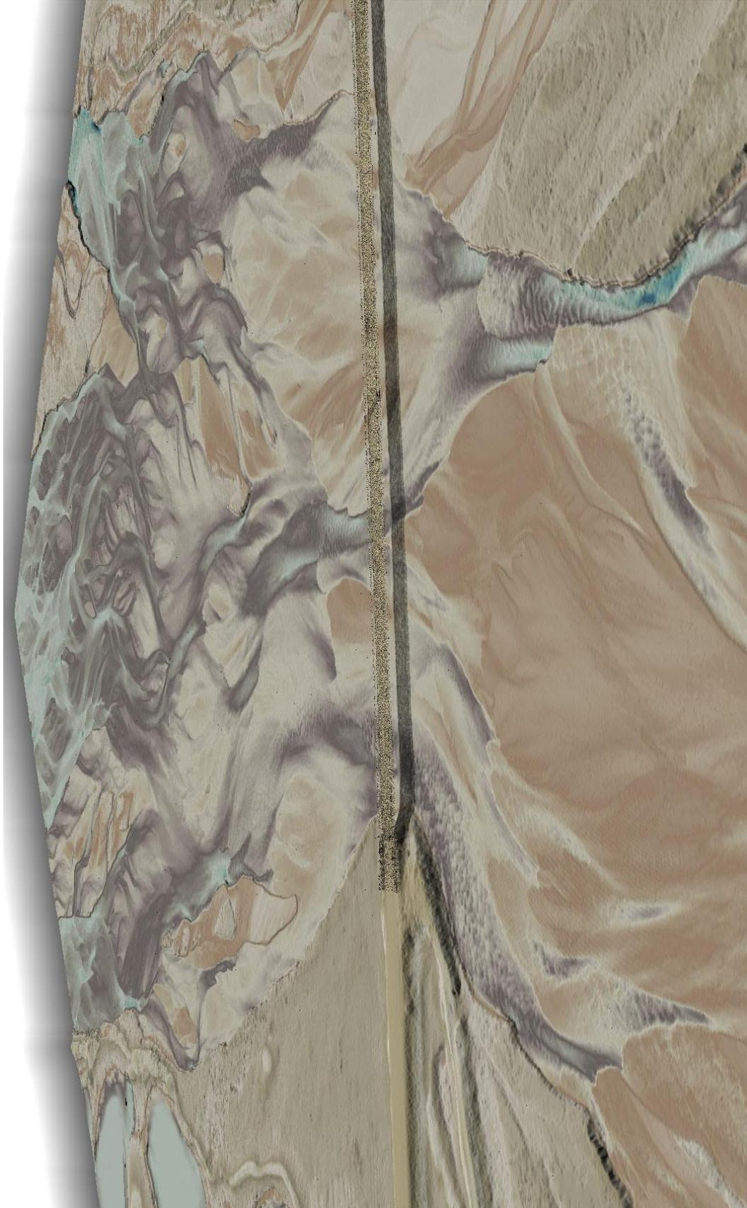
**Figure 21:** This view of the Chapman Bridge crossing over the Platte River shows the incredible detail captured by the bathymetric LIDAR survey. The image was created from the gridded bare earth and bathymetric bottom classified returns, colored by elevation.
