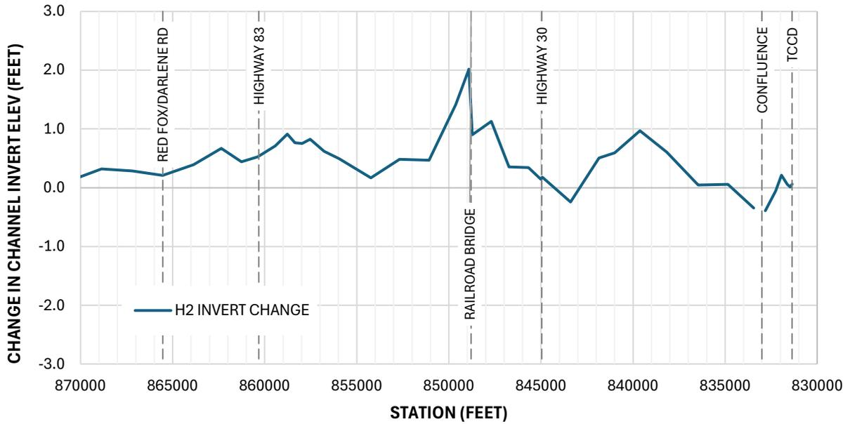
Figure A-9 Change in Channel Invert Elevation – No Action H2
