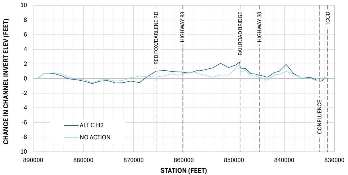
Figure D-6 Change in Channel Invert Elevation – No Action and Alt C H2
