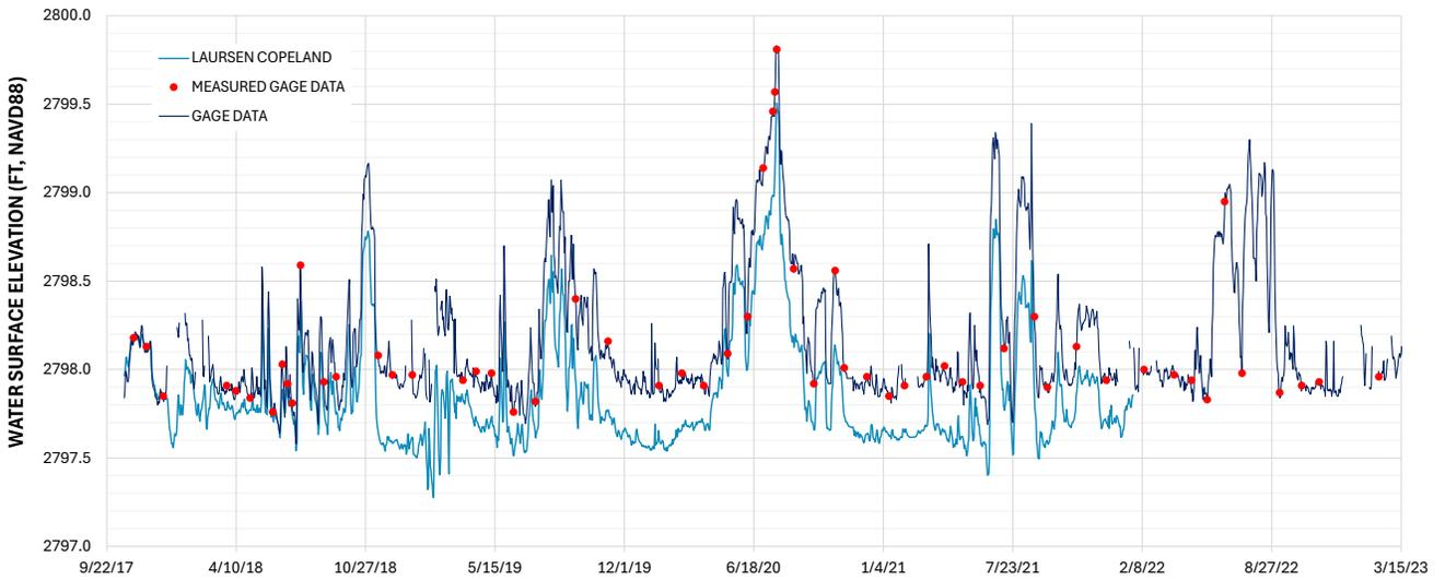
**Figure 5 Model Results using Larsen Copeland vs HWY 83 Gage Data**
