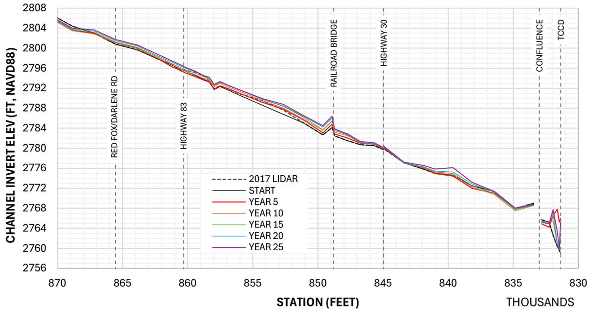
Figure D-7 Channel Profile through Time – Alt C H2
