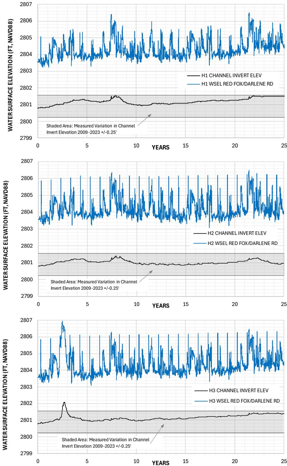
Figure 4-4 No-Action 25-Year Forecast - Water Surface and Channel Elevation at Red Fox/Darlene Rd
