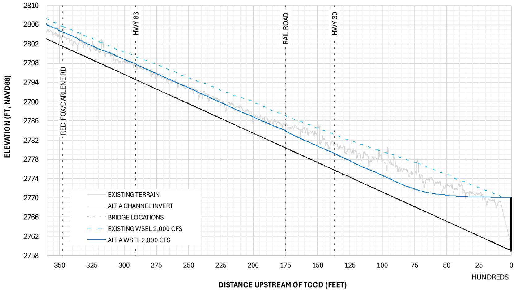
**Figure 4 Existing and Sediment Removal Alt A Water Surface Profile 2,000 cfs**
