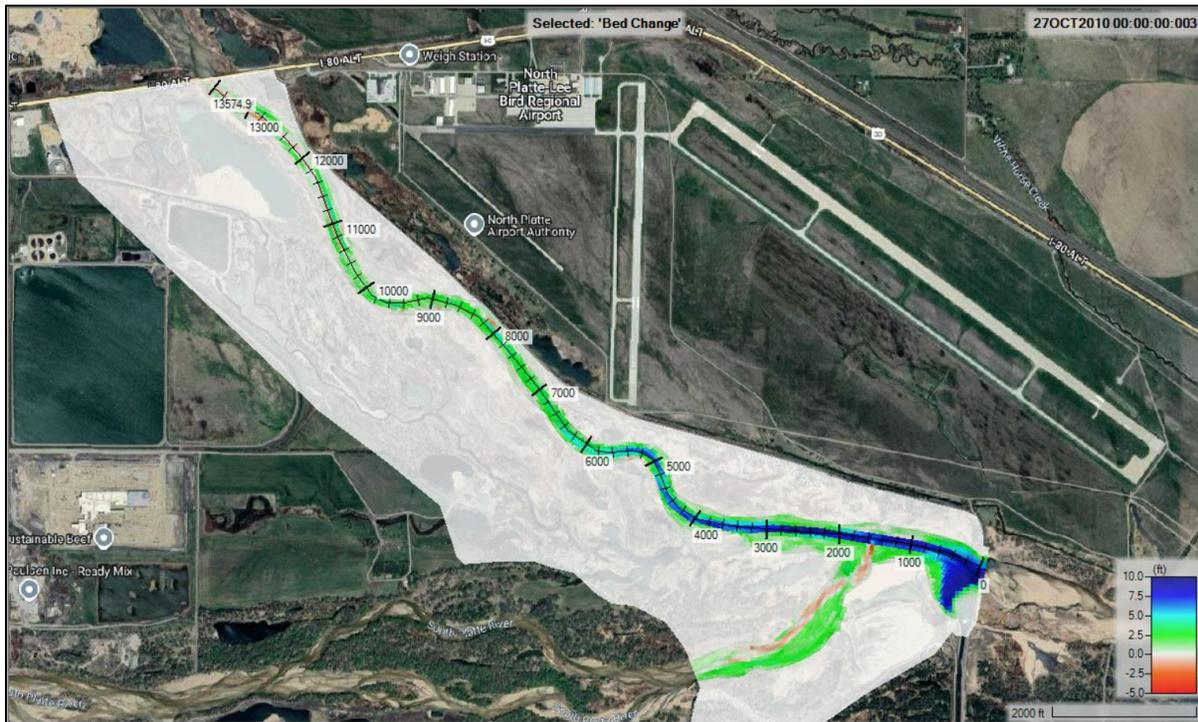
**Figure 5-8 Alt A 2D Model Results – Bed Change at Year 5**
