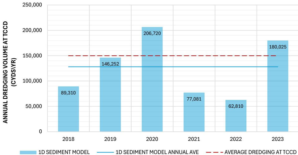
**Figure 10 Comparison of Calibration Model Annual Dredging Volume at TCCD using Yang**
