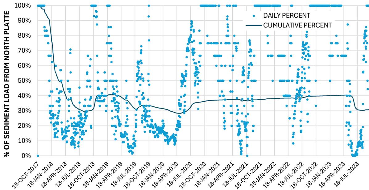
**Figure 13 Percent of Sediment Load from North Platte over Calibration Period**
