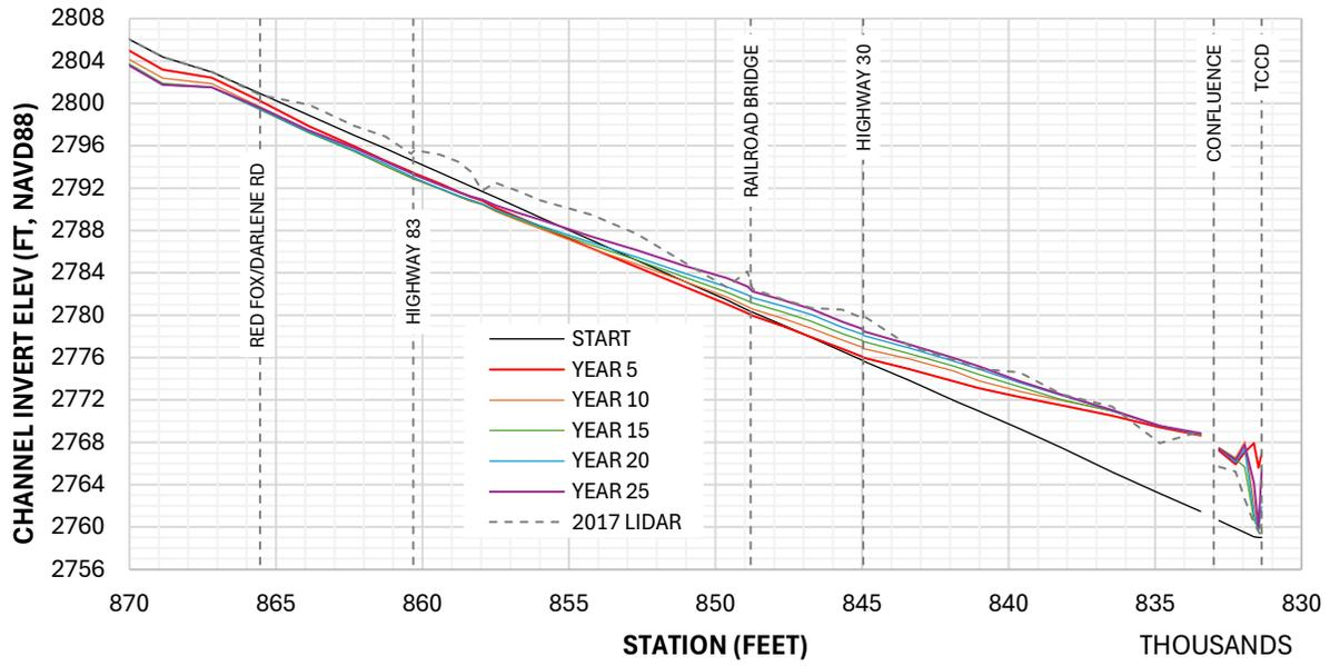
Figure B-12 Channel Profile through Time – Alt A H2
