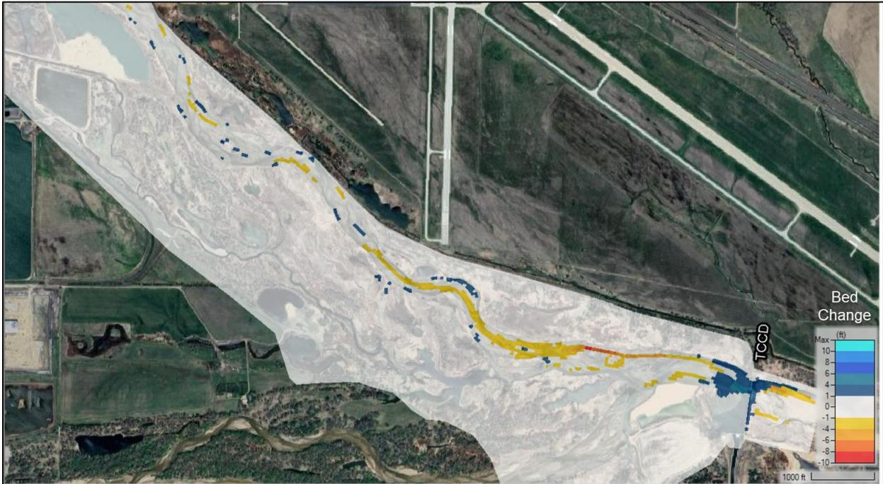
Figure 5-30 Headcut - 2D Sediment Transport Model Bed Change
