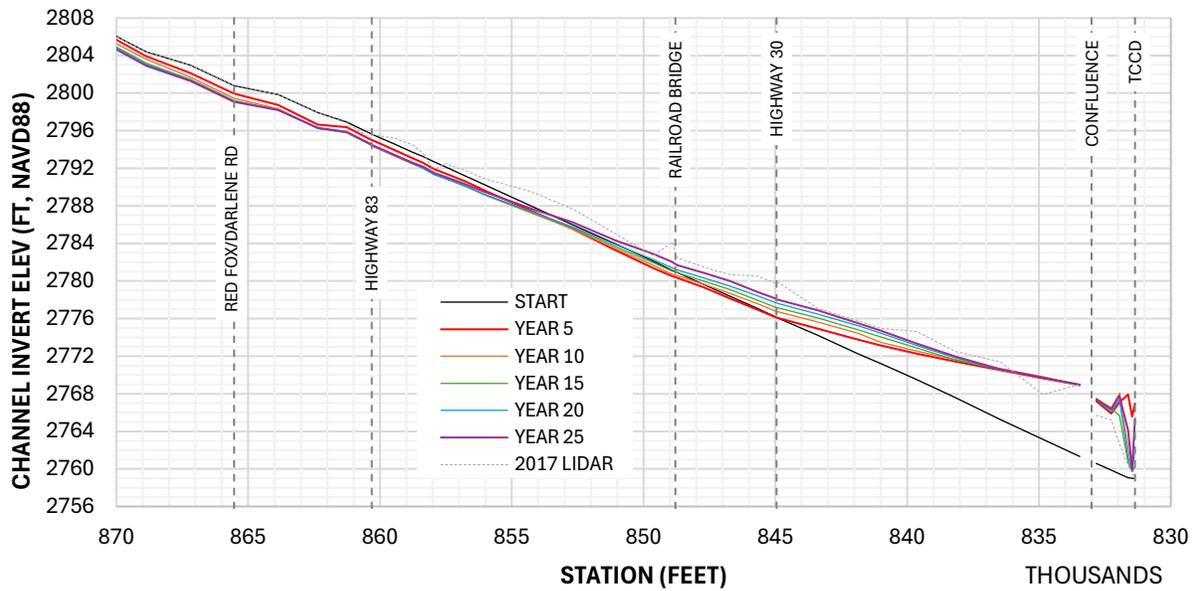
Figure B-7 Channel Profile through Time – Alt A H1
