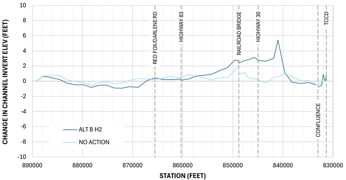
Figure C-6 Change in Channel Invert Elevation – No Action and Alt B H2
