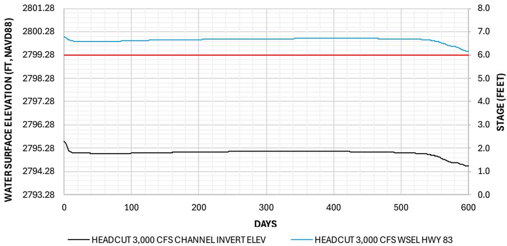
Figure 5-28 Headcut - Water Surface and Channel Elevation at HWY 83
