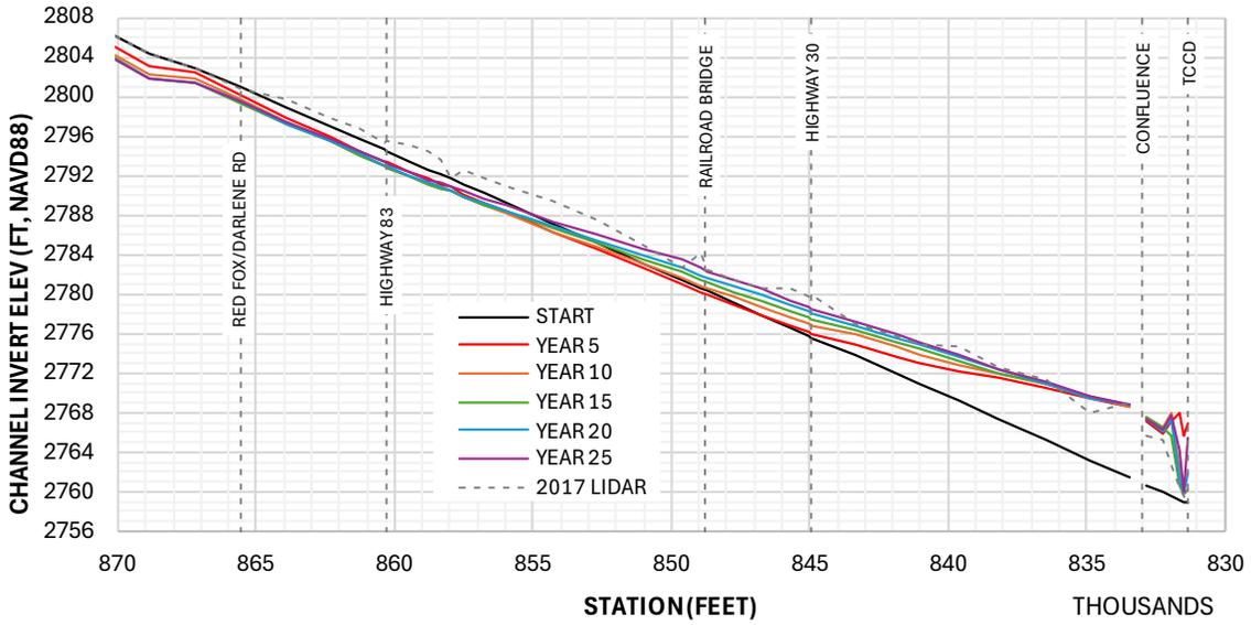
Figure 5-6 Alt A Progression of Channel Profile
