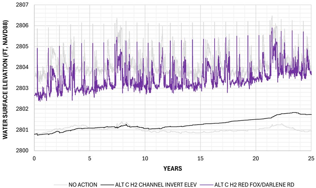
**Figure 5-19 Alt C 25-Year Forecast - Water Surface and Channel Elevation at Red Fox/Darlene Rd**
