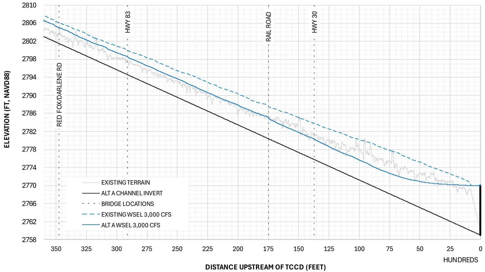
**Figure 4 Existing and Sediment Removal Alt A Water Surface Profile 3,000 cfs**
