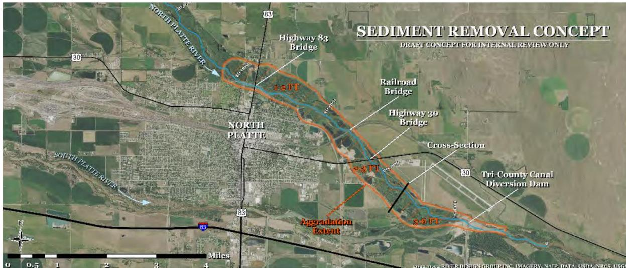
Figure 13. Sediment Removal Concept – VESPR Report (RDG 2023)
