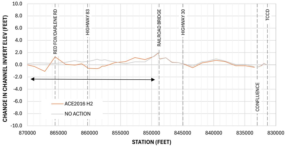
Figure F-4 Change in Channel Invert Elevation – No Action and ACE2016 Alt H2
