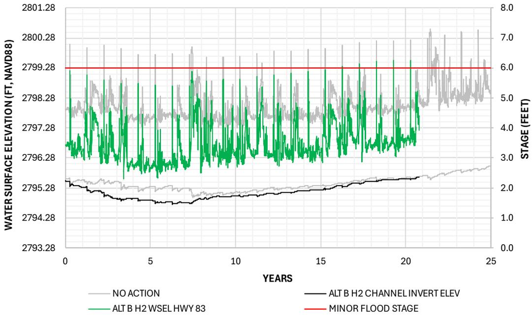
**Figure 5-13 Alt B 25-Year Forecast - Water Surface and Channel Elevation at HWY 83**
