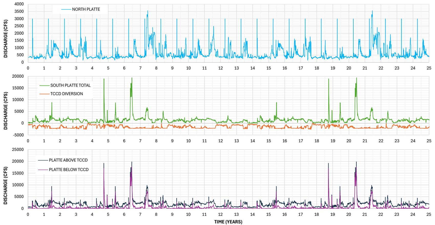
**Figure 3-9 25-Year Hydrograph for Sediment Transport Modeling – H2 Hydrograph**
