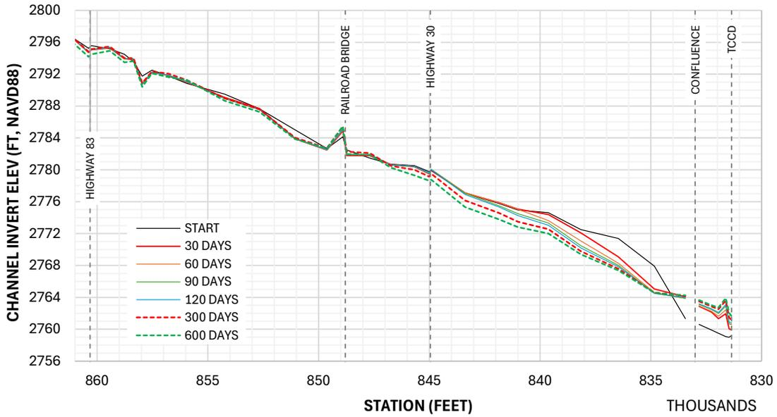
Figure 5-27 Headcut Progression of Channel Profile
