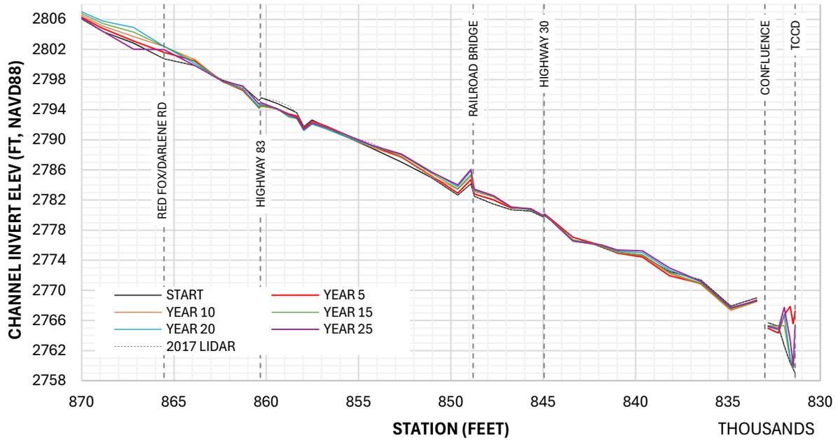
Figure 5-24 Mod ACE 2016 Alt Progression of Channel Profile
