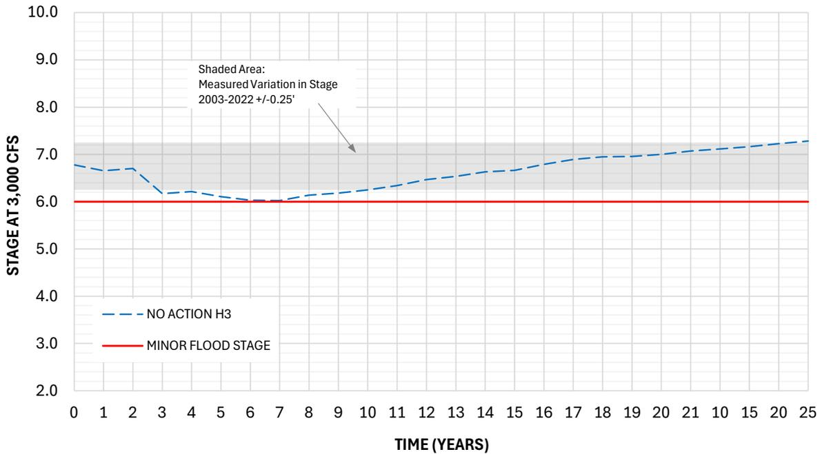
Figure A-11 Stage at HWY83 at 3,000 cfs through Time – No Action H3
