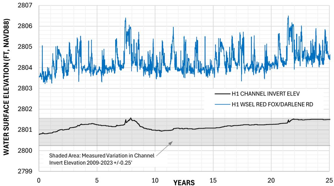
Figure A-4 Water Surface and Channel Elevation at Red Fox/Darlene Rd – No Action H1
