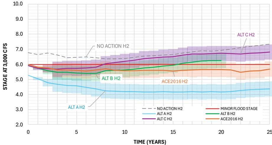
Figure 5-26 Alternative Comparisons - Stage at 3,000 cfs through Time
