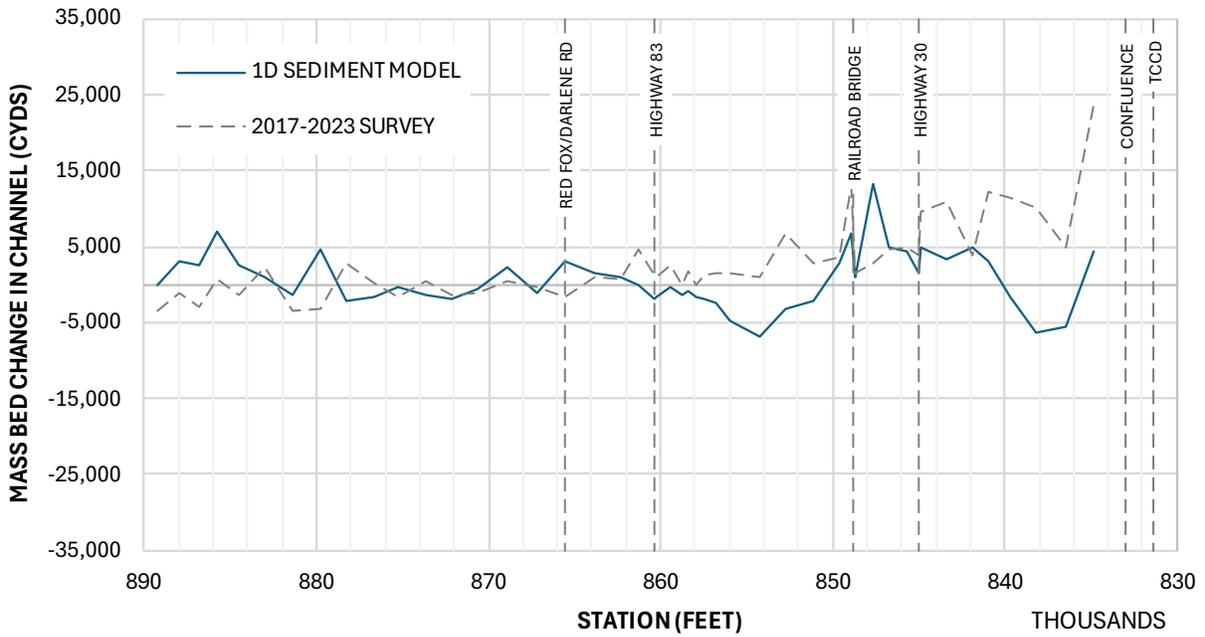
**Figure 12 Mass Bed Change in Channel – Calibration Model vs Survey Data using Yang**
