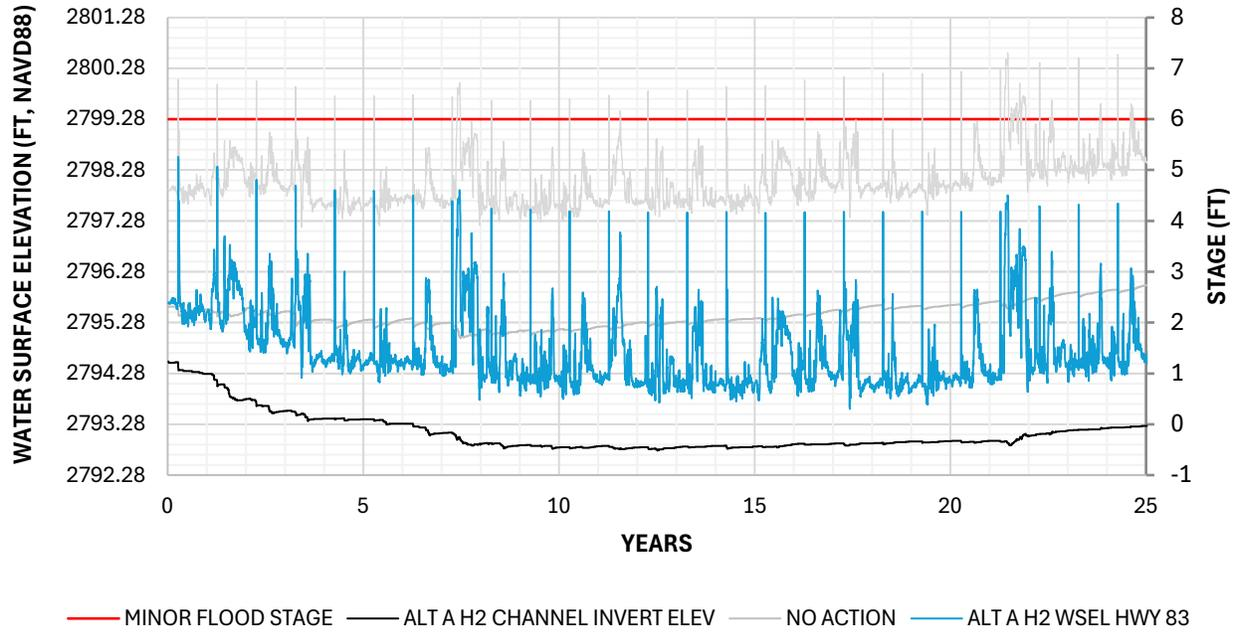
Figure B-8 Water Surface and Channel Elevation at HWY 83 – No Action and Alt A H2
