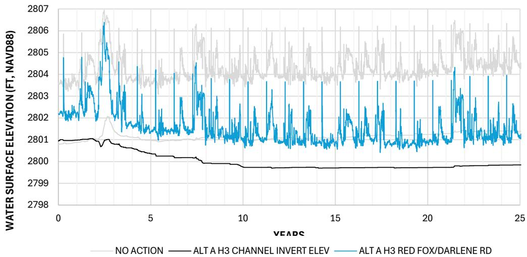
**Figure 5-5 Alt A 25-Year Forecast - Water Surface and Channel Elevation at Red Fox/Darlene Rd**
