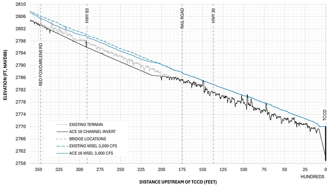
**Figure 5-21 3,000 cfs Water Surface Profile - Existing Condition and Modified ACE 2016 Alt**
