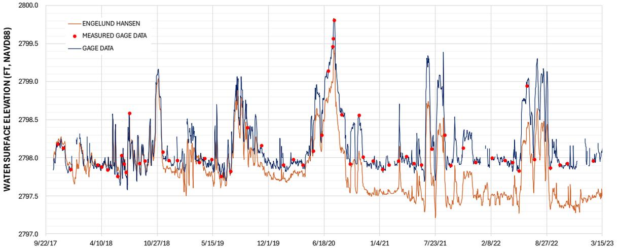
**Figure 7 Model Results using Engelund Hansen vs HWY 83 Gage Data**
