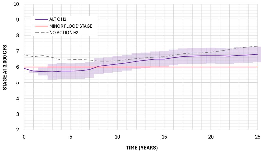
Figure 5-20 Alt C H2 25-Year Forecast - Stage at 3,000 cfs through Time
