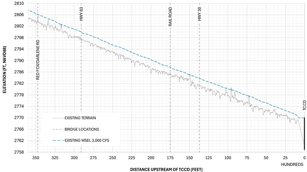
**Figure 4-2 3,000 cfs Water Surface Profile - Existing Condition**
