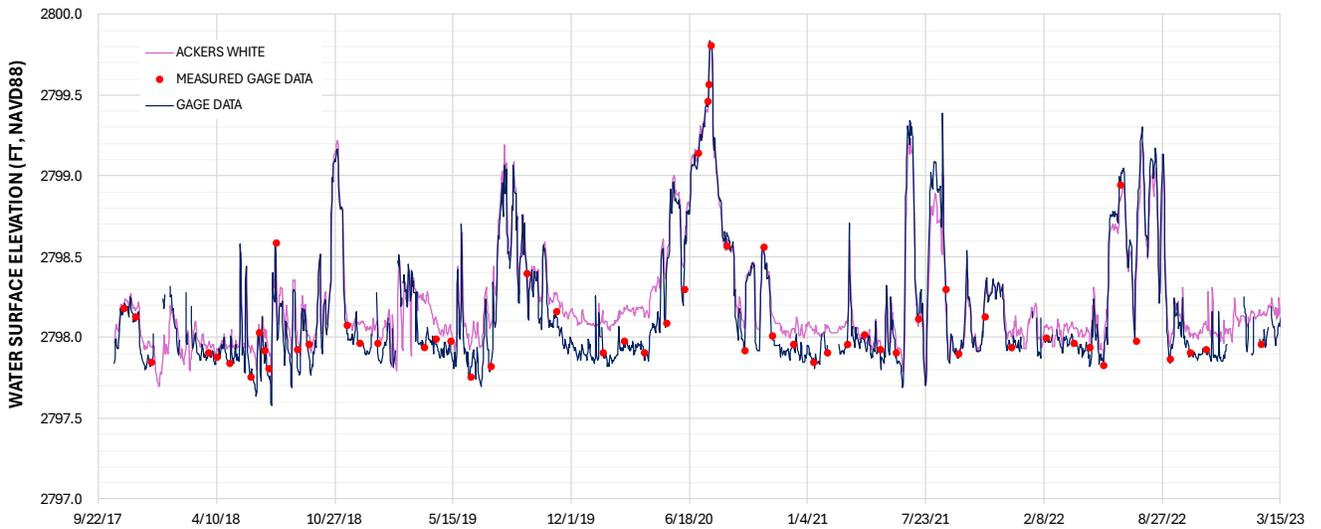
**Figure 6 Model Results using Ackers White vs HWY 83 Gage Data**
