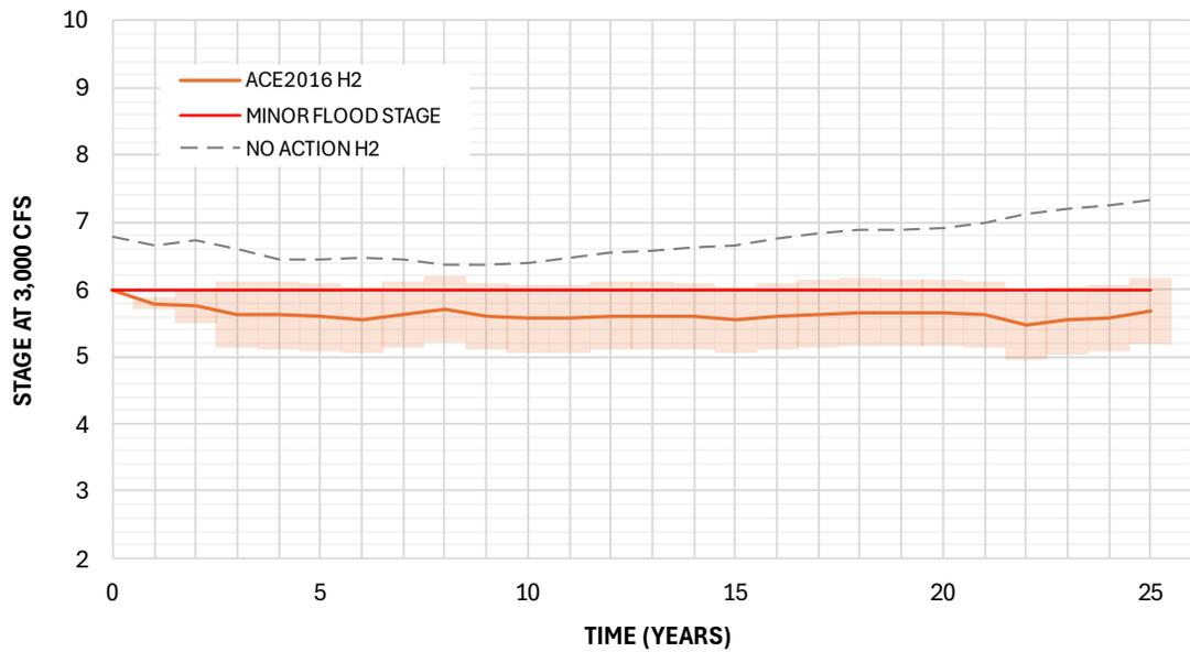
Figure 5-25 Mod ACE 2016 H2 25-Year Forecast - Stage at 3,000 cfs through Time
