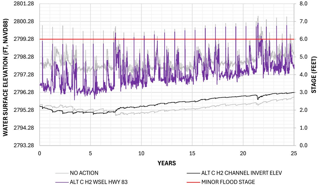
Figure D-3 Water Surface and Channel Elevation at HWY 83 – No Action and Alt C H2
