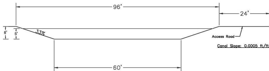
**Figure 7.** Bypass Canal Section – 1,500 cfs Capacity
