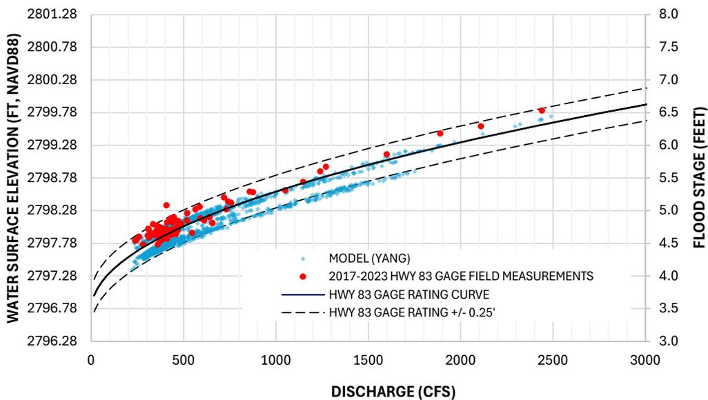
**Figure 3-3 Stage-Discharge Curve at HWY 83 Gage – Gage Data vs Model 2017-2023**
