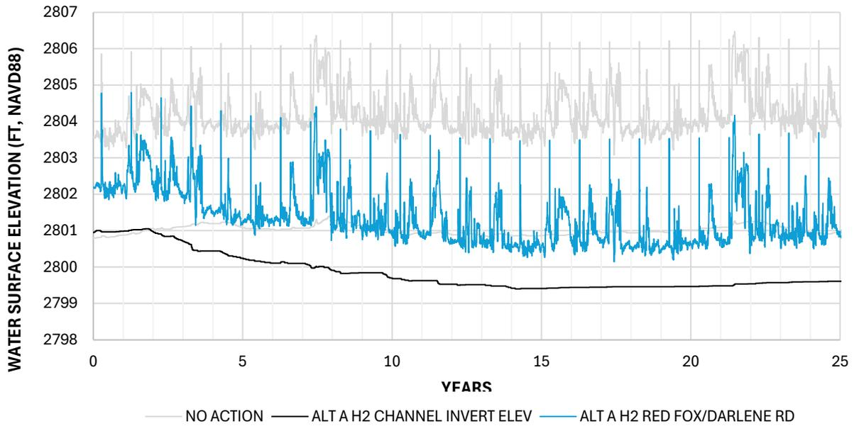
**Figure B-10 Water Surface and Channel Elevation at Red Fox/Darlene Rd – No Action and Alt A H2**
