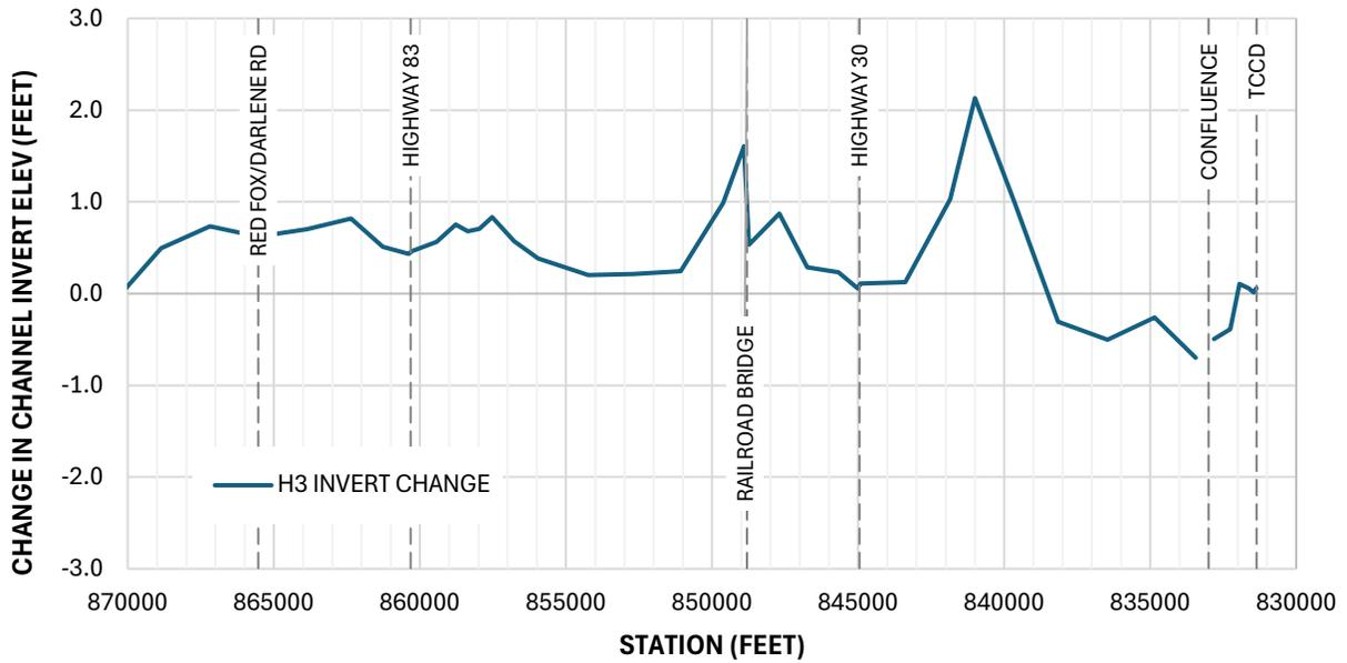
Figure A-13 Change in Channel Invert Elevation – No Action H3
