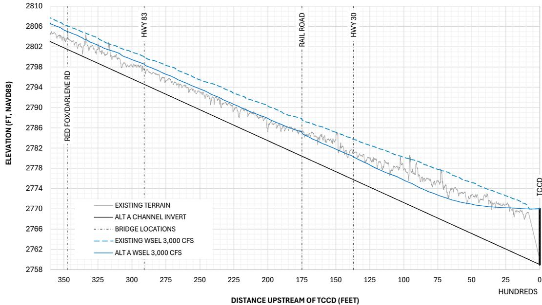
Figure 5-2 3,000 cfs Water Surface Profile - Existing Condition and Alt A
