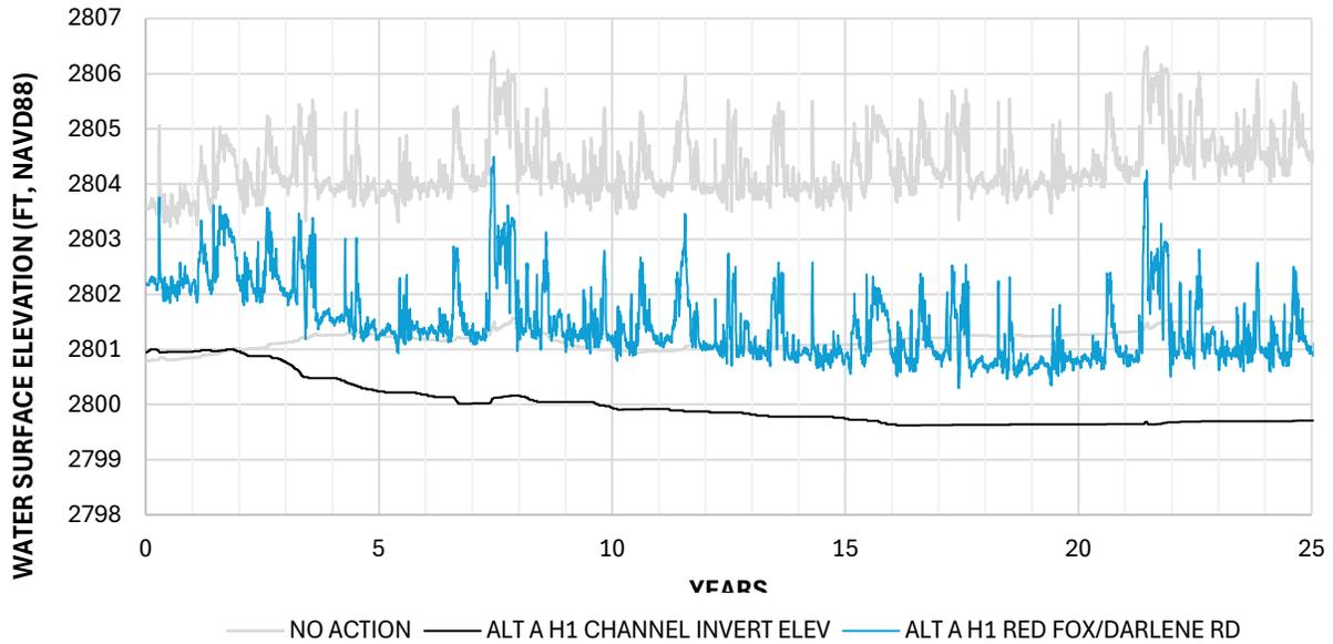
**Figure B-5 Water Surface and Channel Elevation at Red Fox/Darlene Rd – No Action and Alt A H1**
