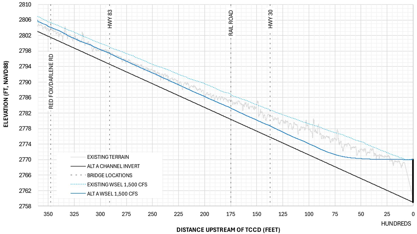
**Figure 3 Existing and Sediment Removal Alt A Water Surface Profile 1.500 cfs**
