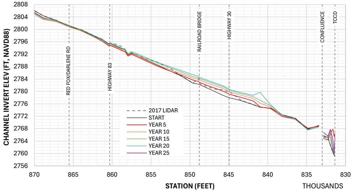
Figure C-7 Channel Profile through Time – Alt B H2
