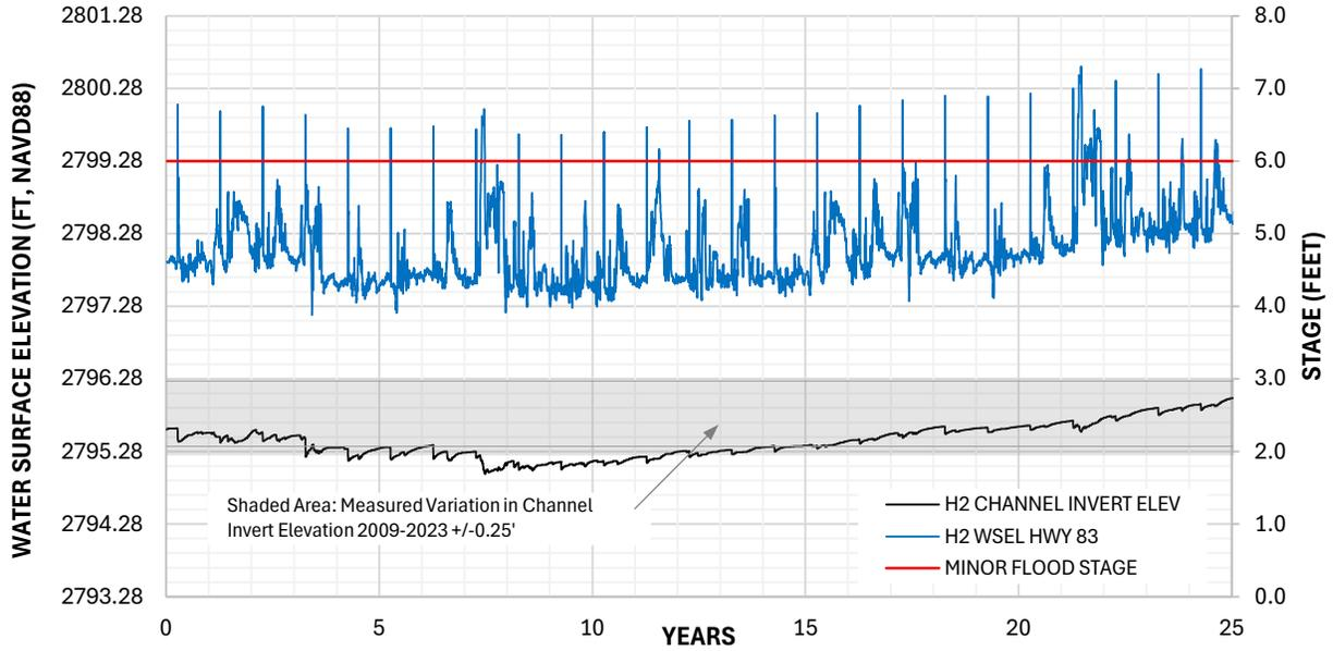
Figure A-6 Water Surface and Channel Elevation at HWY 83 – No Action H2
