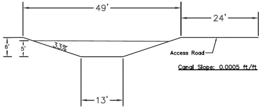
**Figure 10.** Bypass Canal Cross Section – 500 cfs Capacity
