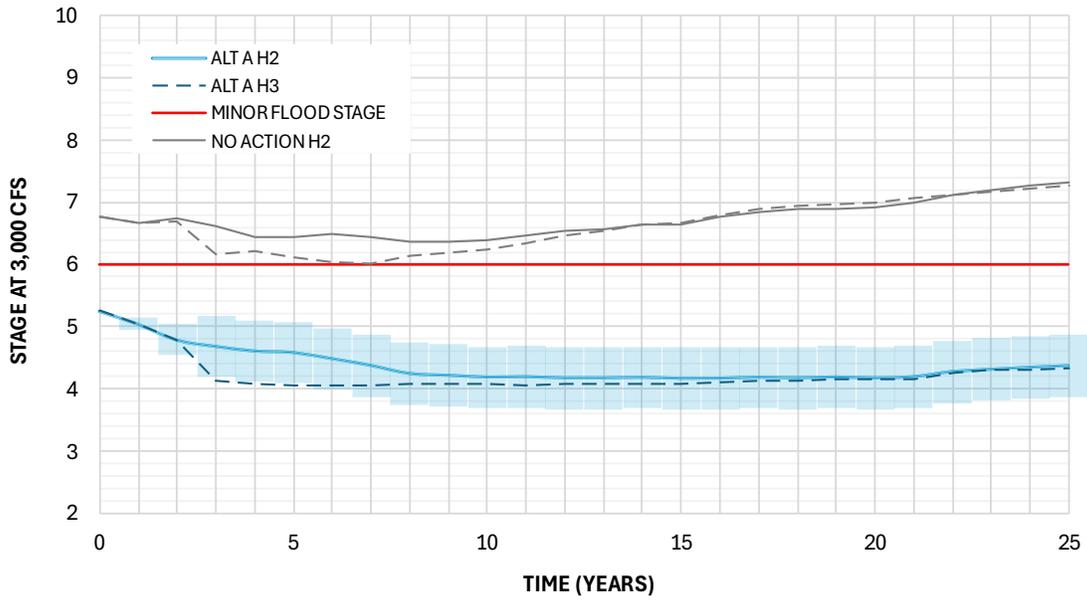
Figure 5-7 Alt A and No Action H2 and H3 25-Year Forecast - Stage at 3,000 cfs through Time
