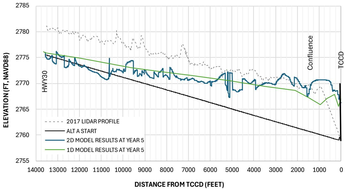
Figure 5-10 Comparison of Alt A 1D and 2D Sediment Model Results – Channel Profile at Start and Year 5.
