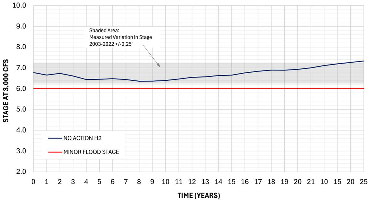
Figure A-7 Stage at HWY83 at 3,000 cfs through Time – No Action H2
