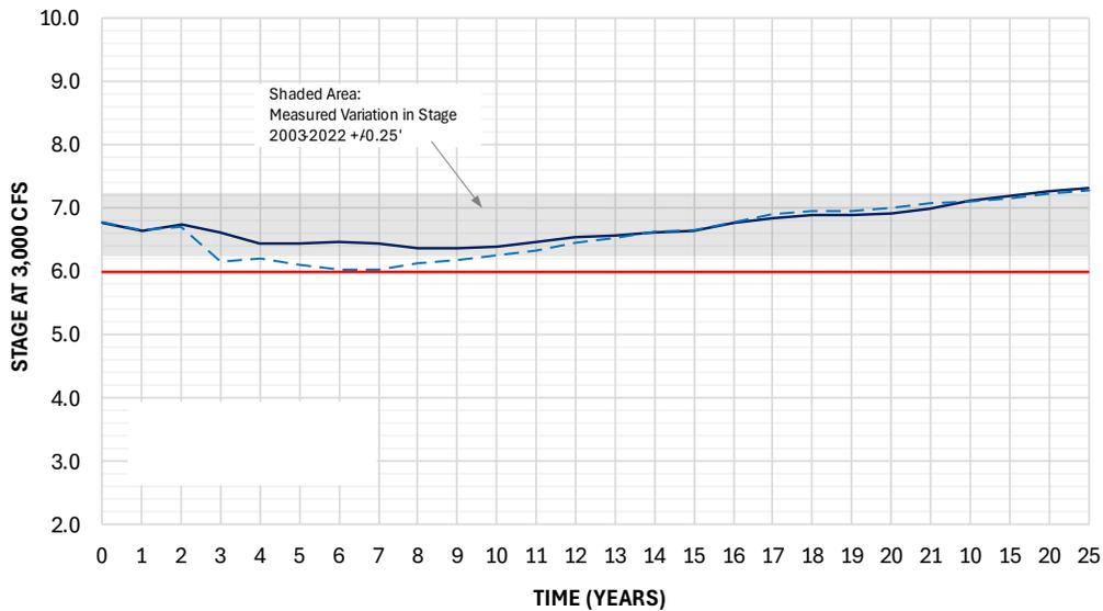
Figure 4-5 No-Action H2 and H3 25-Year Forecast - Stage at 3,000 cfs through Time
