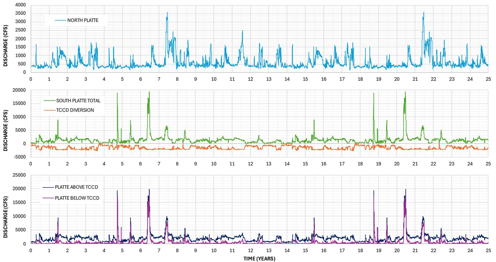
**Figure 3-8 25-Year Hydrograph for Sediment Transport Modeling – H1 Hydrograph**
