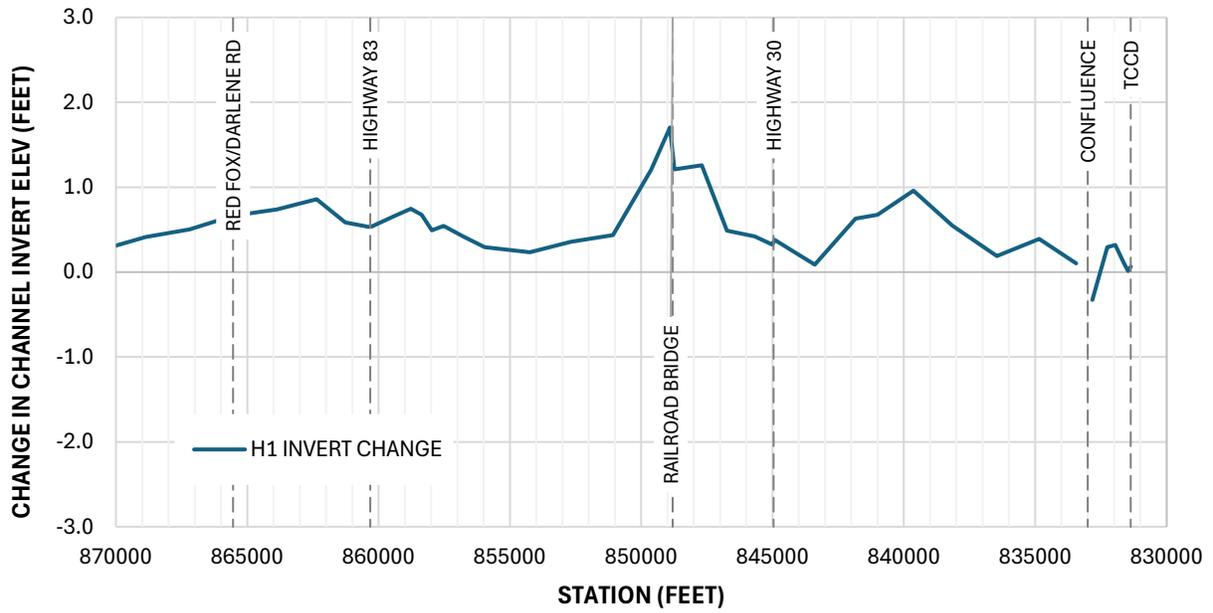
**Figure A-5 Change in Channel Invert Elevation – No Action H1**
