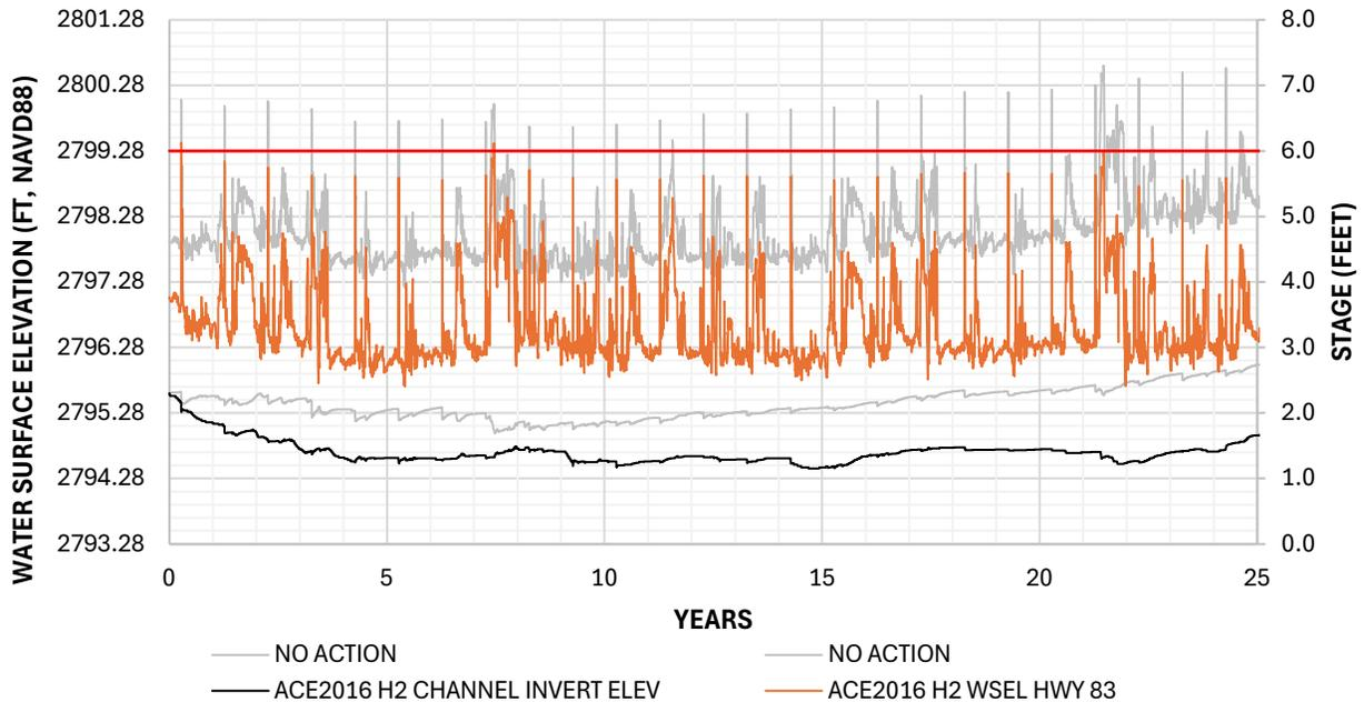
**Figure F-1 Water Surface and Channel Elevation at HWY 83 – No Action and ACE2016 Alt H2**
