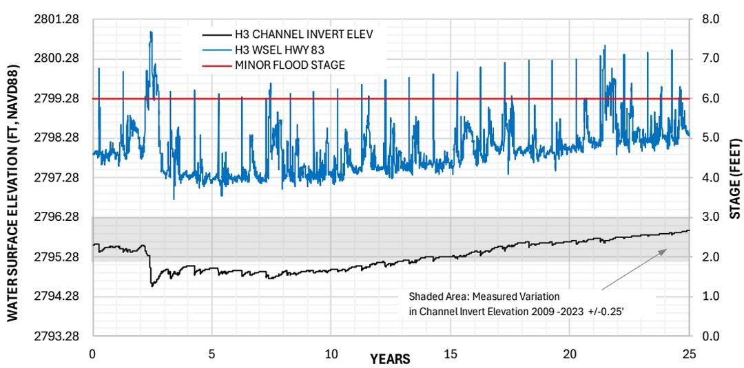
**Figure 4-3 No-Action 25-Year Forecast for - Water Surface and Channel Elevation at HWY 83
