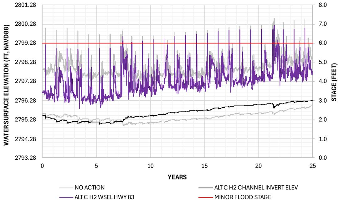
**Figure 5-18 Alt C 25-Year Forecast - Water Surface and Channel Elevation at HWY 83**
