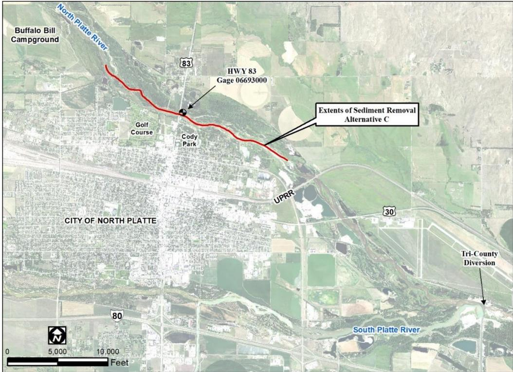
Figure 5-16 Extents of Sediment Removal Alternative C
