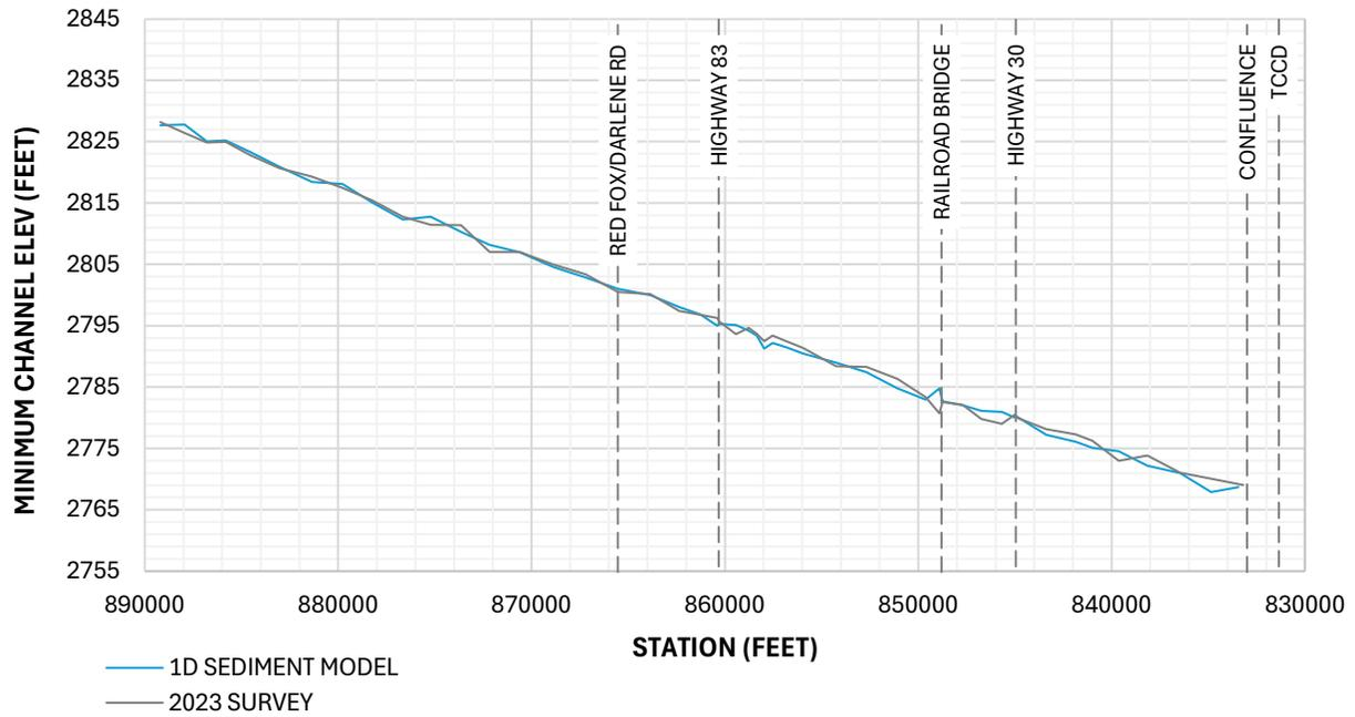
**Figure 11 Channel Profile Comparison – Calibration Model vs 2023 Survey using Yang**
