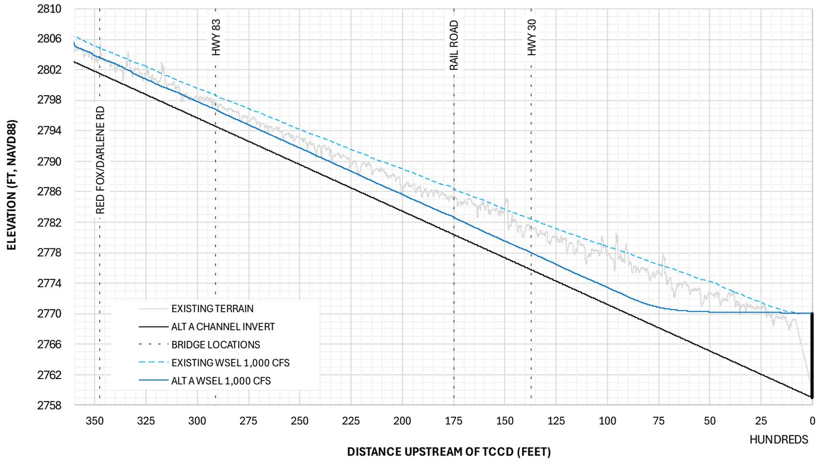
Figure 2 Existing and Sediment Removal Alt A Water Surface Profile 1,000 cfs
