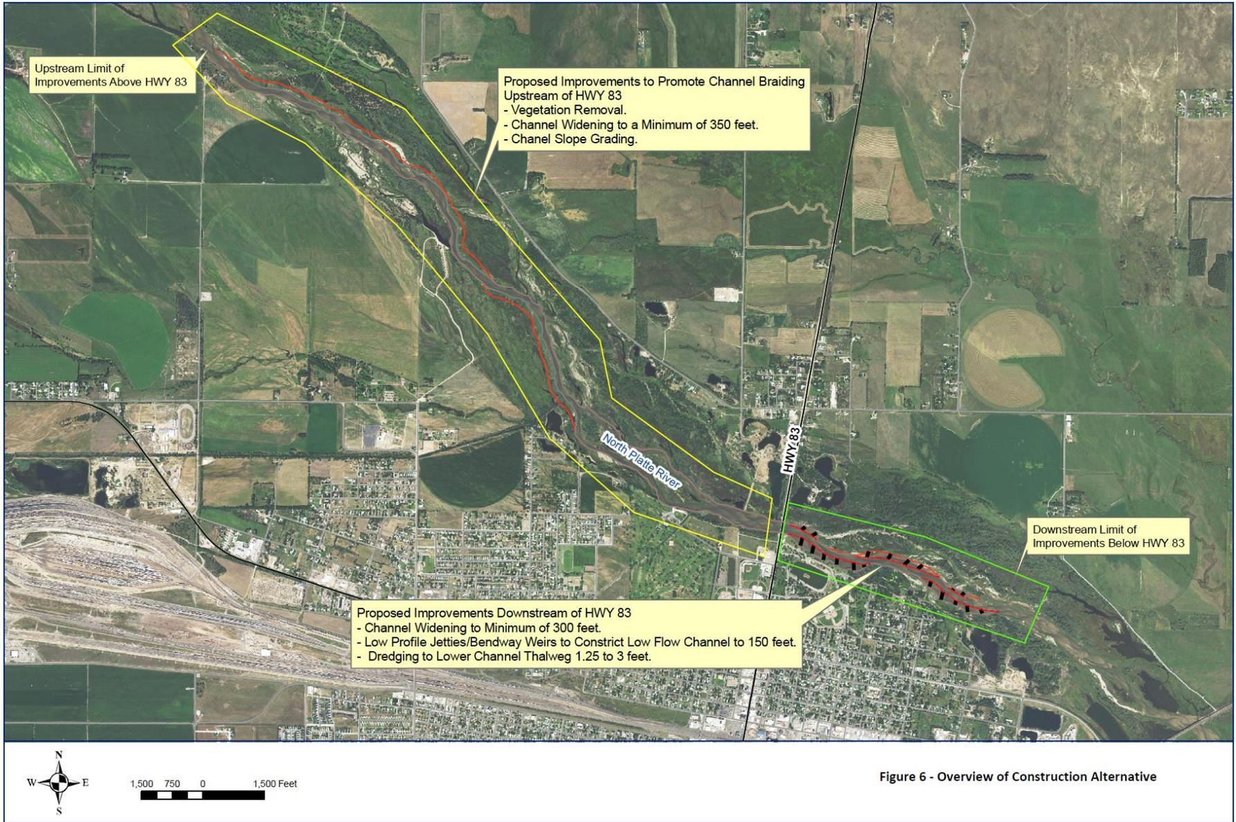
Figure 6 - Overview of Construction Alternative
