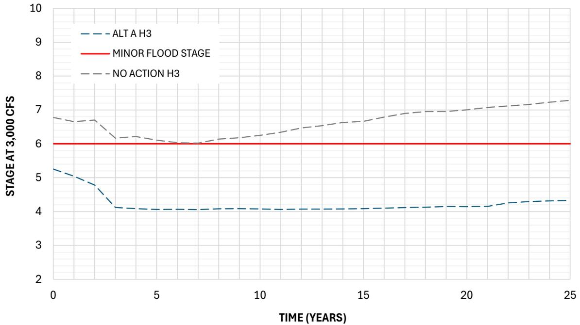
Figure B-14 Stage at HWY83 at 3,000 cfs through Time – No Action and Alt A H3
