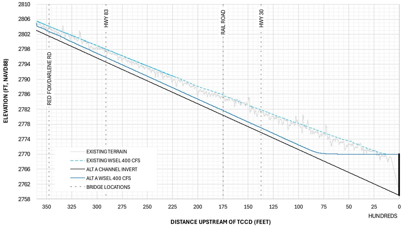
**Figure 1 Existing and Sediment Removal Alt A Water Surface Profile 400 cfs (Baseflow)**
