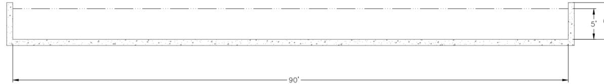
**RECTANGULAR CONCRETE CANAL SECTION - 1,500 CFS CAPACITY**
