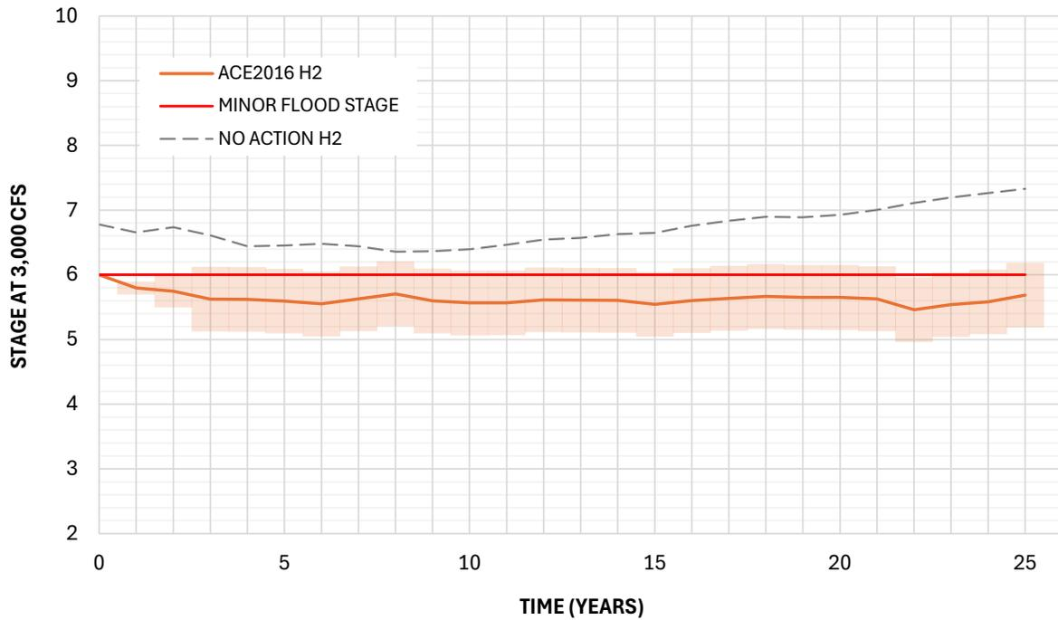
Figure F-2 Stage at HWY83 at 3,000 cfs through Time – No Action and ACE2016 Alt H2
