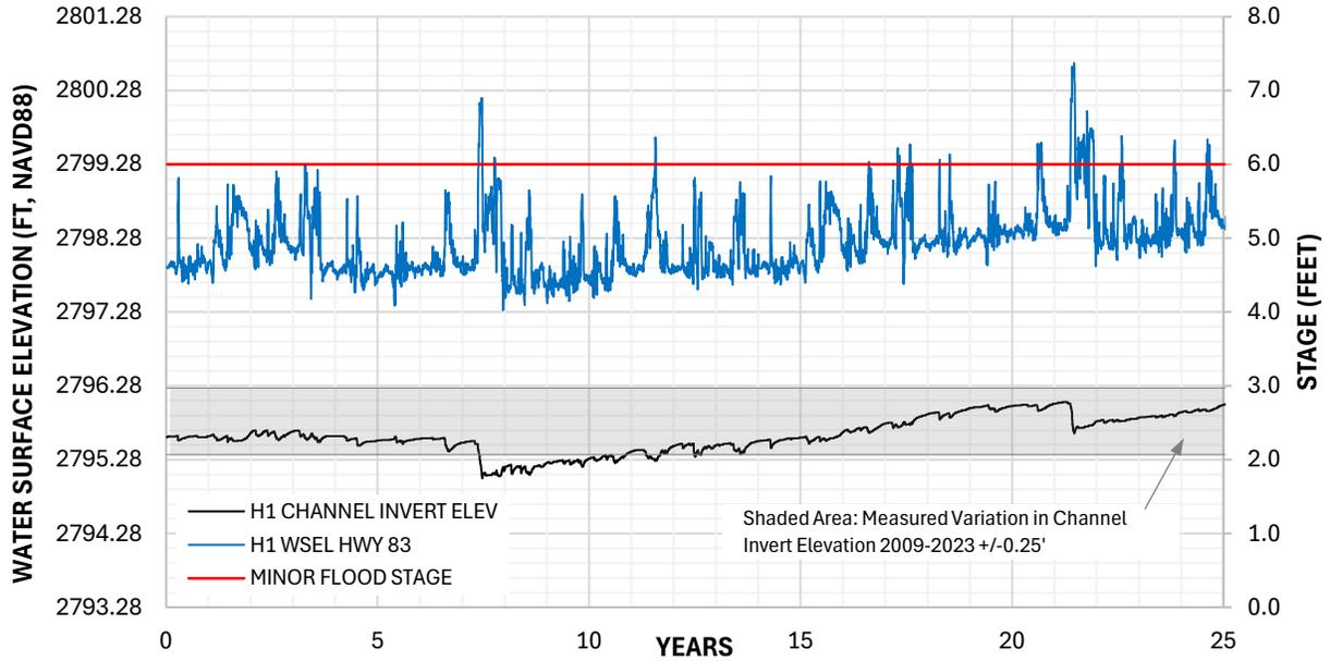
Figure A-3 Water Surface and Channel Elevation at HWY 83 – No Action H1
