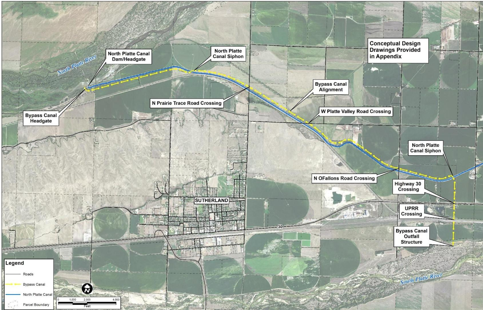
Figure 7-1 Bypass Canal Alignment
