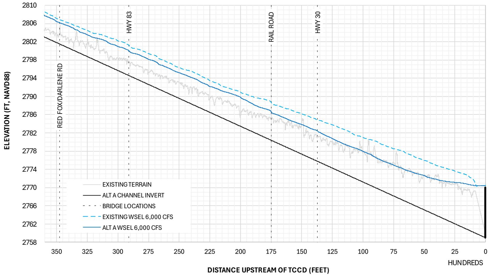
**Figure 4 Existing and Sediment Removal Alt A Water Surface Profile 6,000 cfs**
