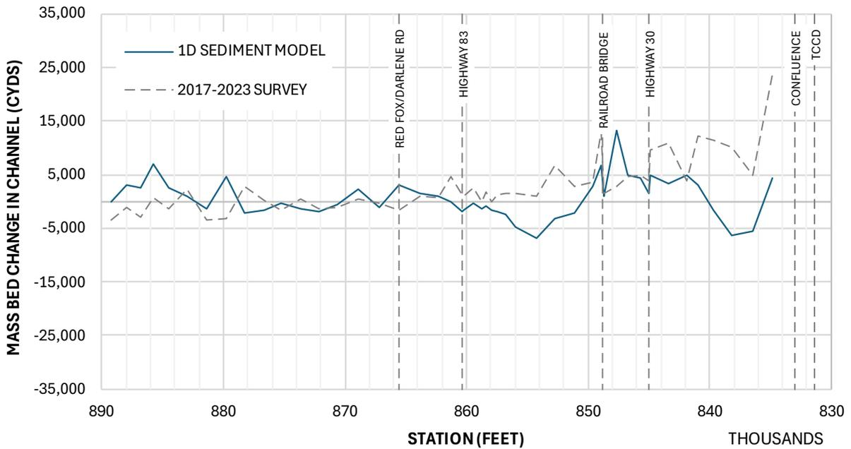
Figure 3-7 Mass Bed Change in Channel – Model vs Survey Data
