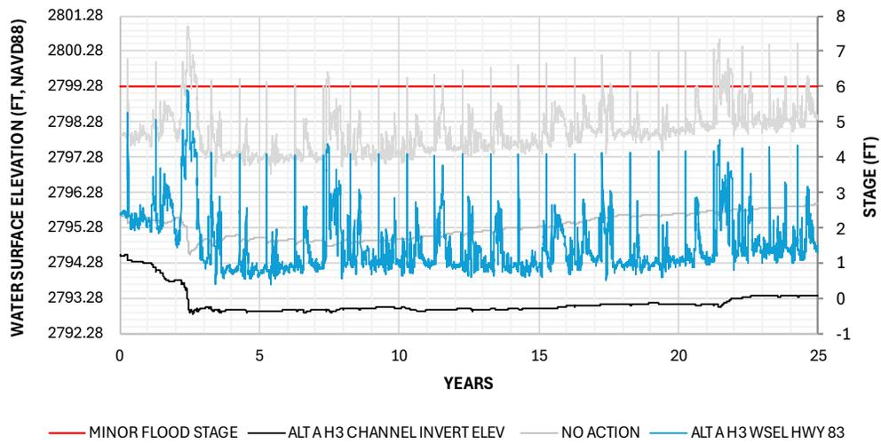
**Figure 5-4 Alt A 25-Year Forecast - Water Surface and Channel Elevation at HWY 83**
