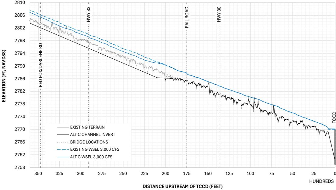
Figure 5-17 3,000 cfs Water Surface Profile - Existing Condition and Alt C
