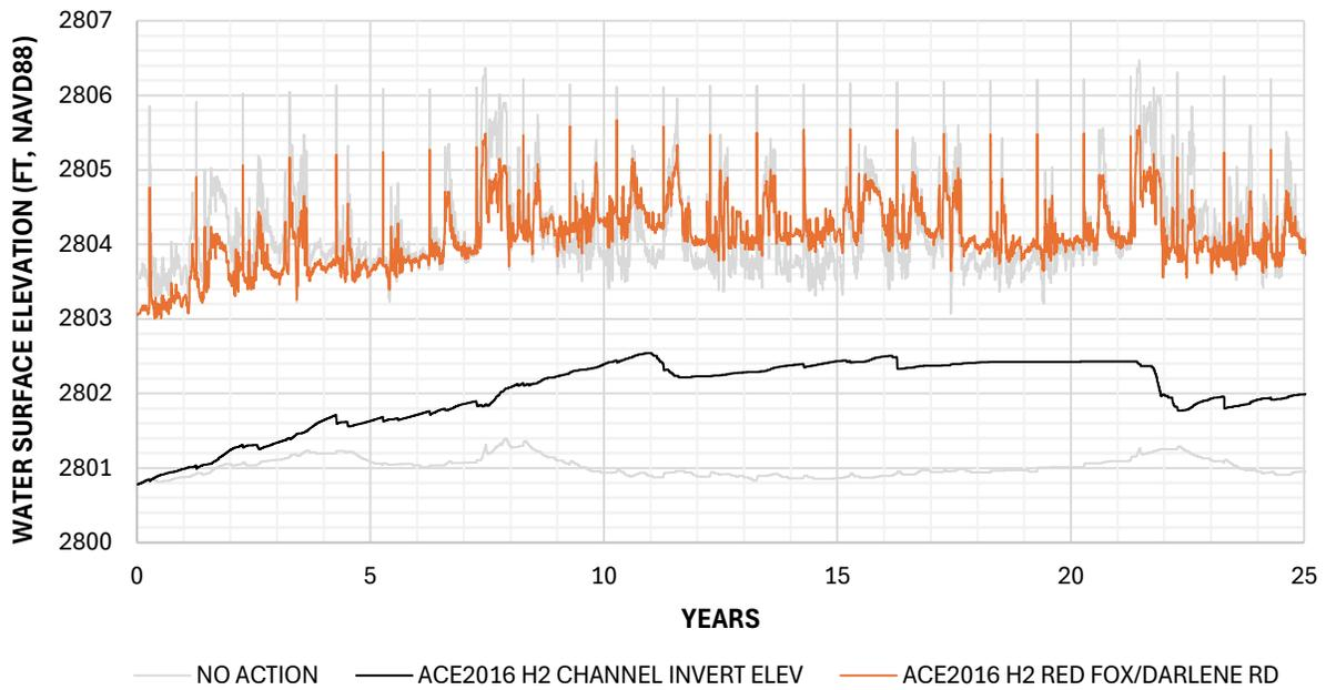
Figure F-3 Water Surface and Channel Elevation at Red Fox/Darlene Rd – No Action and ACE2016 Alt H2
