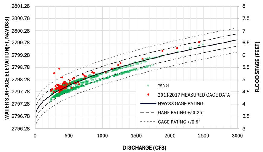
**Figure 9 Stage Discharge Rating Curves at HWY 83 Gage – 1D Sediment Transport Model Results 2017-2023 using 4 Transport Equations**
