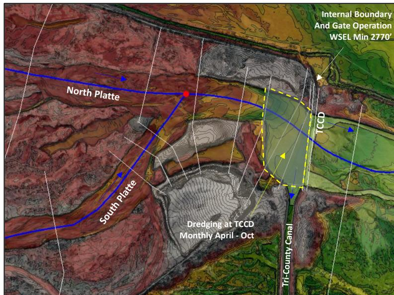
Figure 3-2 Area of Model Dredging at TCCD
