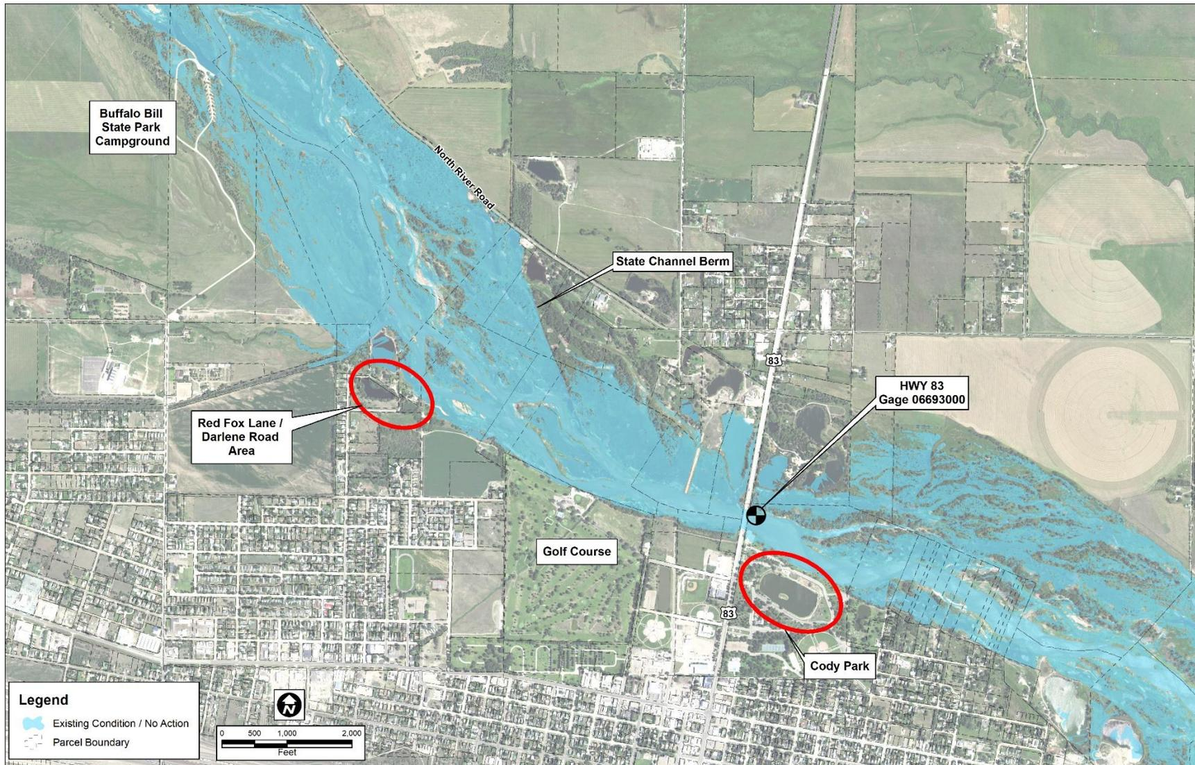
Figure 4-1 North Platte Chokepoint Existing Conditions/No-Action - Inundation Mapping at 3,000 cfs
