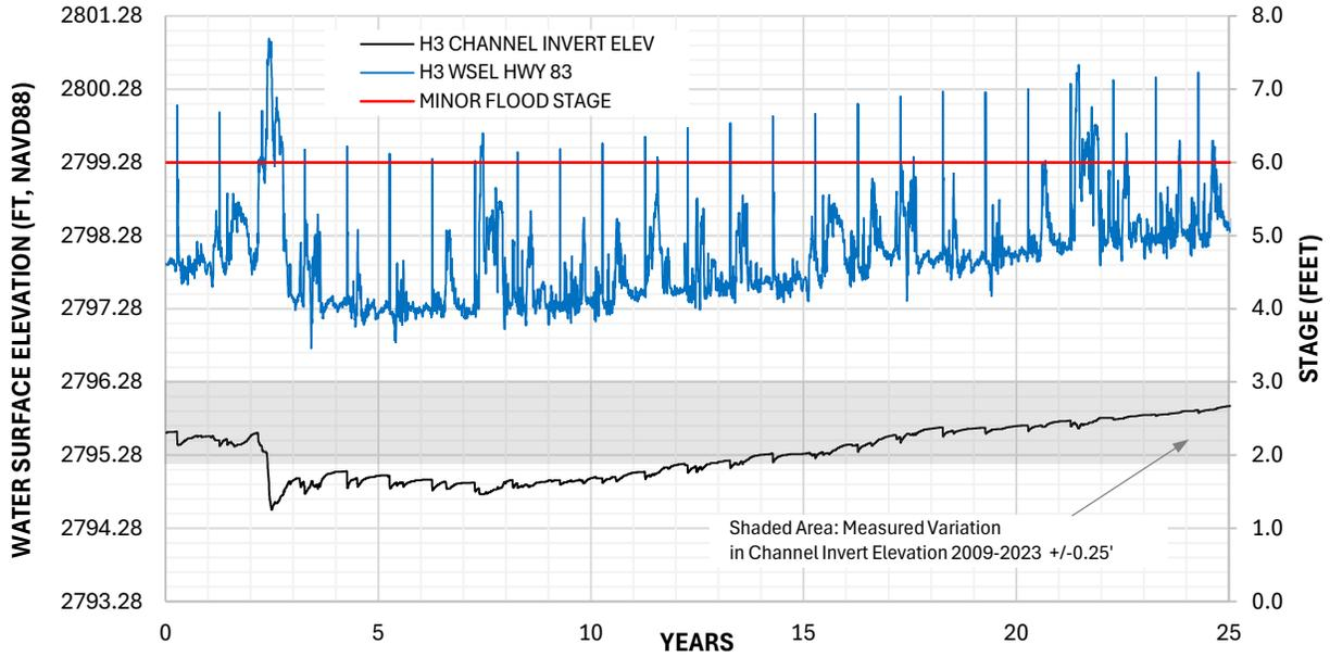
Figure A-10 Water Surface and Channel Elevation at HWY 83 – No Action H3
