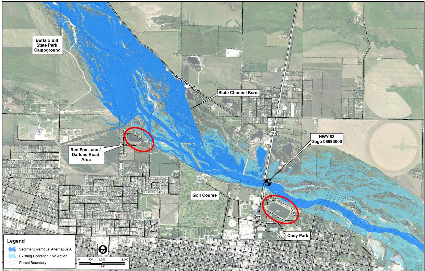
Figure 5-3 North Platte Chokepoint Inundation Mapping at 3,000 cfs – Existing Conditions/No Action and Alt A
