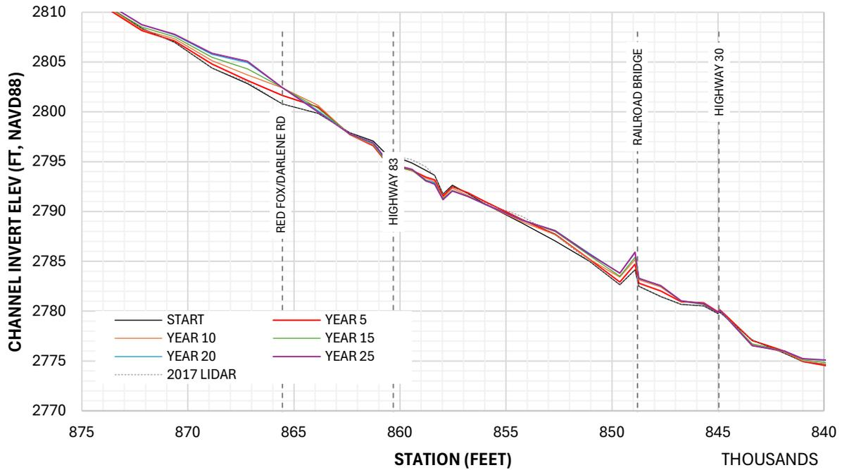
Figure F-5 Channel Profile through Time – ACE2016 Alt H2
