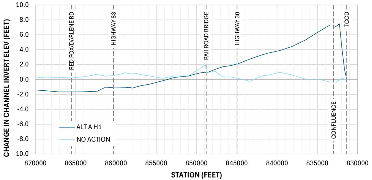
Figure B-6 Change in Channel Invert Elevation – No Action and Alt A H1
