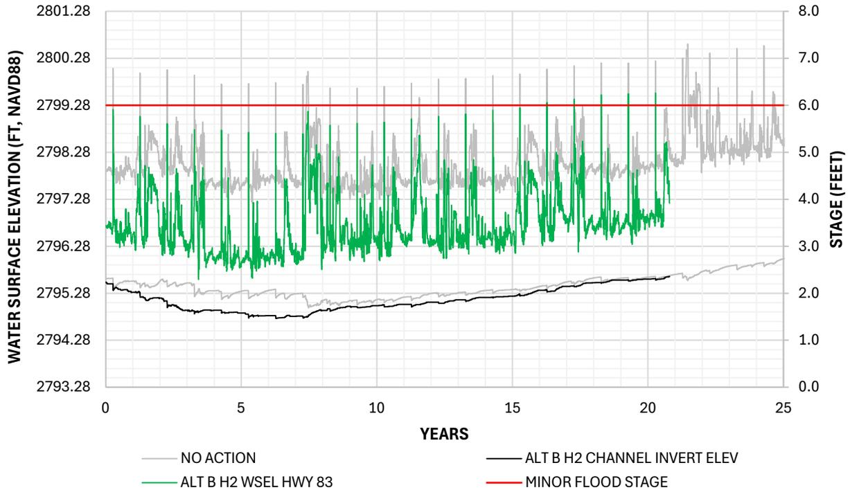
Figure C-3 Water Surface and Channel Elevation at HWY 83 – No Action and Alt B H2
