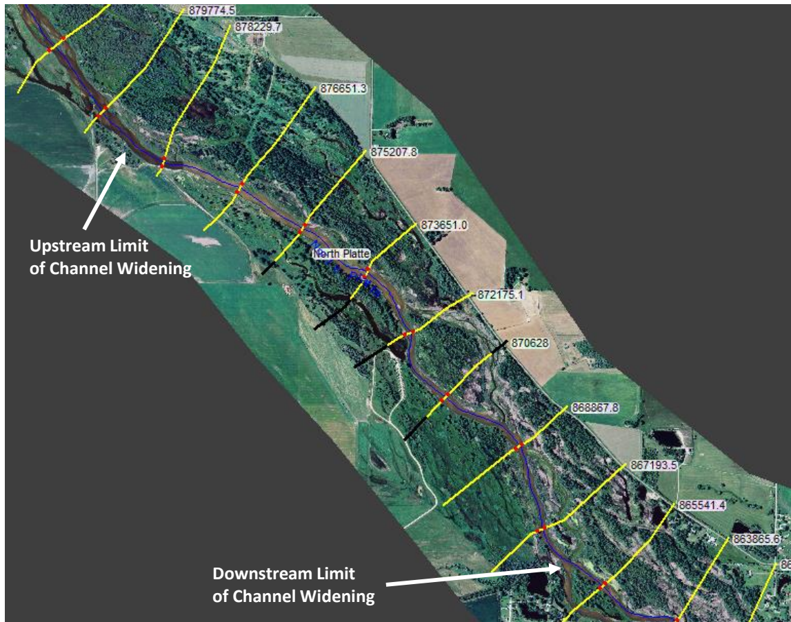
Figure 6. Limits of Channel Widening upstream of Highway 83. Channel would be widened to 350 feet.
