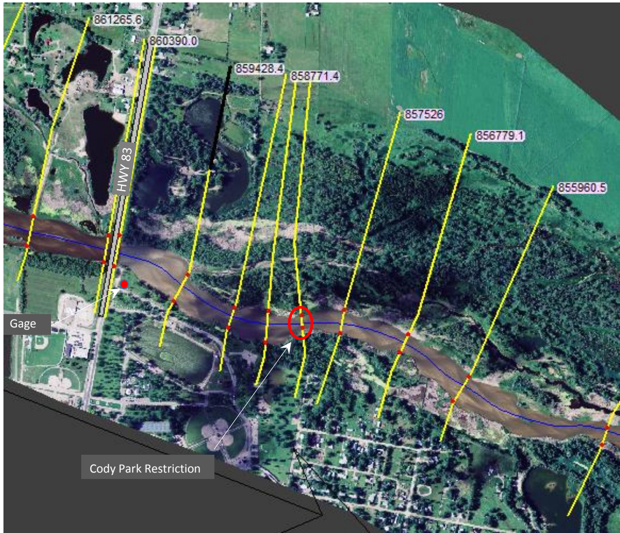
Figure B-4 Choke Point SIAM Reach 4 – HWY 83 to Cody Park Restriction, Station 860268 – 856779
