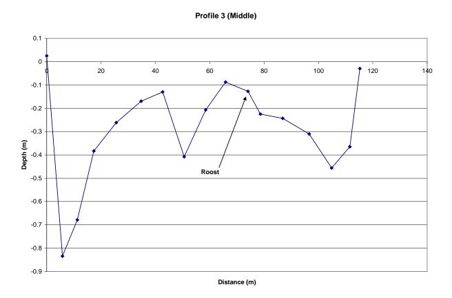
Figure 9. Roost channel profile for Use Site 2 (left to right bank).
