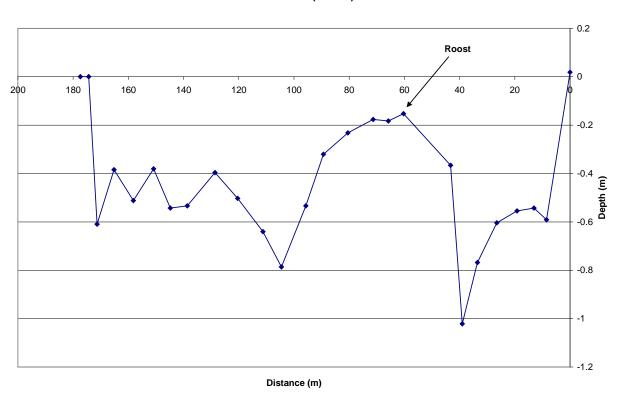
Figure 10. Roost channel profile for Use Site 3 (left to right bank).
