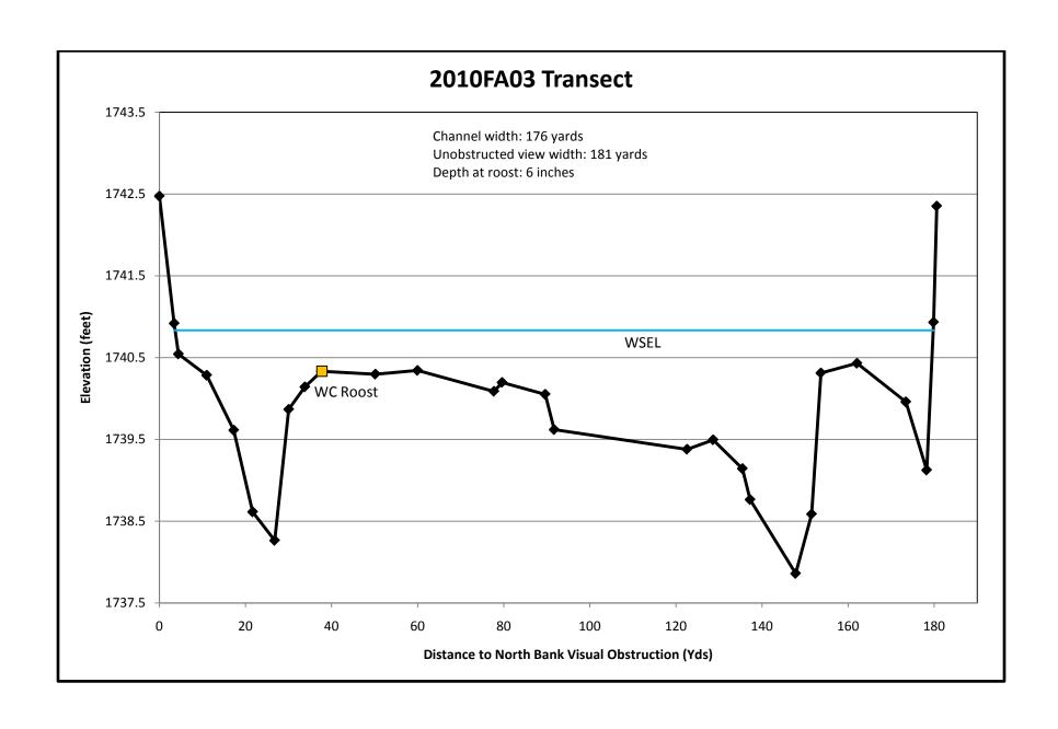
Figure 8. Roost channel profile for Use Site 1 (left to right bank).
