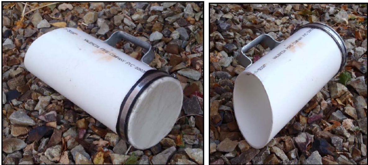
Figure 5. Pipe dredge used to collect bed-material samples for the reach-wide geomorphic and vegetation monitoring project (Ayres and Olsson, 2010).
