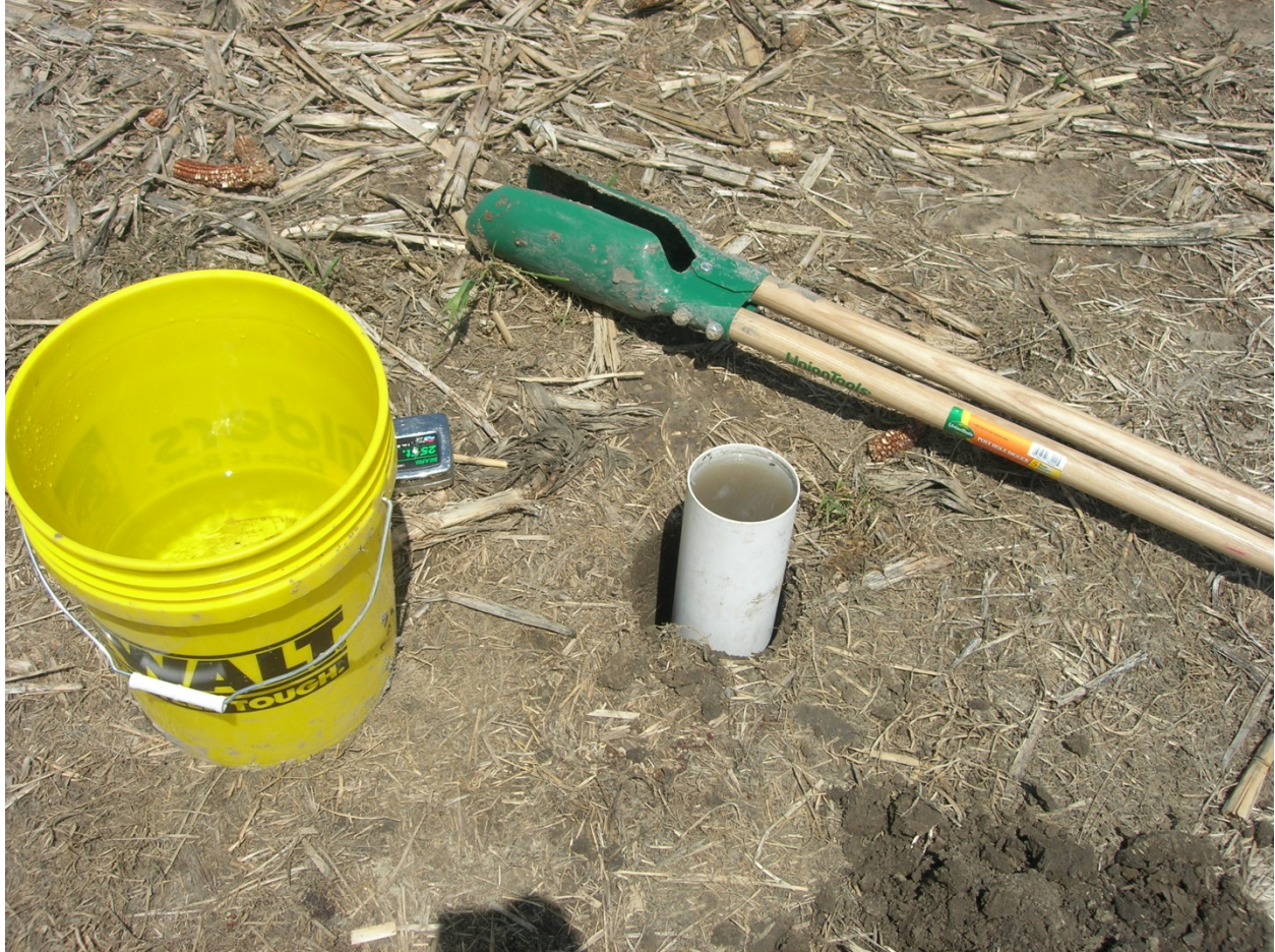
Phelps 9.7 Single-Ring Infiltrometer Percolation Test with 4" PVC (Phelps 9.7)
