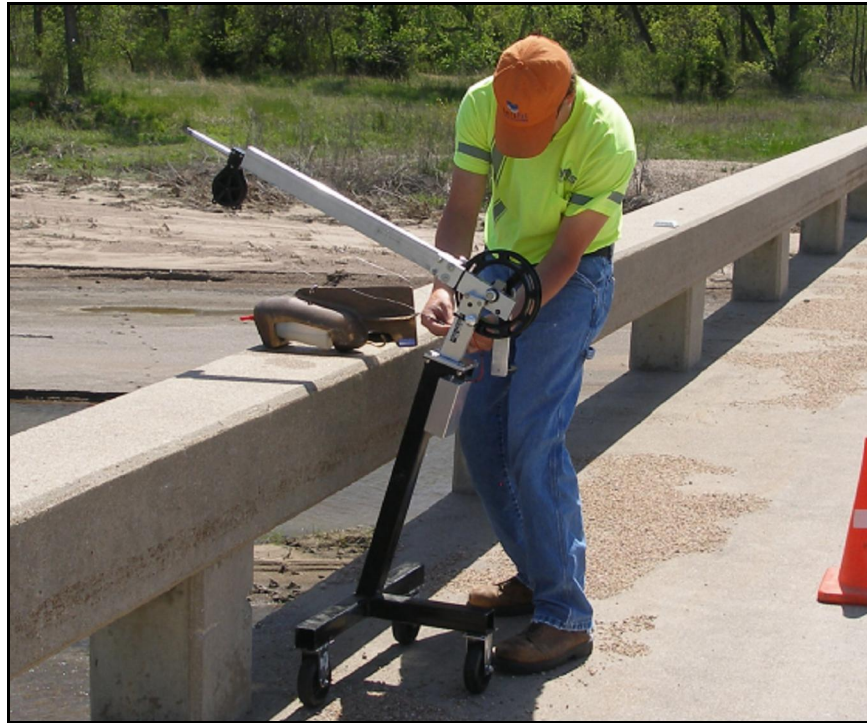
Figure 6.1. View of DH-40 suspended by cable from hand winch mounted on a portable, lightweight, wheeled frame.
