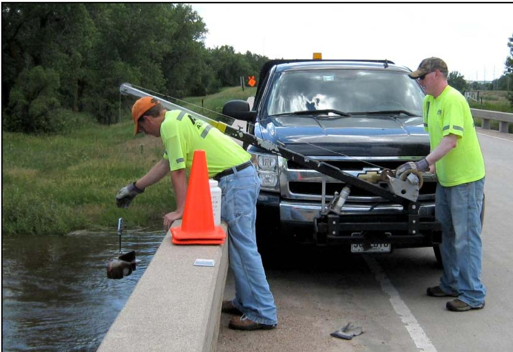
Figure 5.2. View of US DH-76 suspended sediment sampler cable suspended with a B-56 sounding reel on a truck-mounted crane system.
