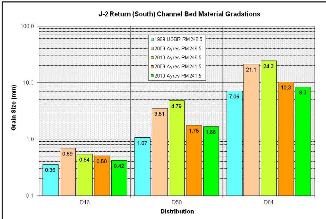
Figure 4.5. Comparison of grain size distribution for the USBR 1989 USBR, Ayres 2009, and Ayres 2010 composite bed material samples at river miles 246.5 and 241.5 on the J-2 Return (South) channel.
