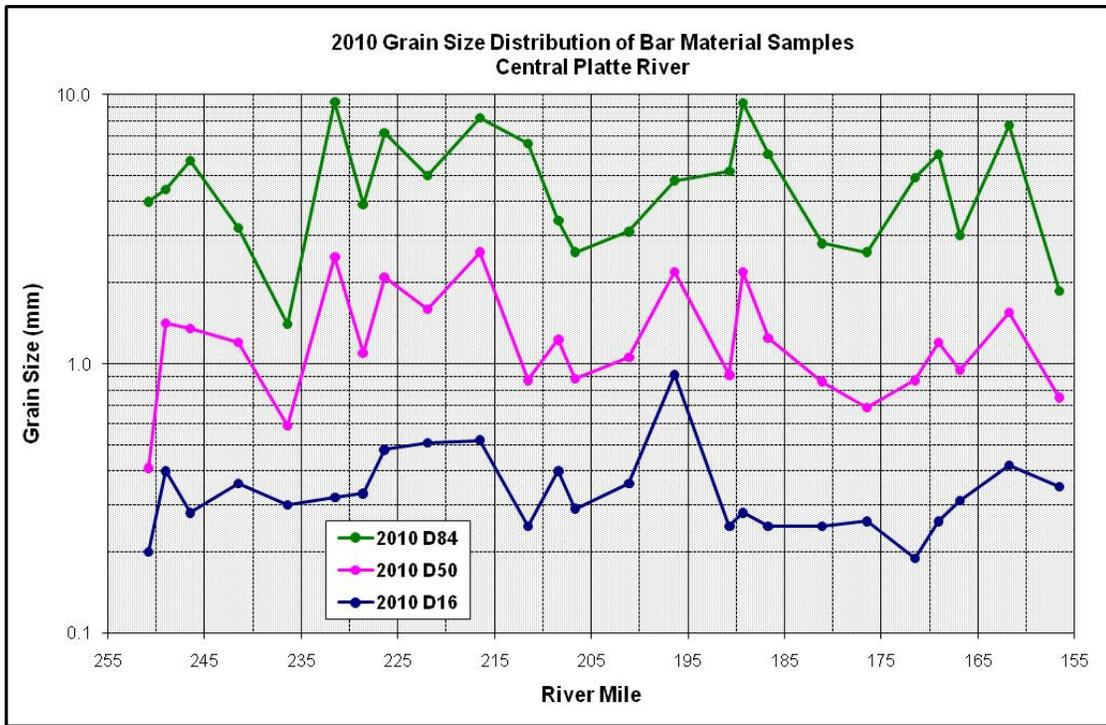
Figure 4.2. Grain size distribution of 2010 composite bar samples by river mile.
