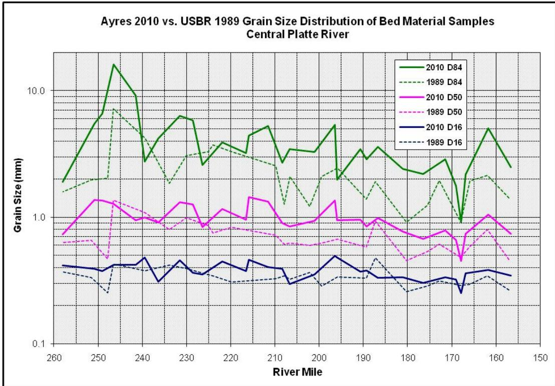
Figure 4.4. Comparison of the grain size distributions of the 2010 bed samples with the 1989 USBR bed samples by river mile.
