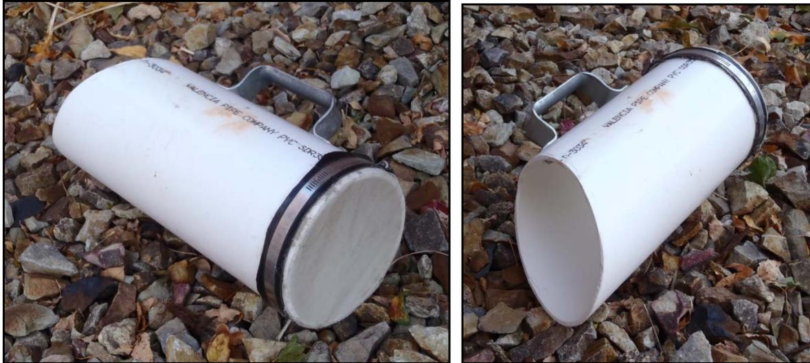
Figure 4.1. Pipe dredge used to collect bed material samples.
