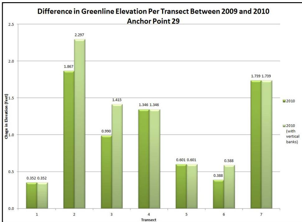
Figure 3.12. Change in 2010 compared to 2009 green line elevations at AP-29. Darker bars exclude vertical bank green lines and lighter bars include them.
