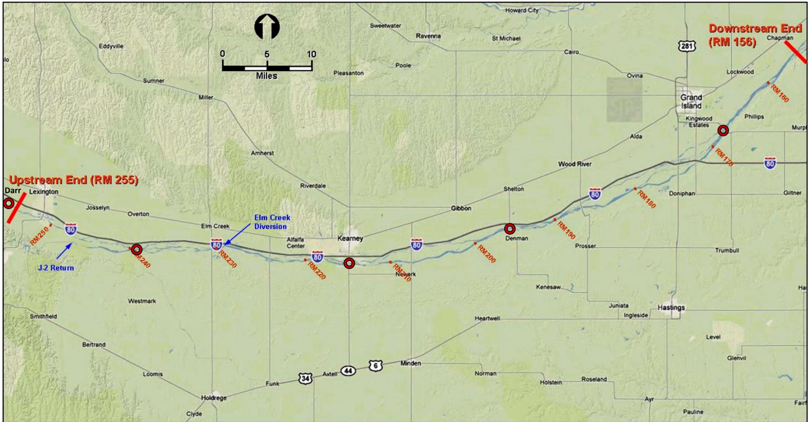
Figure 2.1. Location map showing the project reach for the Channel Geomorphology and In-Channel Vegetation Monitoring. Bedload and suspended sediment sampling bridge sites are shown as red circles.
