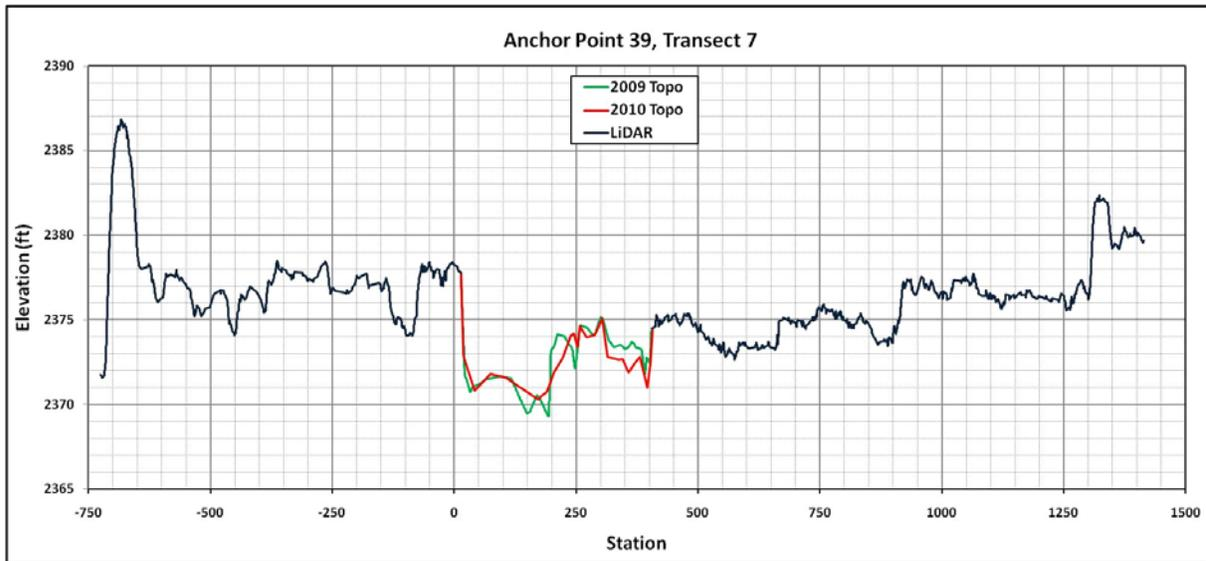
Figure 3.2. View looking downstream of typical cross section (exaggerated scale) compiled from 2009 and 2010 transect survey and 2009 LiDAR data.
