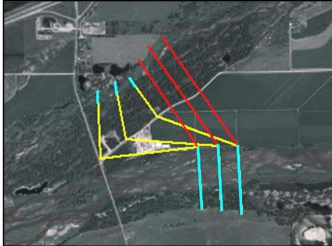
Figure 3.3. View of cross section at anchor point AP13 showing the previous LiDAR alignment (red) and the revised LiDAR alignment (yellow). The transect survey data is shown in blue.
