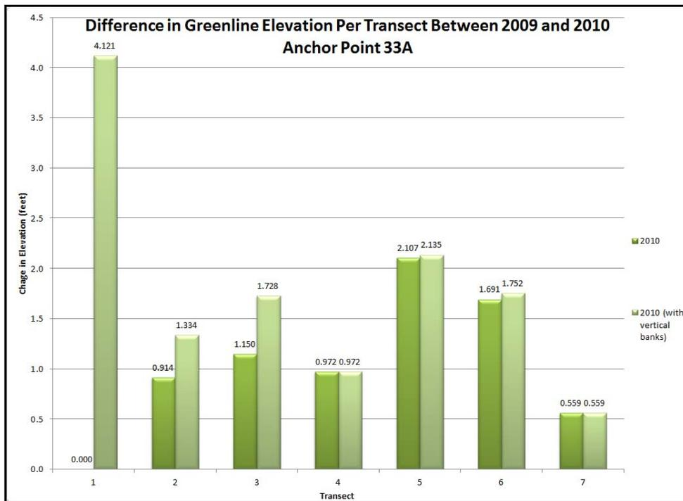
Figure 3.13. Change in 2010 compared to 2009 green line elevations at AP-33a. Darker bars exclude vertical bank green lines and lighter bars include them.
