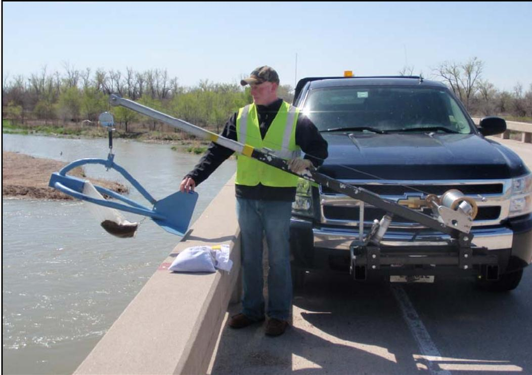
Figure 5.1. View of BL-84 Helley-Smith bedload sampler cable suspended with a B-56 sounding reel on a truck-mounted crane system.
