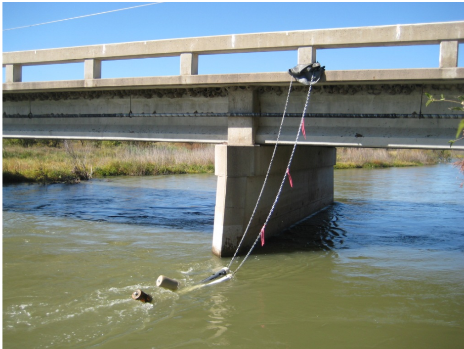
13. MS-5 and YSI 6920 side by side deployment
