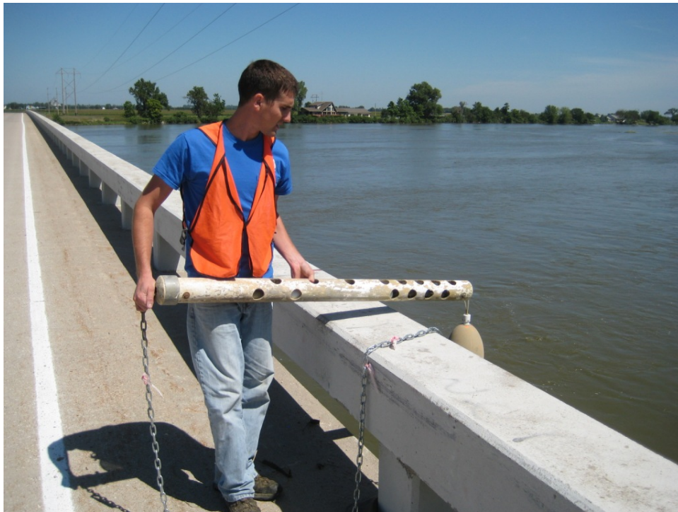
5. MS-5 deployment on Hwy 287 Avenue bridge near Duncan, NE.
