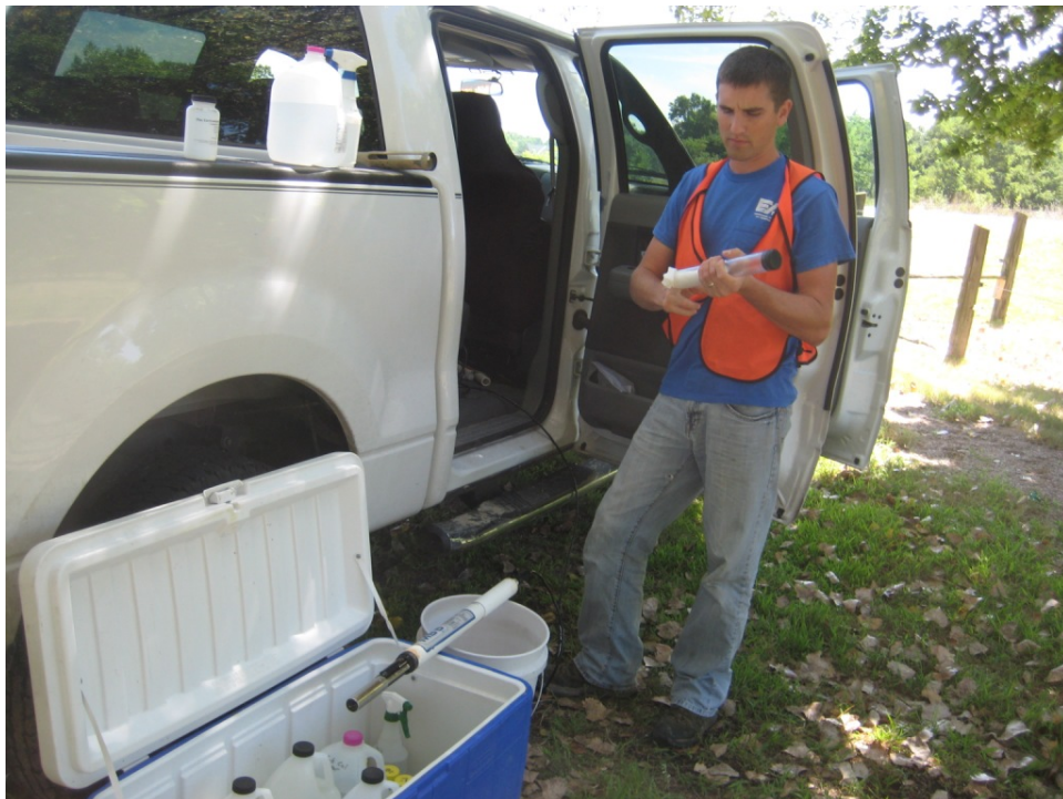
4. MS-5 calibration of standards (pH, specific conductance, turbidity, dissolved oxygen).
