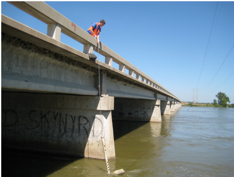
6. MS-5 deployment into the Platte River near Duncan, NE.
