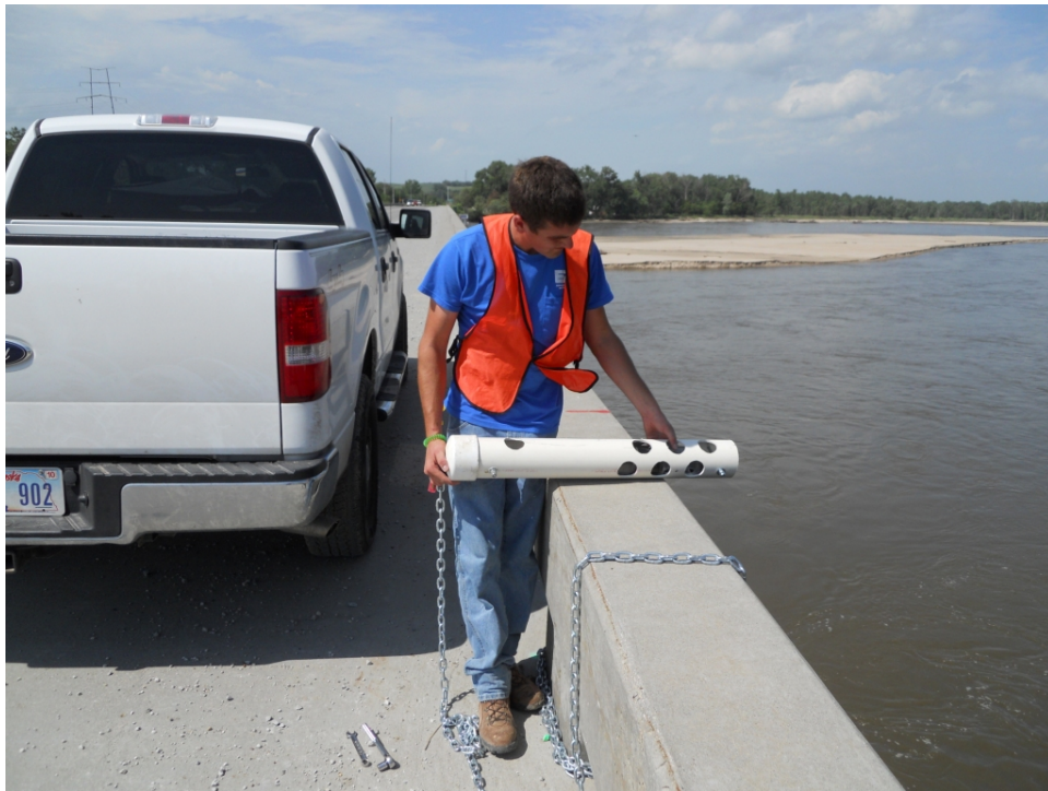
3. Manta 2 deployment on Hwy 50 bridge near Louisville, NE.
