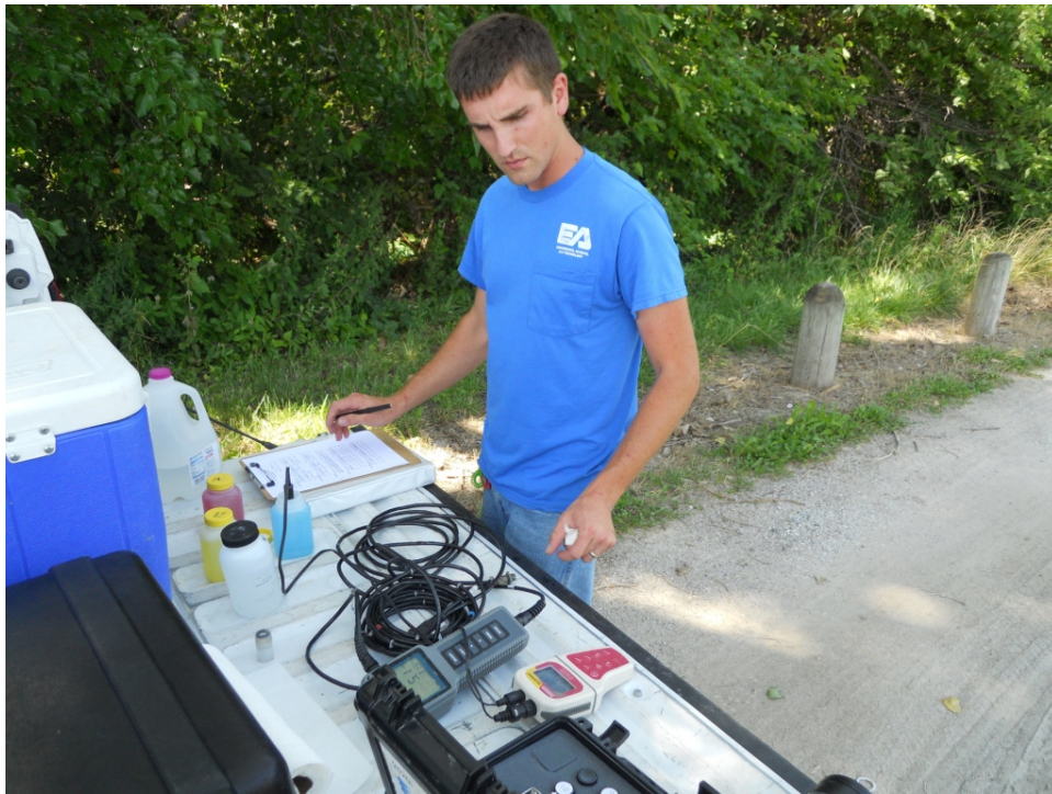
1. Hand held water quality instrument calibration (YSI 85, Oakton 300, LaMotte 2020e).
