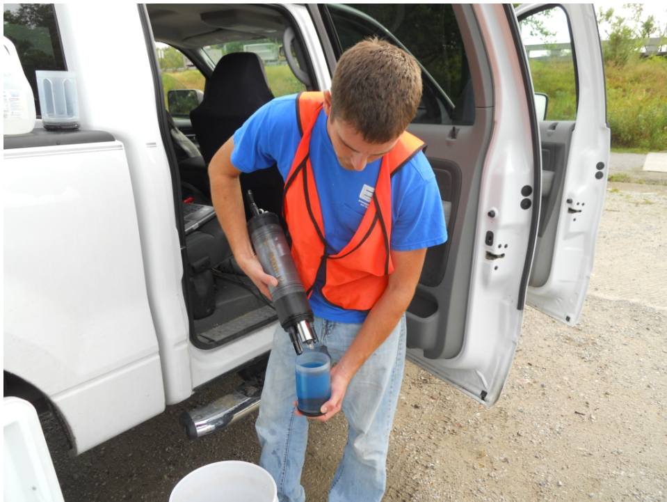
2. Manta 2 calibration of standards (pH, specific conductance, turbidity, dissolved oxygen).
