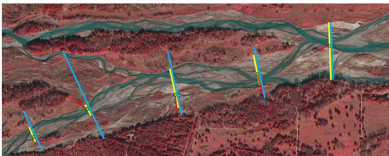
Figure 2. Example of how Unobstructed Channel Width (UOCW; yellow lines), Nearest Forest (NF; red lines) and Unforested Channel Width (UFCW; blue lines) were measured at whooping crane use and available locations.
