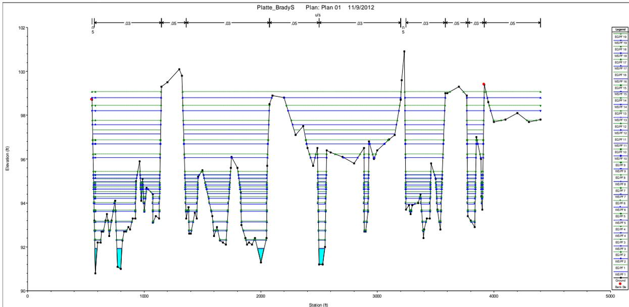
Figure 3.17 Platte at Brady, cross-section with water surface and EGL at flows from 100 to 50,000 cfs
