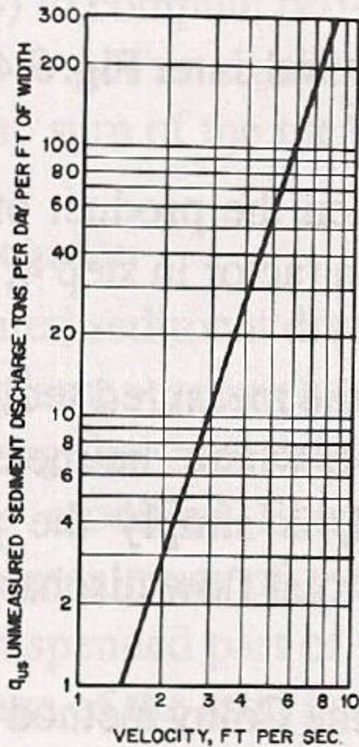
**Fig. 9.45** Relationship between unmeasured sediment discharge and mean velocity (after Colby, 1957).
