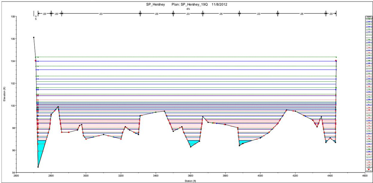
Figure 3.13 South Platte at Hershey, cross-section with water surface and EGL at flows from 100 to 50,000 cfs
