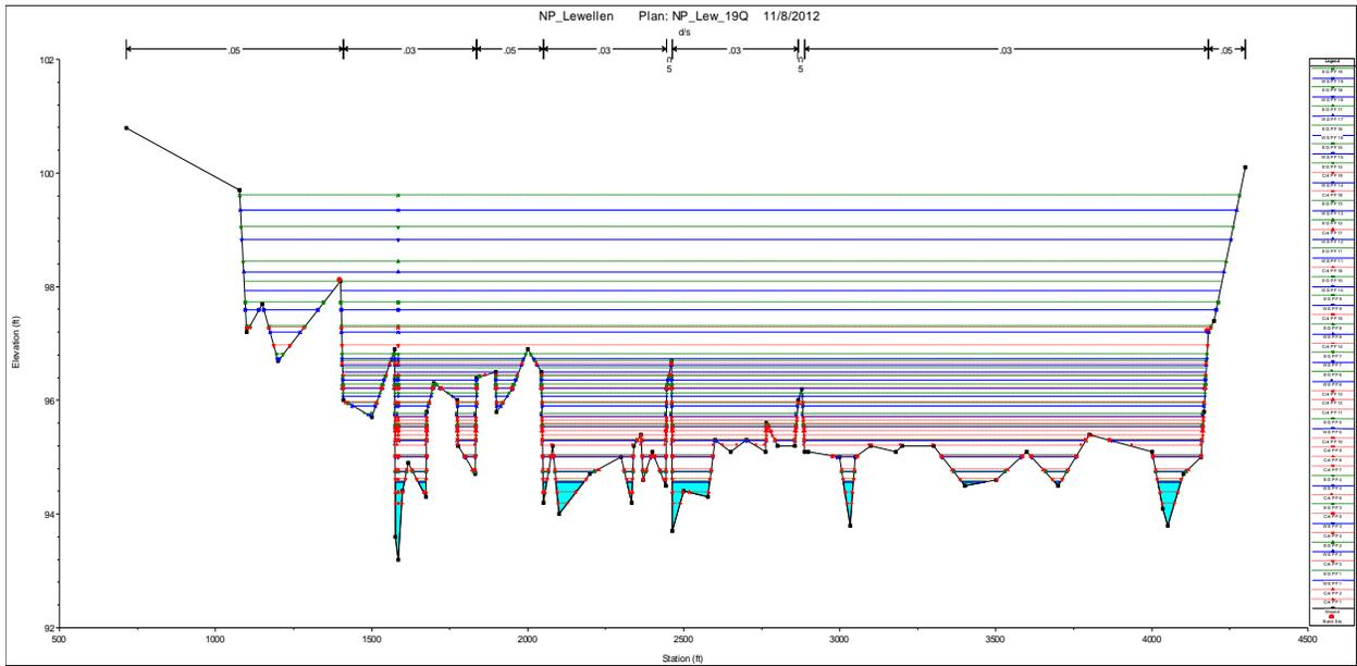
Figure 3.1 North Platte at Lewellen, cross-section with water surface and EGL at flows from 100 to 50,000 cfs
