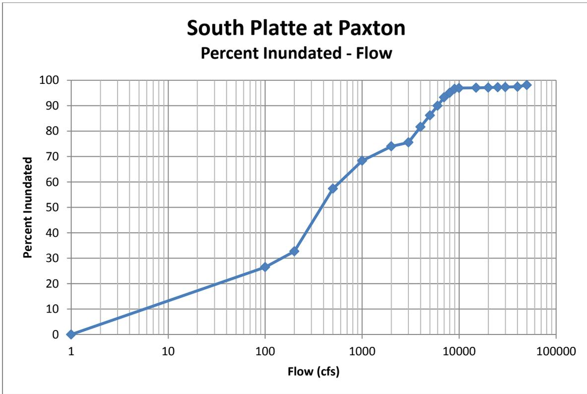
Figure 3.11 South Platte at Paxton, percent inundated – flow
