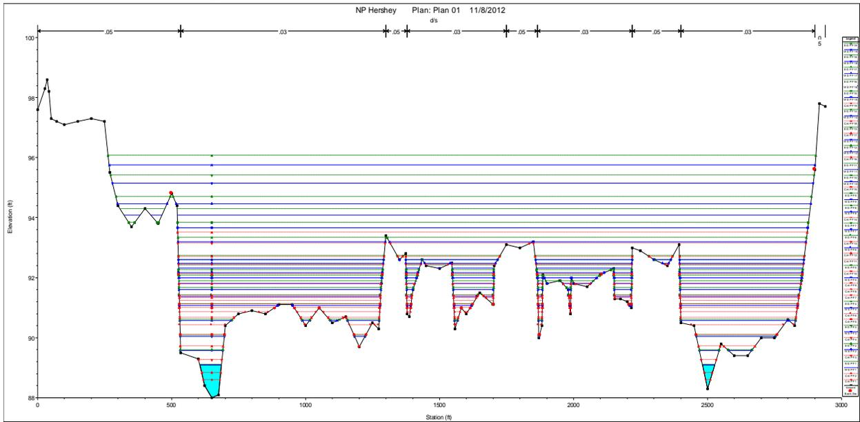
Figure 3.5 North Platte at Hershey, cross-section with water surface and EGL at flows from 100 to 50,000 cfs
