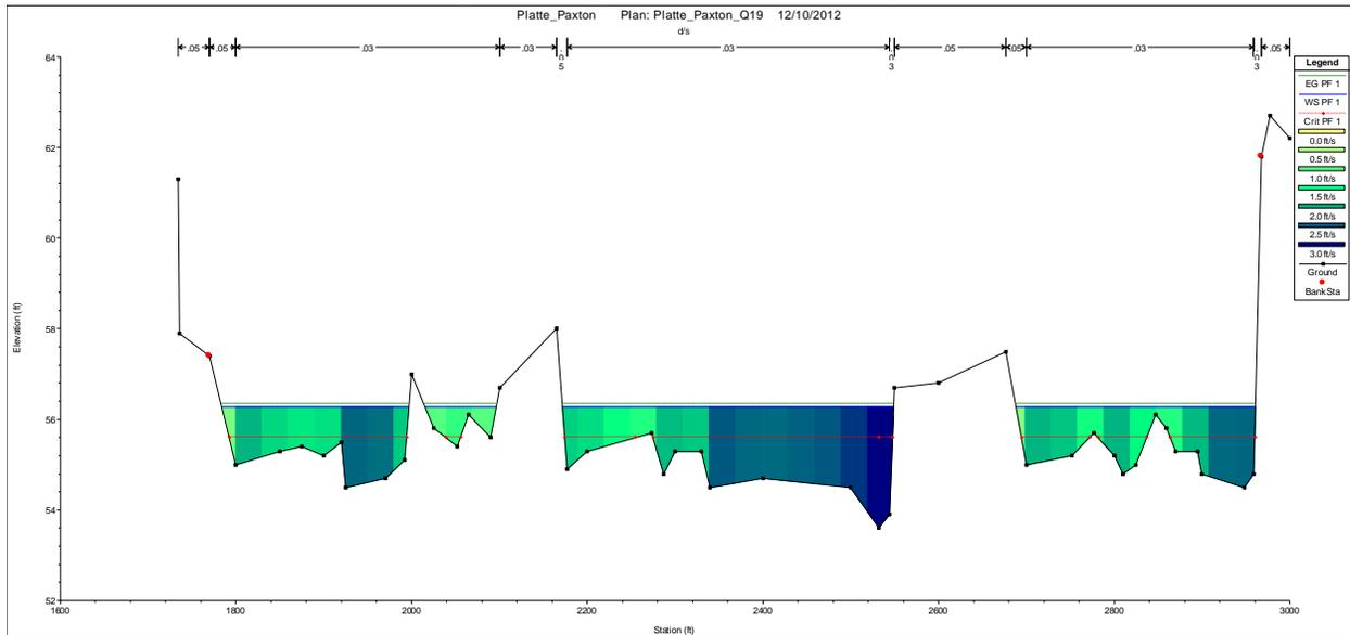
Figure 3.27 South Platte at Paxton – flow distribution
