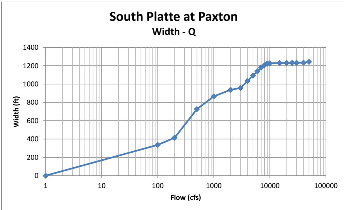
Figure 3.12 South Platte at Paxton, width - flow
