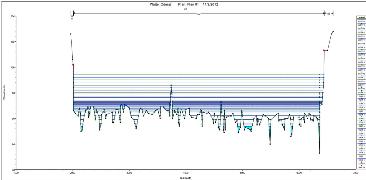
Figure 3.21 Platte at Odessa, cross-section with water surface and EGL at flows from 100 to 50,000 cfs
