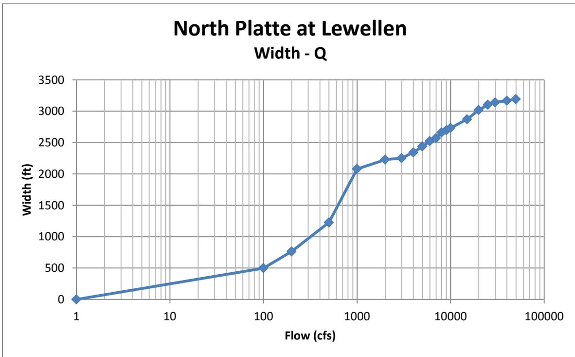
Figure 3.4 North Platte at Lewellen, width - flow
