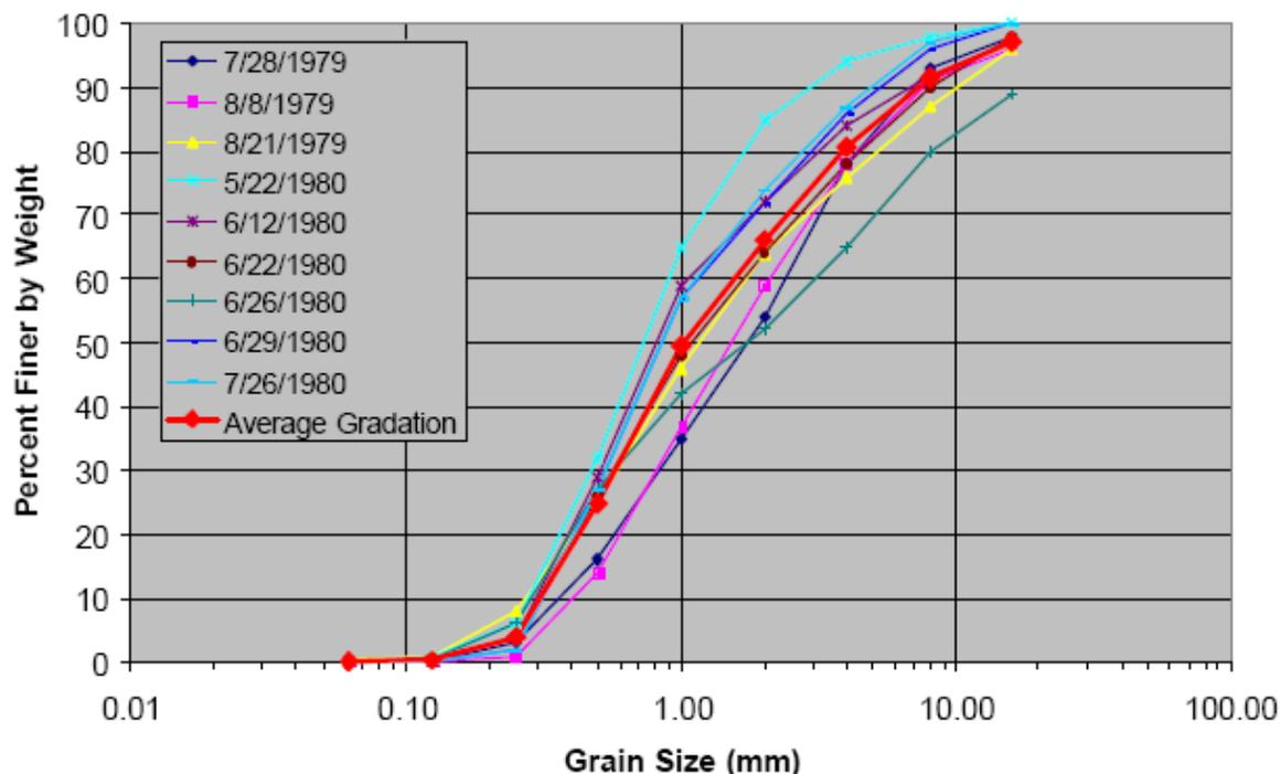
Figure 3.16 Bed Material Grain Size Distributions of the South Platte River at North Platte, Nebraska in 1979-1980.
