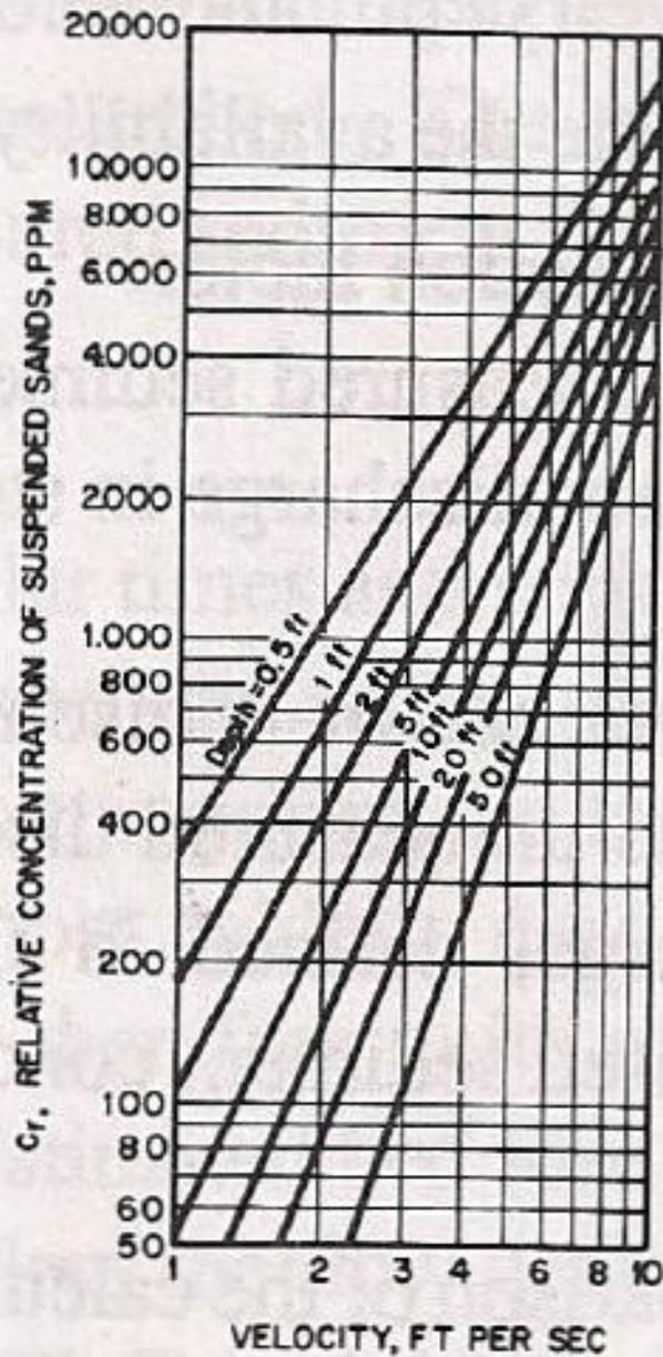
**Fig. 9.46** Relative concentrations of suspended sands for different depths and mean velocity (after Colby, 1957).
