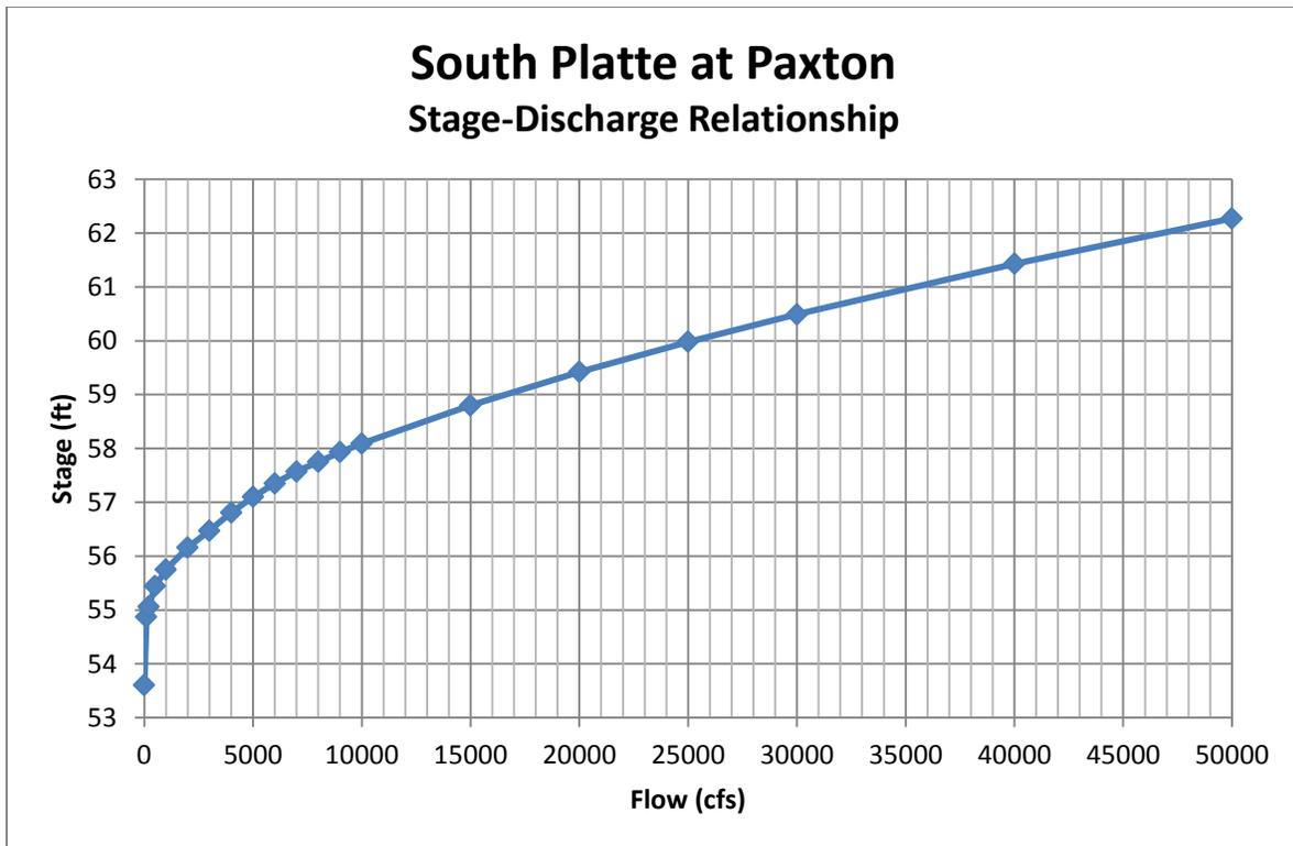
Figure 3.10 South Platte at Paxton, stage-discharge relationship
