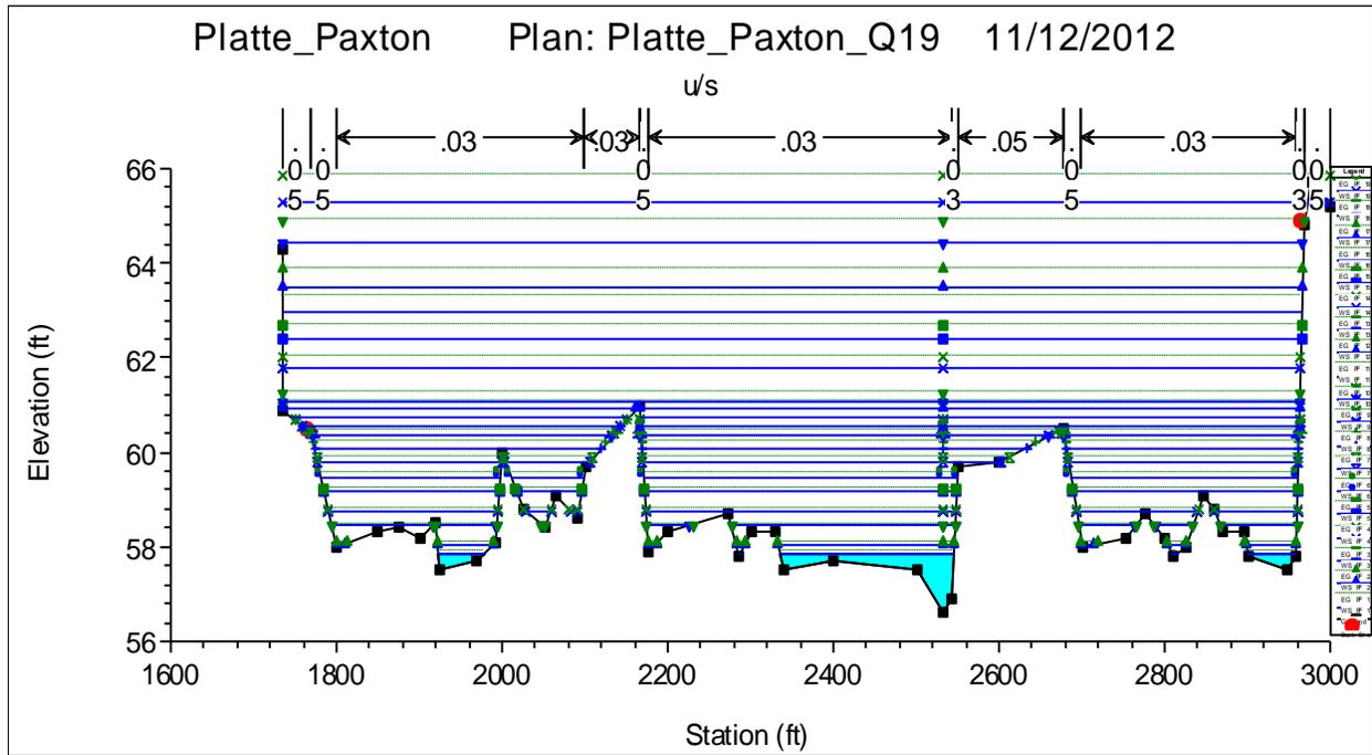
Figure 3.9 South Platte at Paxton, cross-section with water surface and EGL at flows from 100 to 50,000 cfs
