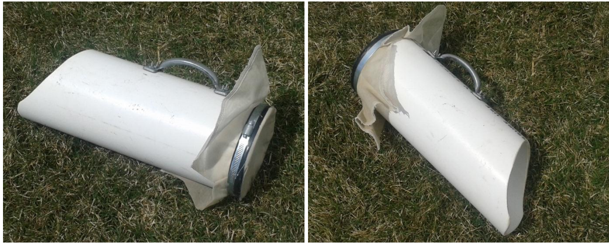
Figure 2.3. Pipe dredge used to collect bed-material samples.
