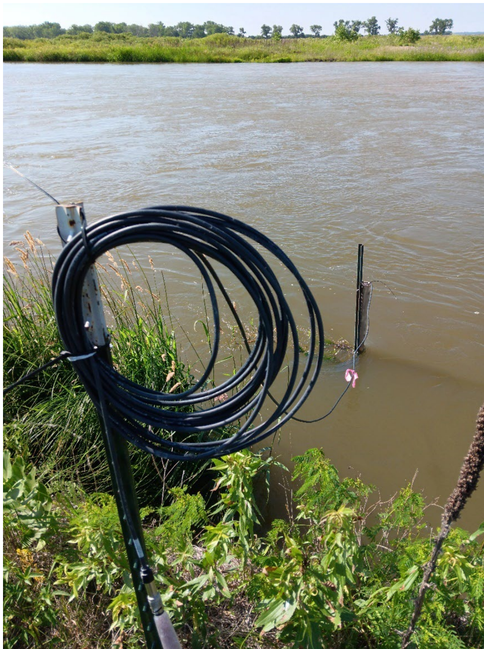
Figure 21. A stage gage assembly that was deployed in the Platte River at the Fort Kearney study area during May 2023.
